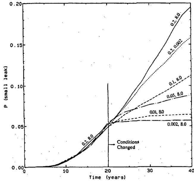
**Figure 5.7 Effect of Lowering Oxygen Concentration at Midlife (20 years) in 102-mm (4-in.) Schedule 80 304 Stainless Steel BWR Pipe. The numbers by each line are the oxygen concentration (ppm) in the coolant during plant startup and steady-state operation, respectively (Failure Analysis Associates 1990).**
