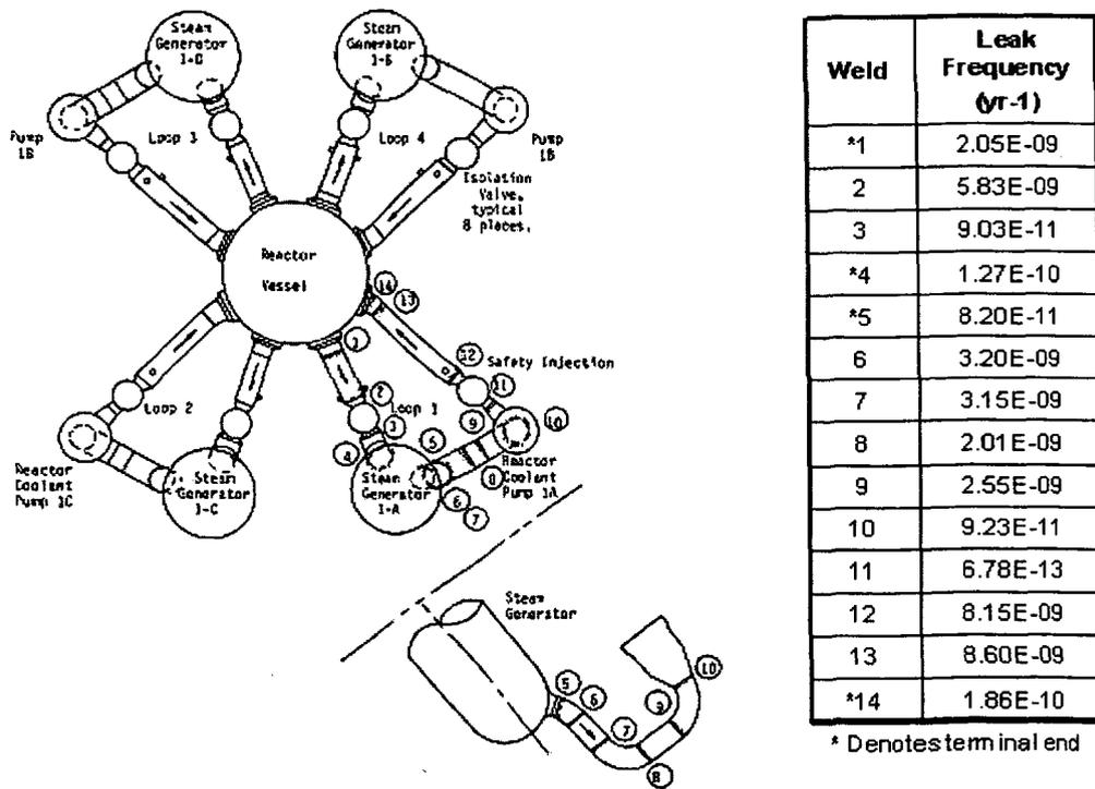
**Figure 5.13 Zion 1 Primary System Piping Weld Locations and NUREG/CR-2189 Estimated Leak Frequencies (Heasler and Simonen 1990)**
