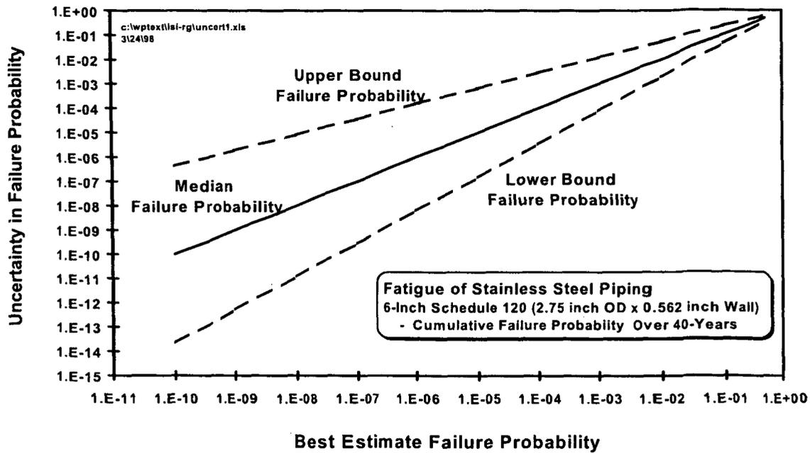
**Figure 6.3 Maximum Failure (Leak and Break) Probabilities from Sample of 100 Cases Evaluated by Uncertainty Analyses (25.4 mm = 1 in.)**
