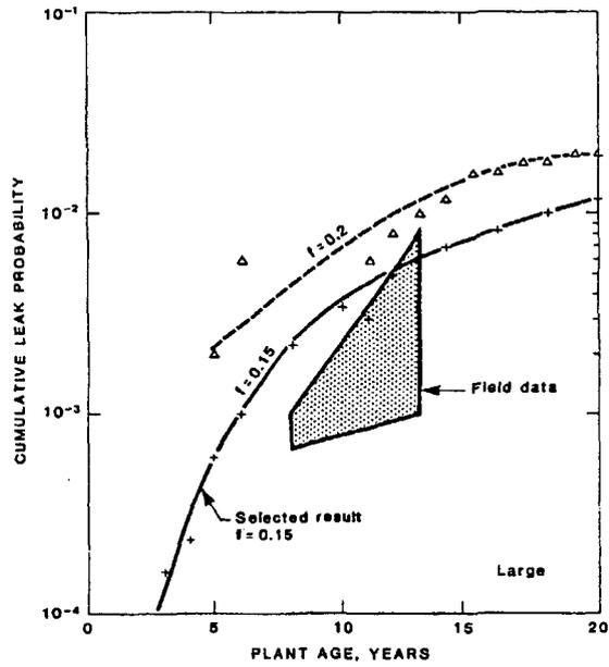
**Figure 5.1 Field Observations of Leak Probabilities and PRAISE Predictions at Various Residual Stress Adjustment Factor Values ( $f$ ) for 304 Stainless Steel Pipes Having Outside Diameters Greater Than 508 mm (>20 in.) (Harris et al. 1985)**
