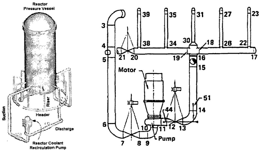
**Figure 5.3 Mark I BWR Reactor Recirculation System Piping**
