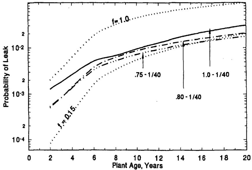
**Figure 5.2 Sample Comparison of PRAISE Cumulative Leak Probabilities (Harris et al. 1985) and Results Obtained by Khaleel et al. (1995) for Various Values of Residual Stress Adjustment Factors and Plant Loading/Unloading Frequencies**
