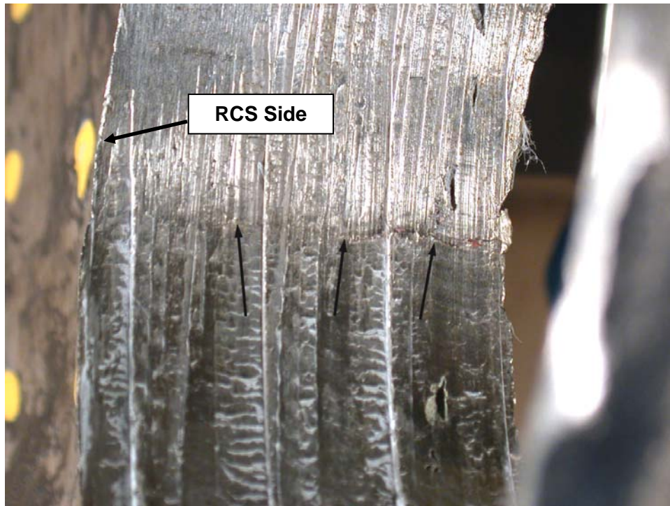
Looking at J-groove weld bore near 10°. ~1.2X
