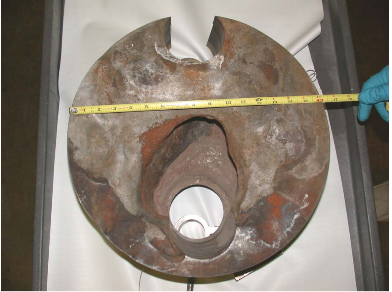
Figure 10.1 Top view of wastage cavity.
