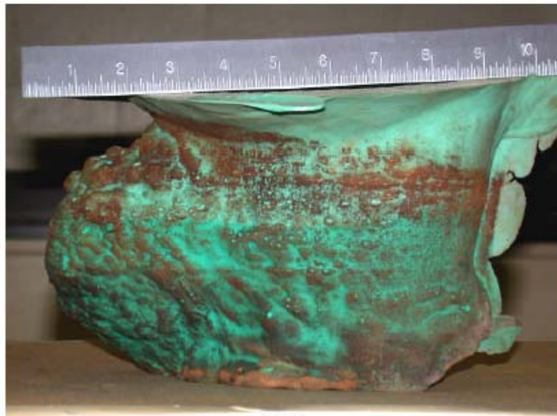
Figure 9.25(b) Dental Mold of Wastage Cavity Looking Towards 180° and 270°. 16
