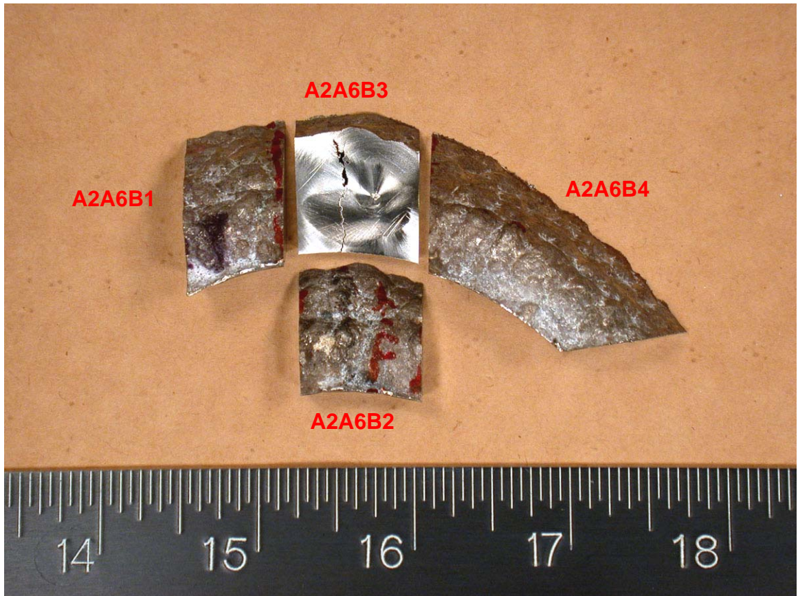
Figure 4.6 J-groove weld with the 10-degree crack showing crack and flow channel. 16
