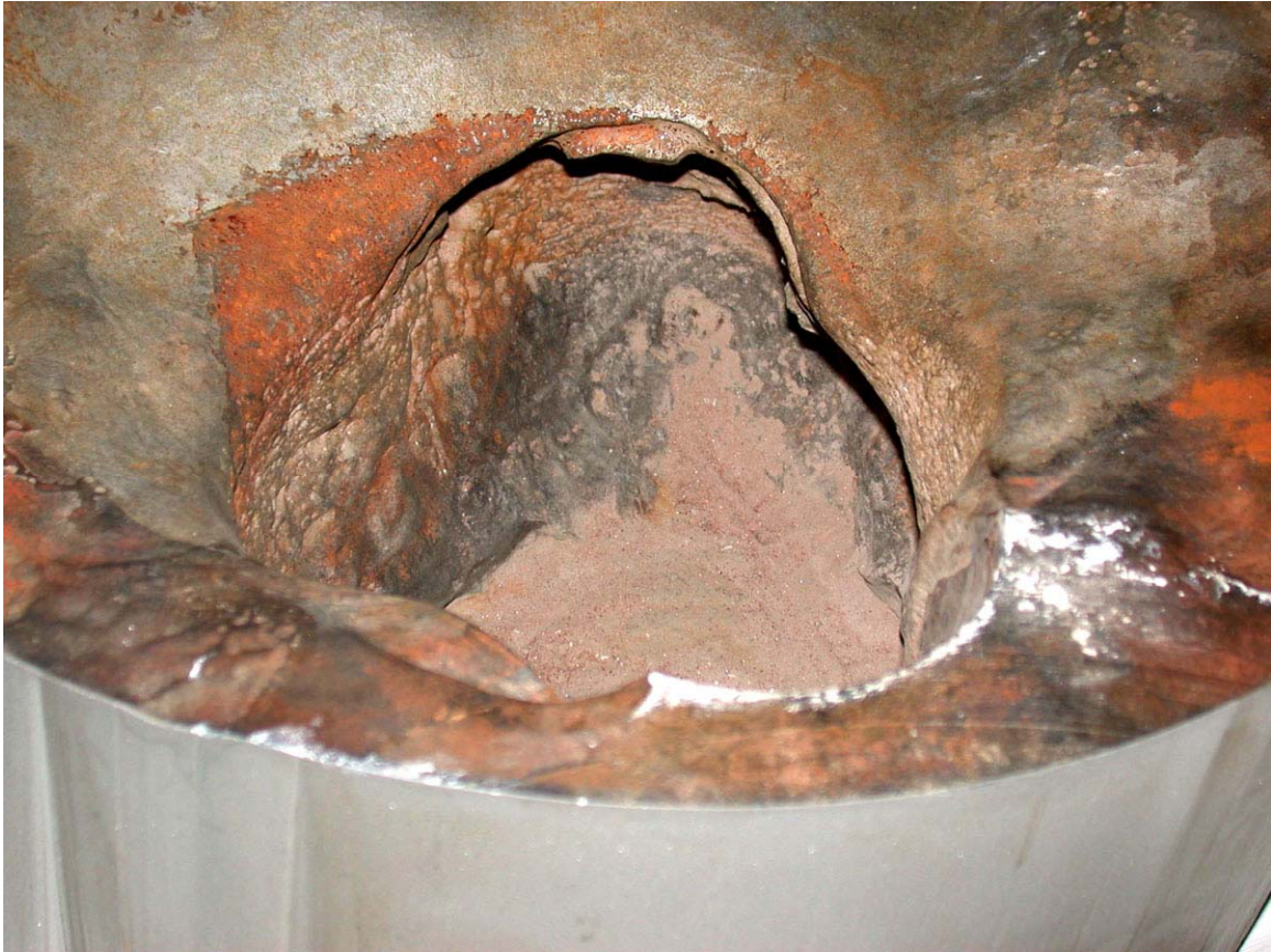
Figure 4.7 Surface morphology of the Davis-Besse RPV head wastage cavity looking toward the nose of the cavity (~10-degree). 17
