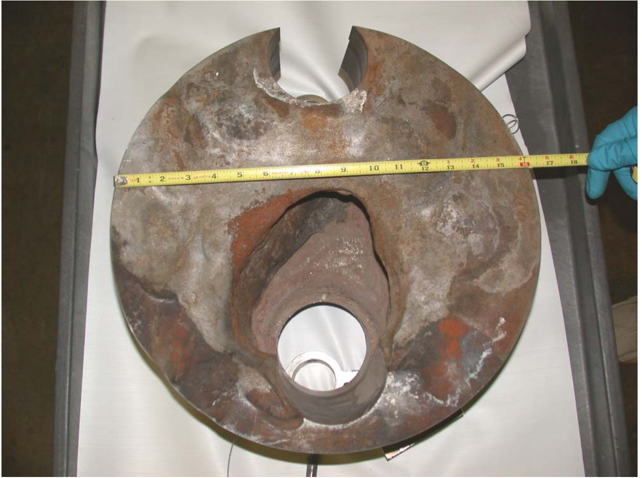
Figure 4.2 Davis-Besse RPV head wastage cavity found adjacent to Nozzle 3. 12
