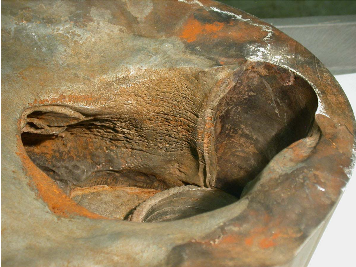
Figure 4.8 Surface morphology of the Davis-Besse RPV head wastage cavity looking toward the 90-degree side. 18
