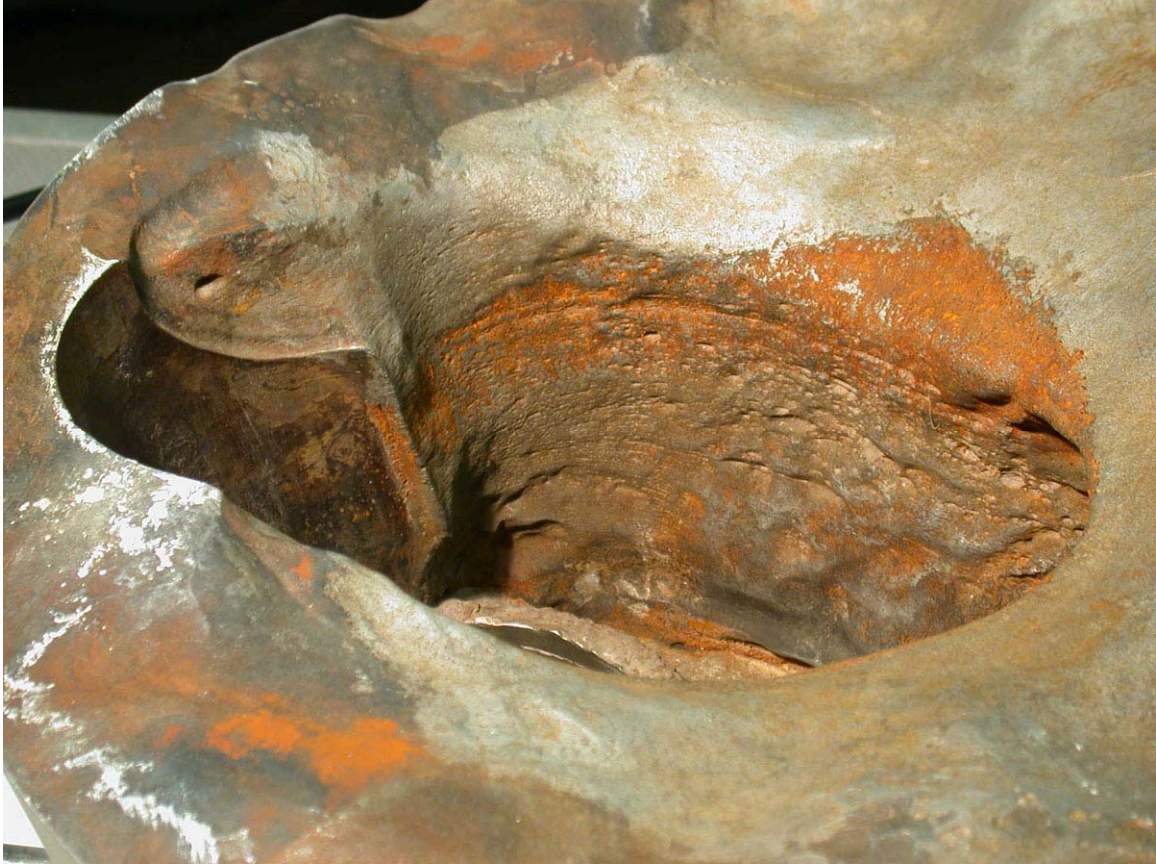
Figure 4.9 Surface morphology of the Davis-Besse RPV head wastage cavity looking toward the 270-degree side. 19
