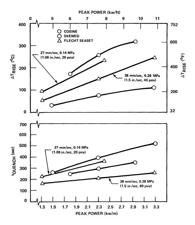
Figure 3-28. Peak Power Effect on Temperature Rise and Quench Time
