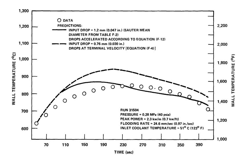
Figure 7-7. Comparisons of Predicted Wall Temperature (Rod 8H) With Data, 3.05 m (120 in.) Elevation
