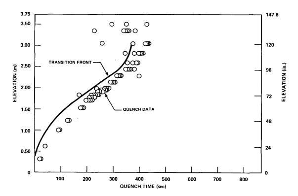
Figure 5-13. Transition Front Curve, Run 31922
