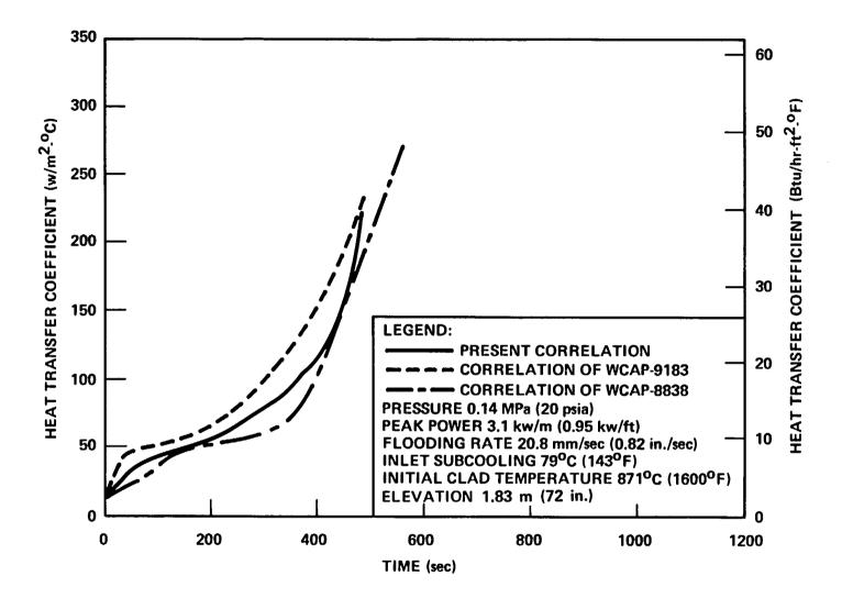
Figure 8-15. Comparison of Present Heat Transfer Coefficient Correlation With Previous Correlations, Cosine Power Run 06638
