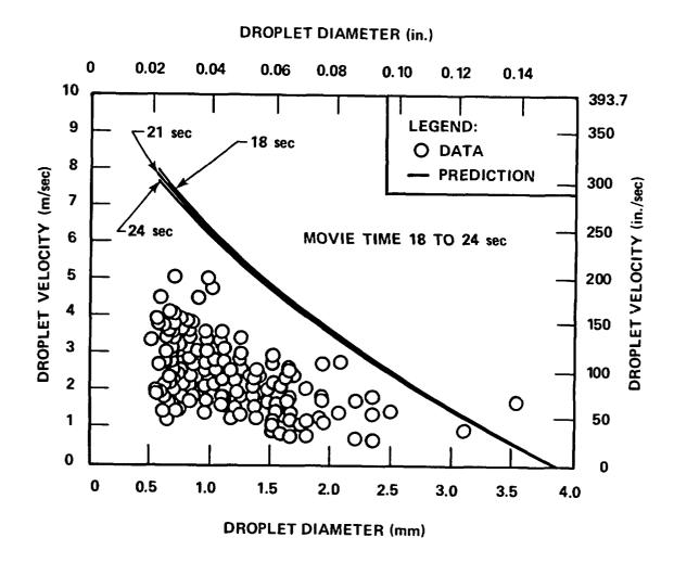
Figure F-6. Comparison of Calculated and Measured Drop Velocities, Run 32114, 0.91 m (36 in.) Elevation
