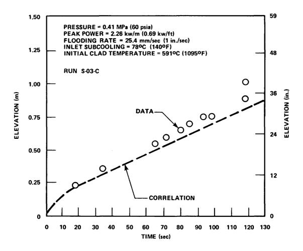
Figure 8-16. Comparison of Predicted and Measured Quench Front Elevations for a Semiscale Test
