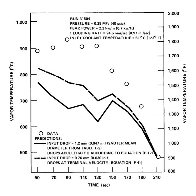
Figure 7-4. Comparisons of Predicted Vapor Temperature With Data, 1.83 m (72 in.) Elevation
