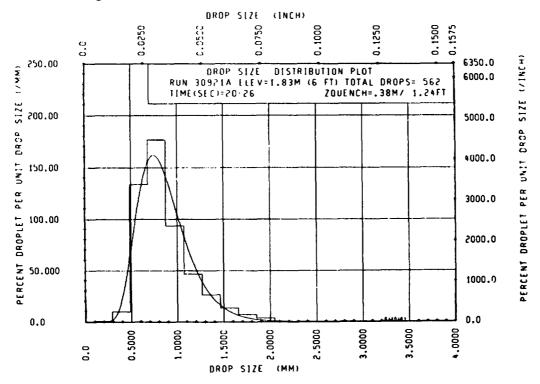
Figure E-4. Drop Size Distribution Plot, Run 3092 IA
