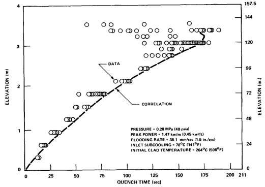
Figure G-11. Quench Correlation Versus Data, Skewed Power Run 12720
