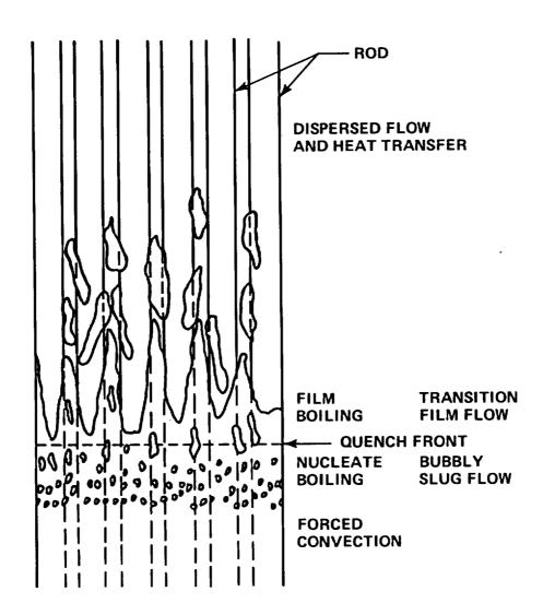
Figure 5-6. Typical Conditions in Rod Bundle During Reflood
