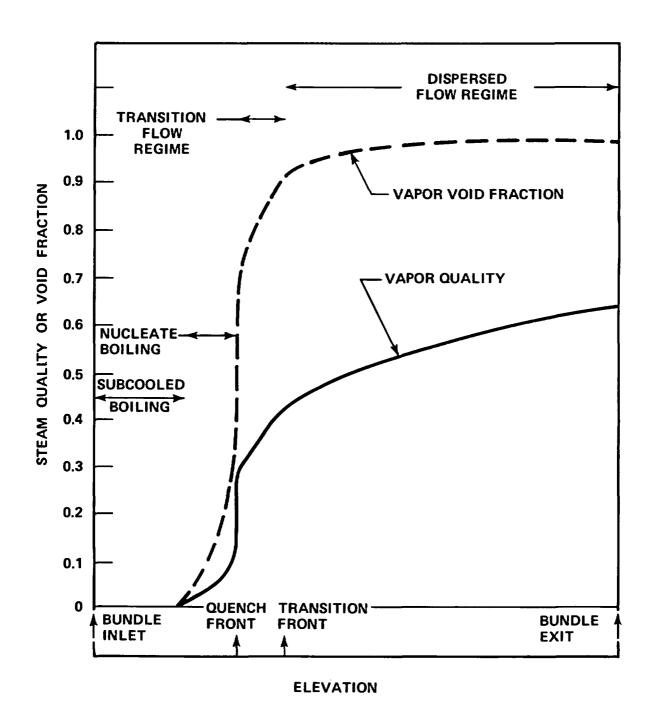
Figure 6-3. Schematic Diagram of Characteristic Vapor Quality and Void Fraction During Reflood
