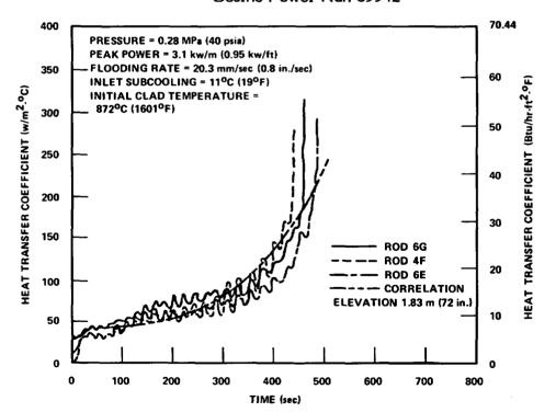
Figure H-26. Heat Transfer Coefficient Correlation Versus Data, Cosine Power Run 05342
