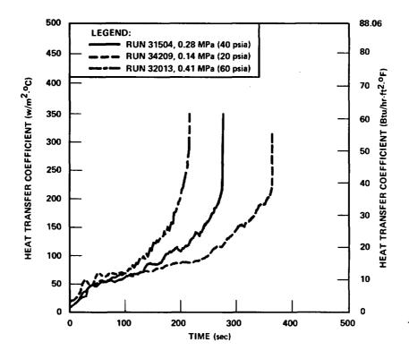
Figure 3-9. Pressure Effect on Heat Transfer
