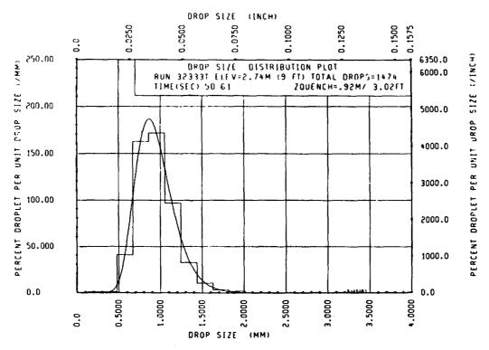
Figure E-19. Drop Size Distribution Plot, Run 32333 (Total), 2.74 m (108 in.) Elevation
