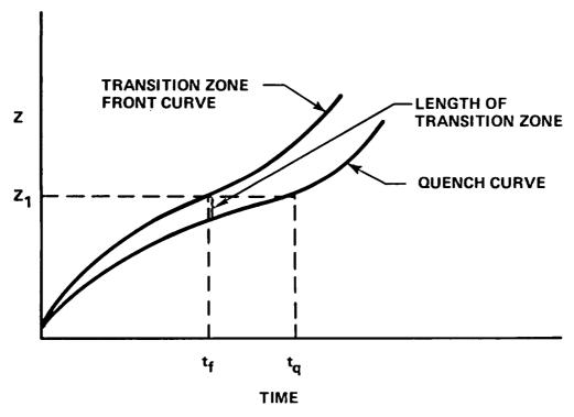
Figure 5-8. Schematic Construction of Transition Zone Curve
