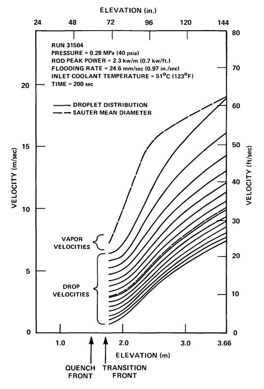
Figure 6-11. Calculated Drop and Vapor Velocities in Dispersed Flow Regime
