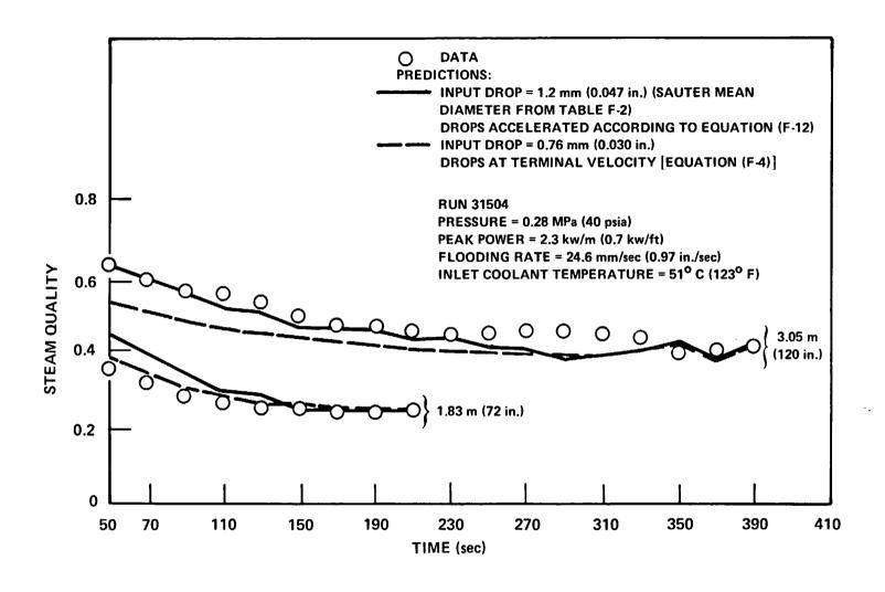
Figure 7-3. Comparisons of Predicted Steam Quality With Data-Based Steam Quality
