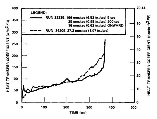
Figure 3-31. Initial Flooding Rate Effect on Heat Transfer Run 32235
