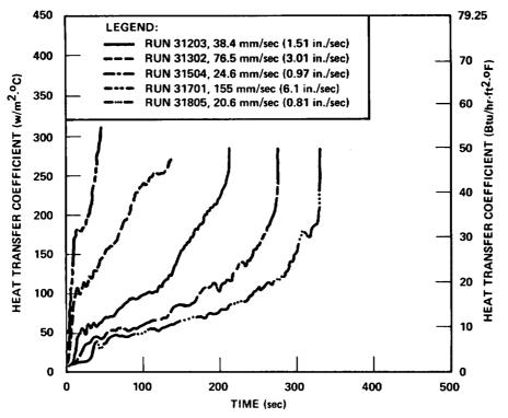
Figure 3-1. Flooding Rate Effect on Heat Transfer [1.83 m (72 in.) Elevation)]
