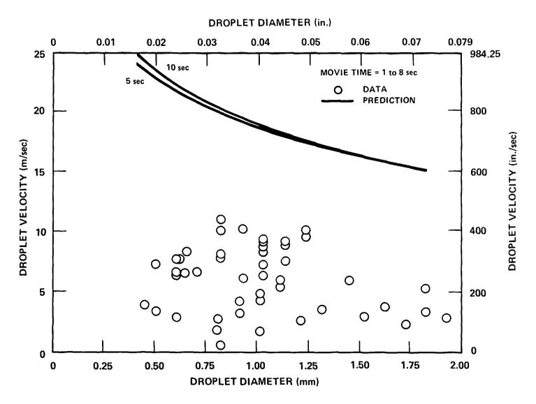
Figure F-5. Comparison of Calculated and Measured Drop Velocities, Run 31701, 2.74 m (108 in.) Elevation
