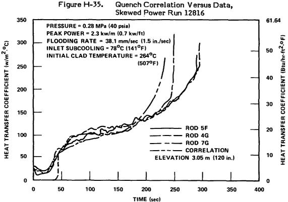
Heat Transfer Coefficient Correlation Versus Data, Skewed Power Run 12816
