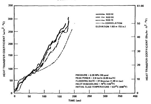
Figure G-4. Heat Transfer Coefficient Correlation Versus Data, Cosine Power Run 00904
