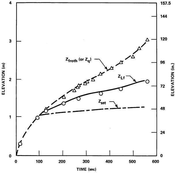
Figure 5-1. FLECHT SEASET Froth Level, Collapsed Liquid Level, and Saturation Level Data
