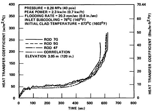
Figure H-30. Heat Transfer Coefficient Correlation Versus Data, Skewed Power Run 15305
