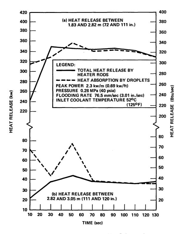
Figure 6-2. Comparisons of Bunole Heat Release and Heat Absorption by Droplets, Run 31302
