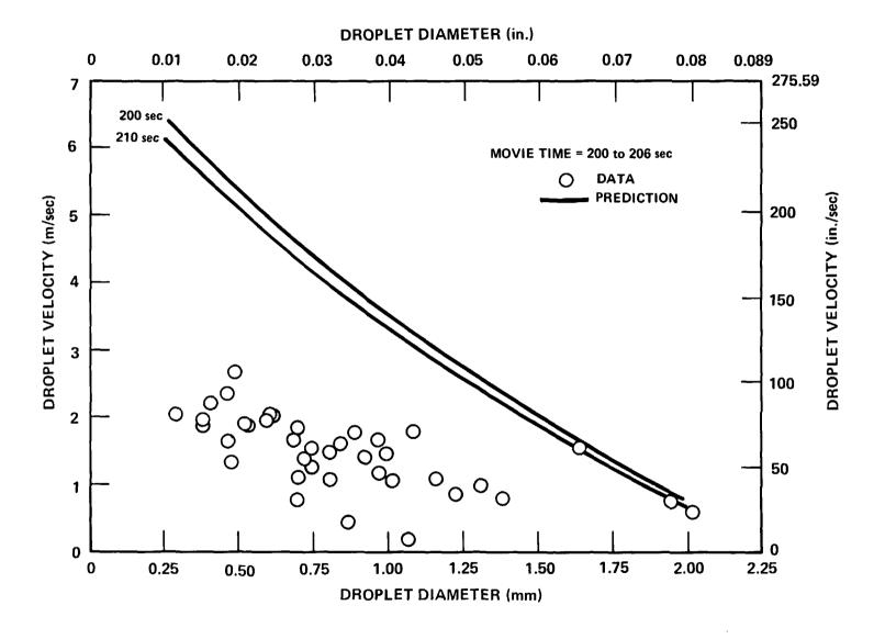
Figure F-3. Comparison of Calculated and Measured Drop Velocities, Run 31504, 1.83 m (72 in.) Elevation
