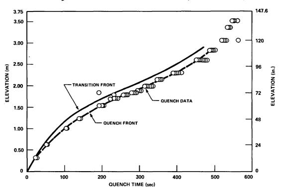
Figure 5-16. Transition Front Curve, Run 34006
