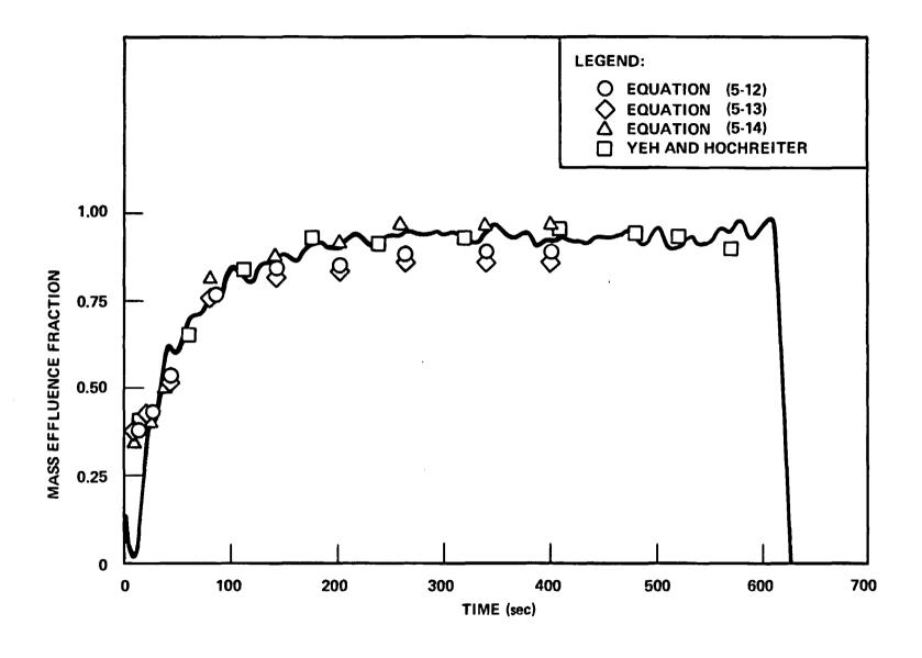
Figure 5-5. Mass Effluence Fraction Compared With Model Predictions, Run 31504
