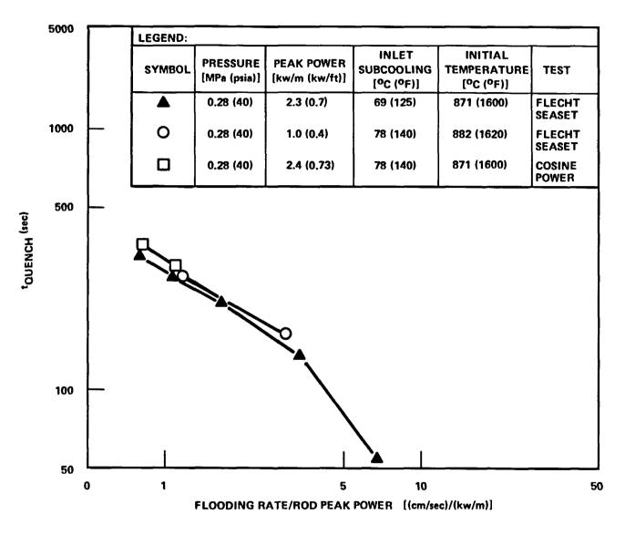
Figure 3-8.  $t_{Quench}$  Vs. Flood Rate/Rod Peak Power
