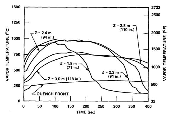
Figure 4-4. Vapor Temperature at Various Elevations, Run 31504
