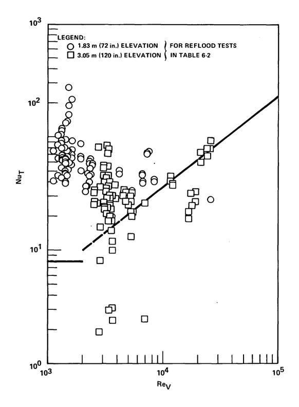
Figure 6-13. Calculated Nusselt Number (Based on Heater Rod Total Heat Flux) Versus Vapor Reynolds Number
