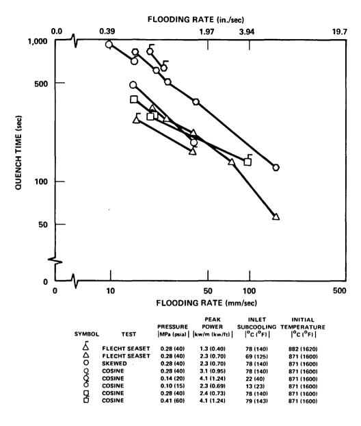
Figure 3-6. Quench Time Versus Flooding Rate
