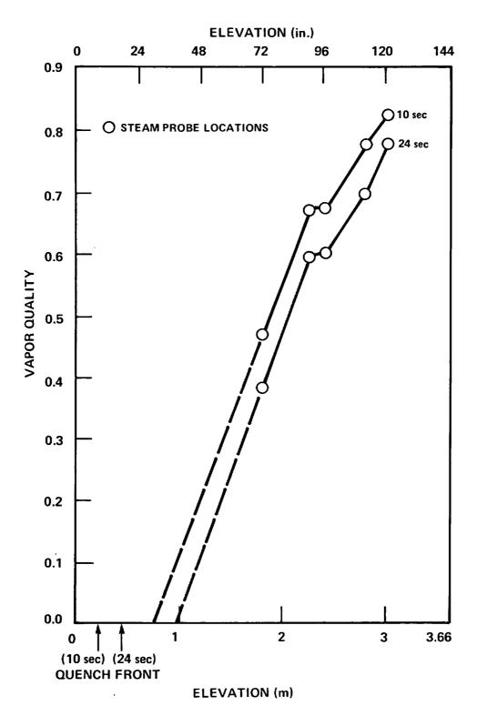
Figure F-1. Data-Based Steam Quality for Run 34524 Shortly After Flooding
