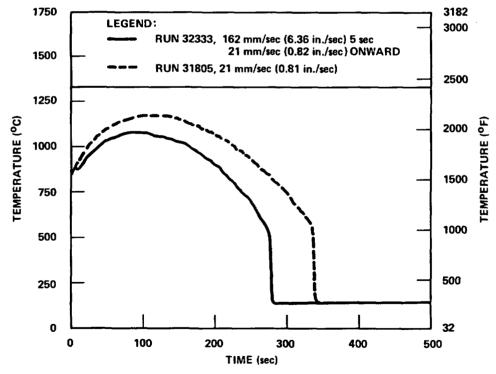
Figure 3-30. Initial Flooding Rate Effect on Temperature, Run 32333
