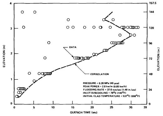
Figure G-3. Quench Correlation Versus Data, Cosine Power Run 00904
