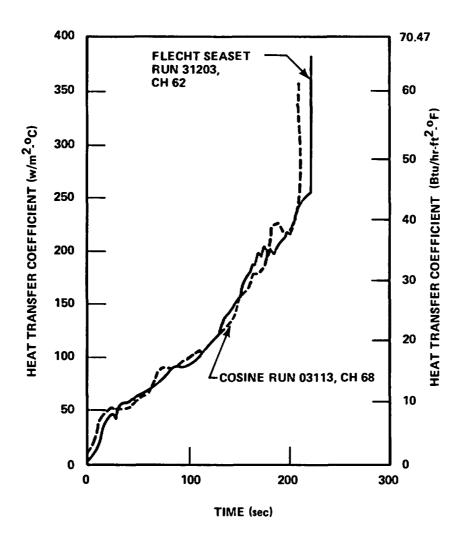
Figure 3-49. Overlap Test Heat Transfer Coefficient Comparison, FLECHT SEASET Run 31203 and Cosine Run 03113
