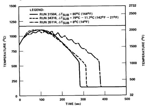
Figure 3-40. Subcooling Transient Effect on Temperature
