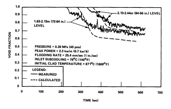
Figure 5-2. Comparison of Calculated and Measured Void Fraction, Run 31504 (sheet 2 of 2)
