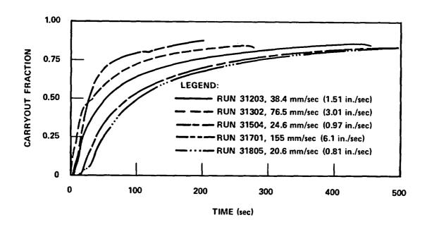
Figure 3-3. Flooding Rate Effect on Carryout Fraction
