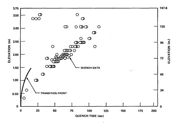
Figure 5-15. Transition Front Curve, Run 31701
