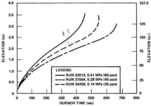
Figure 3-12. Pressure Effect on Quench Front Advance
