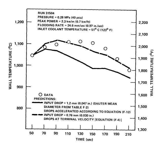
Figure 7-6. Comparisons of Predicted Wall Temperature (Rod 8H) With Data, 1.83 m (72 in.) Elevation
