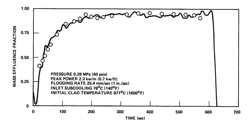
Figure 5-3. Comparison of Calculated and Measured Mass Storage Rate, Run 31504
