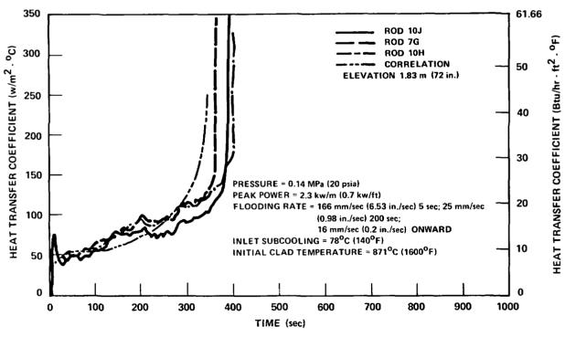
Figure H-16. Heat Transfer Coefficient Correlation Versus Data, FLECHT SEASET Run 32235
