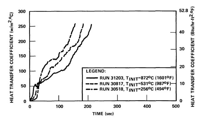
Figure 3-19. Initial Clad Temperature Effect on Heat Transfer
