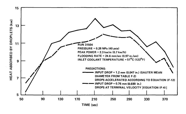
Figure 7-2. Predicted Droplet Heat Absorption Rate Between 2.90 and 3.05 m (114 and 120 in.) Elevations
