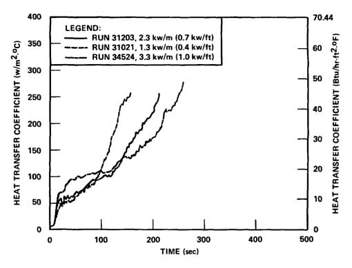
Figure 3-24. Peak Power Effect on Heat Transfer
