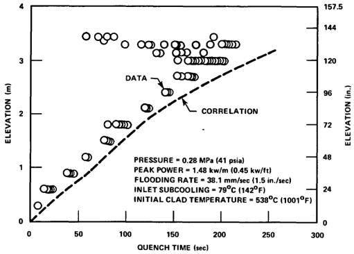
Figure G-5. Quench Correlation Versus Data, Skewed Power Run 11719
