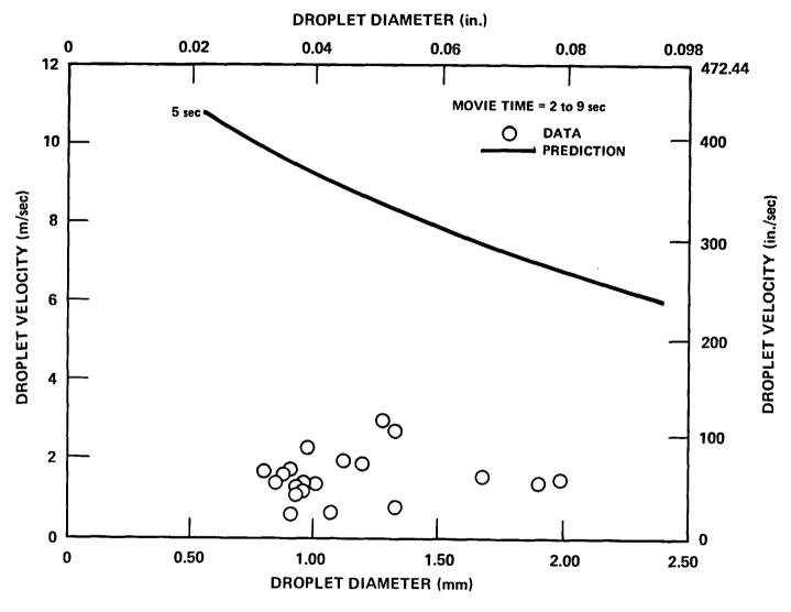
Figure F-4. Comparison of Calculated and Measured Drop Velocities, Run 31701, 0.91 m (36 in.) Elevation
