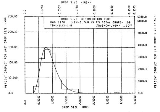
Figure E-10. Drop Size Distribution Plot, Run 31701, 2.74 m (108 in.) Elevation
