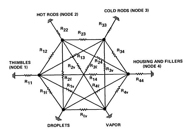
Figure 6-5. Radiation Network for Calculating Radiation Heat Transfer in FLECHT SEASET 161-Rod Bundle
