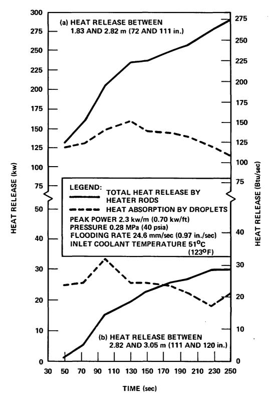
Figure 6-1. Comparisons of Bundle Heat Release and Heat Absorption by Droplets, Run 31504
