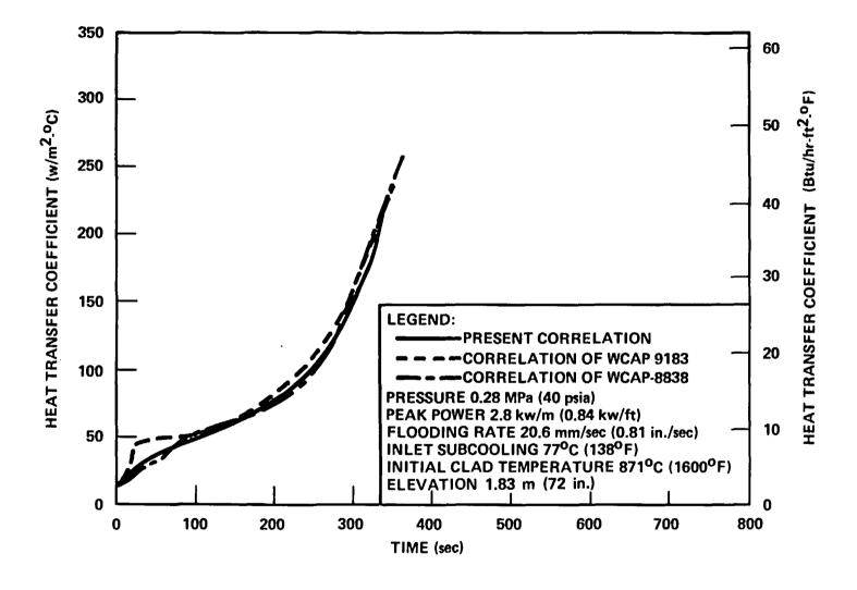
Figure 8-13. Comparison of Present Heat Transfer Coefficient Correlation With Previous Correlations, Cosine Power Run 02414
