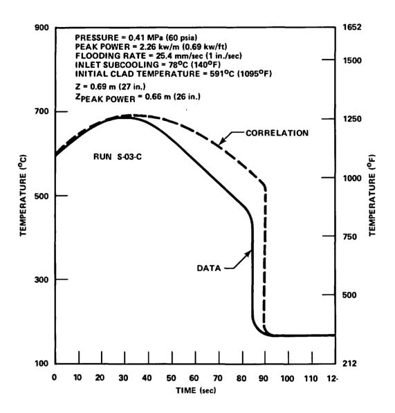
Figure 8-17. Comparison of Predicted and Measured Clad Surface Temperatures for a Semiscale Test
