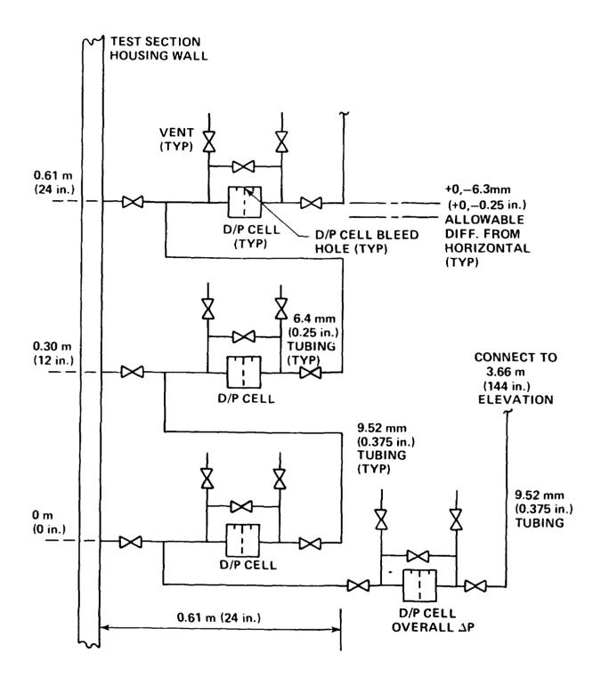
Figure 2-3. FLECHT SEASET Unblocked Bundle Test Section Housing Differential Pressure Cell Hookup
