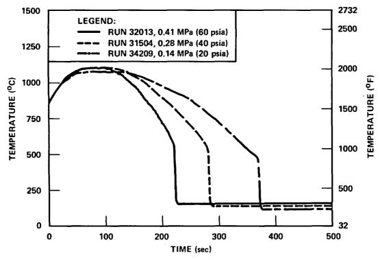
Figure 3-10. Pressure Effect on Temperature
