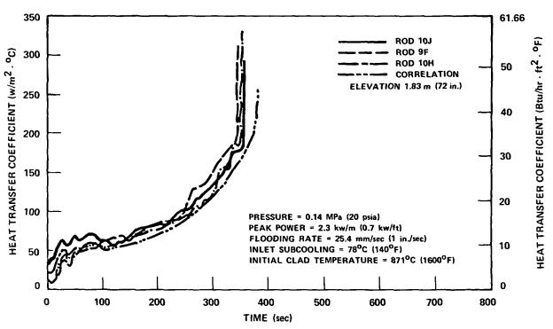
Figure H-8. Heat Transfer Coefficient Correlation Versus Data, FLECHT SEASET Run 34209
