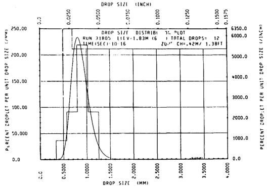
Figure E-12. Drop Size Distribution Plot, Run 31805, 1.83 m (72 in.) Elevation
