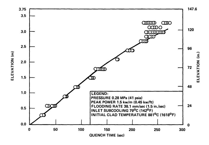
Figure 8-3. Quench Correlation Versus Data, FLECHT Skewed Profile Run 11618
