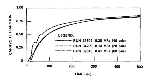
Figure 3-11. Pressure Effect on Carryout Fraction
