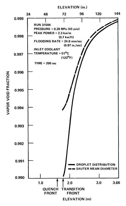
Figure 6-7. Calculated Vapor Void Fraction in Dispersed Flow Regime
