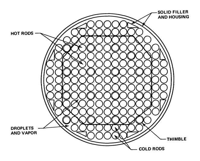
Figure 6-4. Six Radiation Nodes for Calculating Radiation Heat Transfer in FLECHT SEASET 161-Rod Bundle
