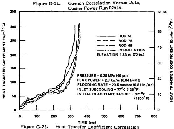
Heat Transfer Coefficient Correlation Versus Data, Cosine Power Run 02414
