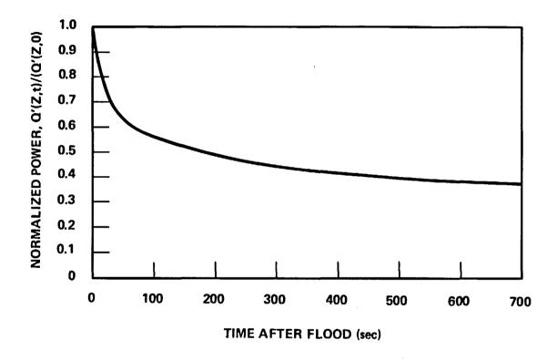
Figure I-1. FLECHT Power Decay Curve B Normalized With Initial Power
