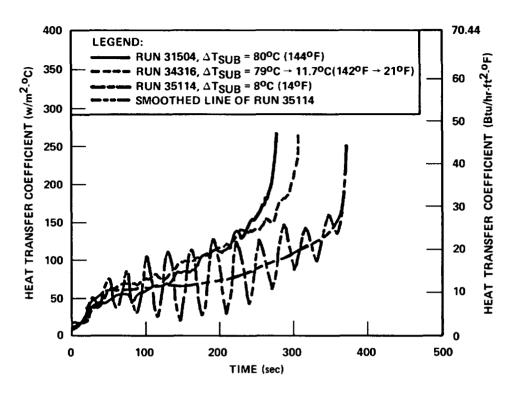
Figure 3-39. Subcooling Transient Effect on Heat Transfer
