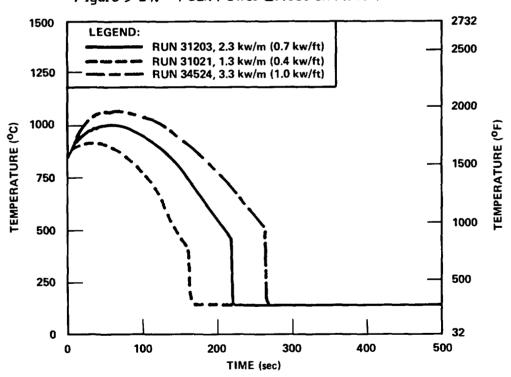
Figure 3-25. Peak Power Effect on Temperature
