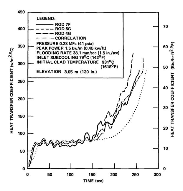
Figure 8-12. Comparison of Heat Transfer Coefficient Correlation With Data From Skewed Power Run 11618
