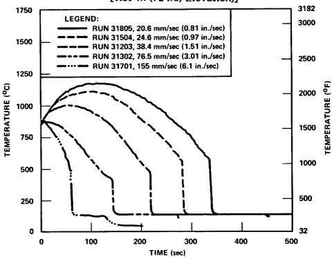
Figure 3-2. Flooding Rate Effect on Temperature
