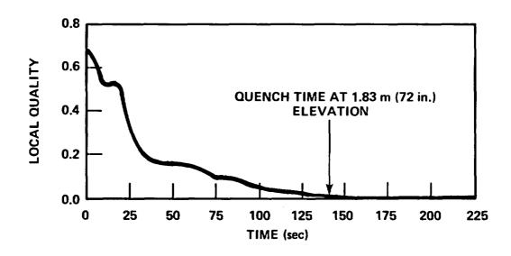
Figure B-8. Quality Transient, 1.83 m (72 in.) Elevation, Run 31302
