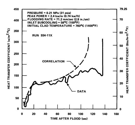
Figure 8-18. Comparison of Predicted and Measured Heat Transfer Coefficients for a BWR FLECHT Test
