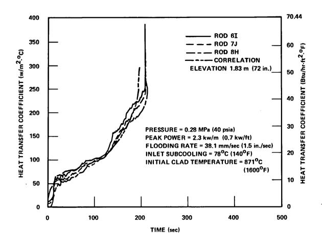
Figure 8-10. Comparison of Heat Transfer Coefficient Correlation With Data From FLECHT SEASET Run 31203
