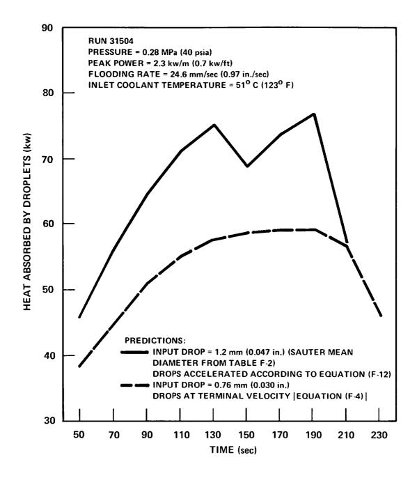
Figure 7-1. Predicted Droplet Heat Absorption Rate Between 1.83 and 2.29 m (72 and 90 in.) Elevations
