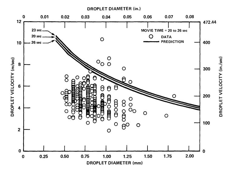
Figure F-2. Comparison of Calculated and Measured Drop Velocities, Run 30921, 1.83 m (72 in.) Elevation
