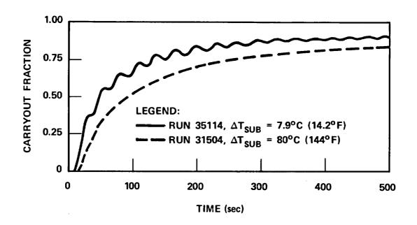
Figure 3-16. Subcooling Effect on Carryout Fraction
