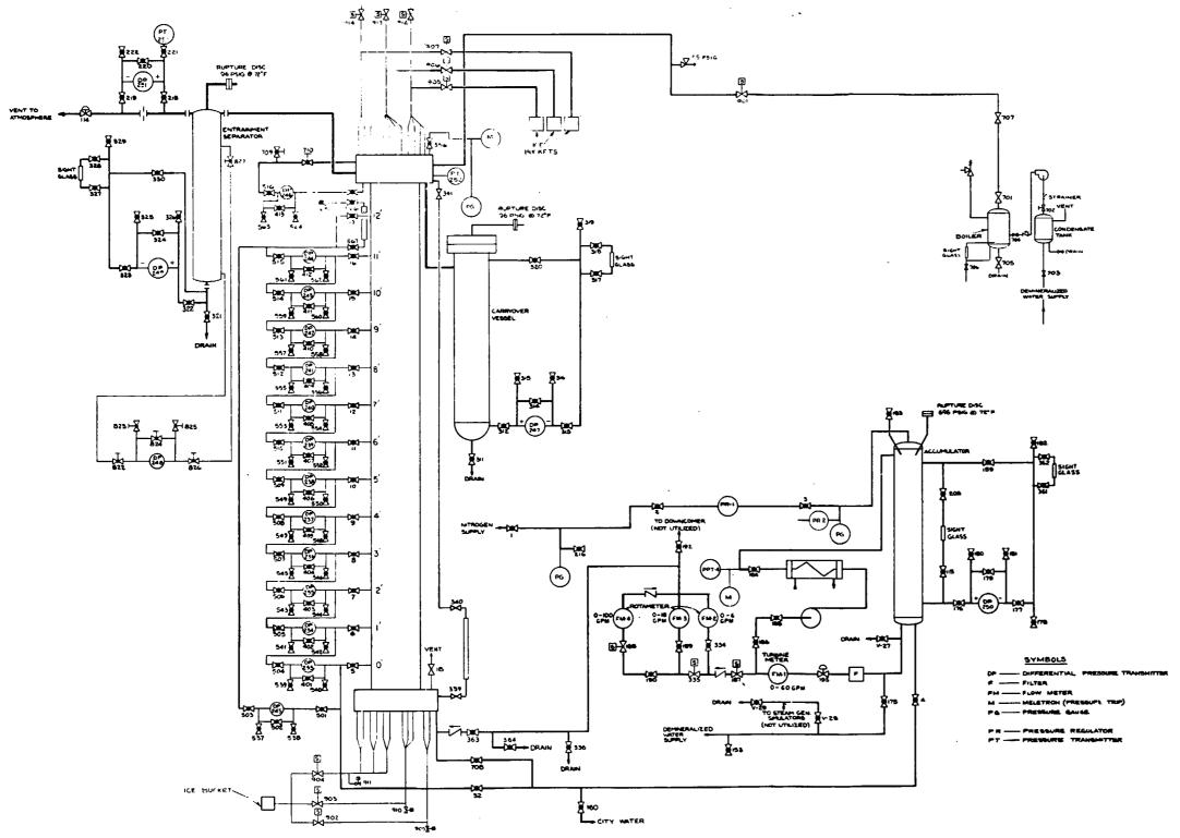
Figure 2-1. Flow Diagram for Forced Reflood Configuration (FLECHT SEASET Unblocked Bundle)
