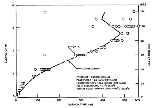
Figure H-17. Quench Correlation Versus Data, Cosine Power Run 02603
