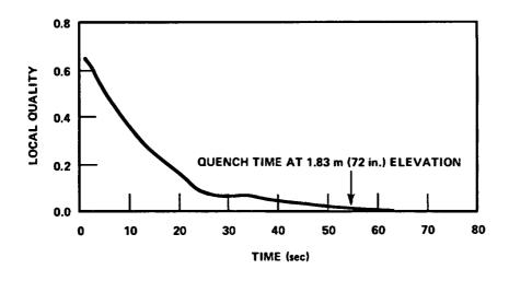
Figure B-12. Quality Transient, 1.83 m (72 in.) Elevation, Run 31701
