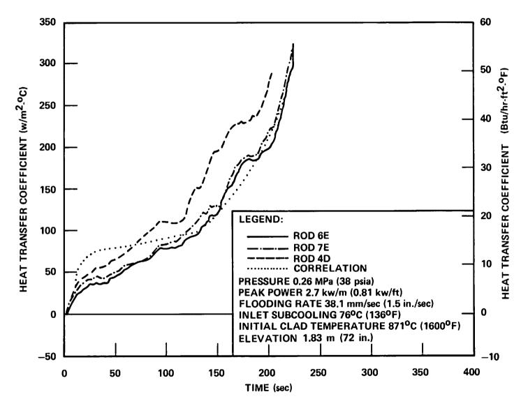
Figure 8-11. Comparison of Heat Transfer Coefficient Correlation With Data From Cosine Power Run 03113
