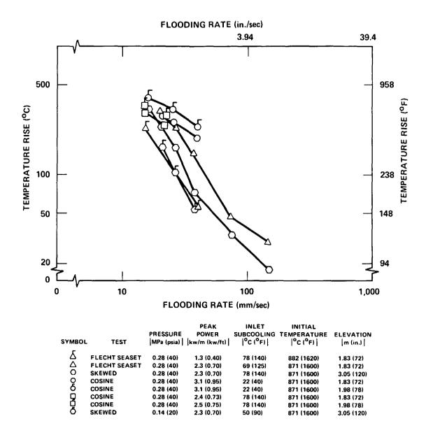
Figure 3-5. Temperature Rise Comparisons at Various Flooding Rates
