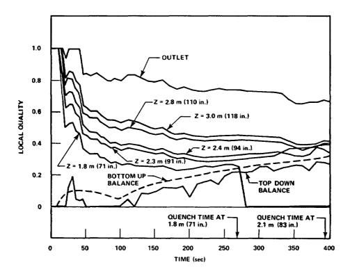
Figure 4-2. Local Quality at Various Elevations, Run 31504
