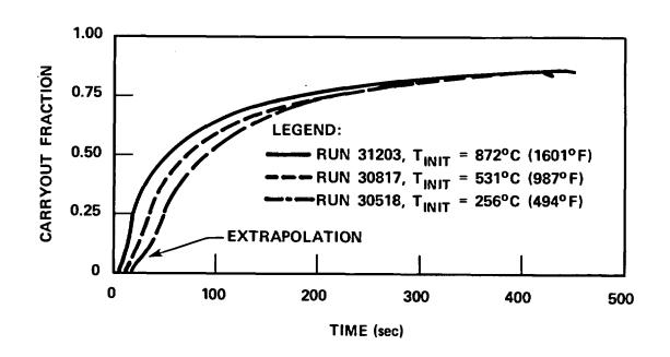
Figure 3-21. Initial Clad Temperature Effect on Carryout Fraction
