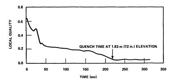
Figure B-4. Quality Transient, 1.83 m (72 in.) Elevation, Run 31203
