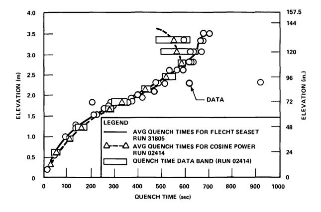
Figure 3-48. Overlap Test Quench Curve Comparison, FLECHT SEASET Run 31805 and Cosine Run 02414
