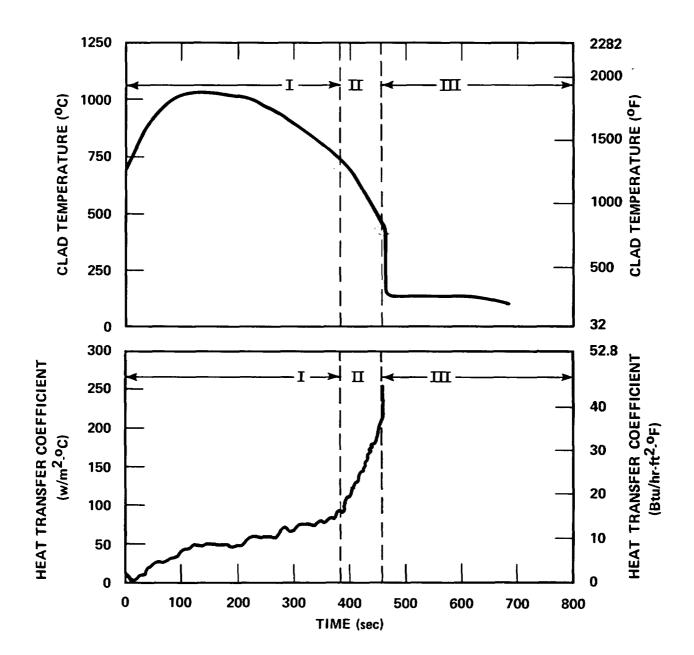
Figure 5-7. Temperature and Heat Transfer Coefficient Curve, Showing Transition Zone (II)
