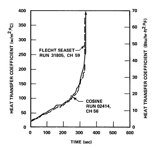
Figure 3-52. Overlap Test Heat Transfer Coefficient Comparison, FLECHT SEASET Run 31085 and Cosine Run 02414
