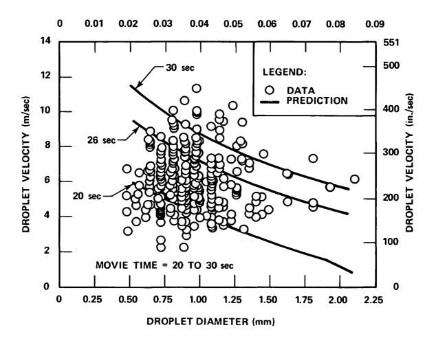
Figure F-7. Comparison of Calculated and Measured Drop Velocities, Run 32114, 2.74 m (108 in.) Elevation
