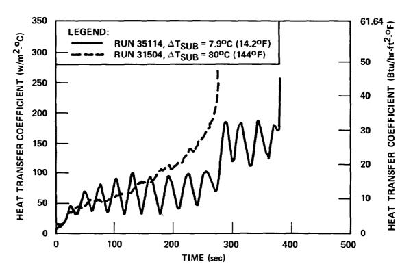
Figure 3-14. Subcooling Effect on Heat Transfer
