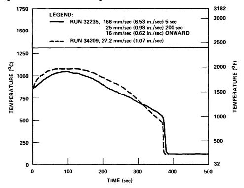
Figure 3-32. Initial Flooding Rate Effect on Temperature, Run 32235
