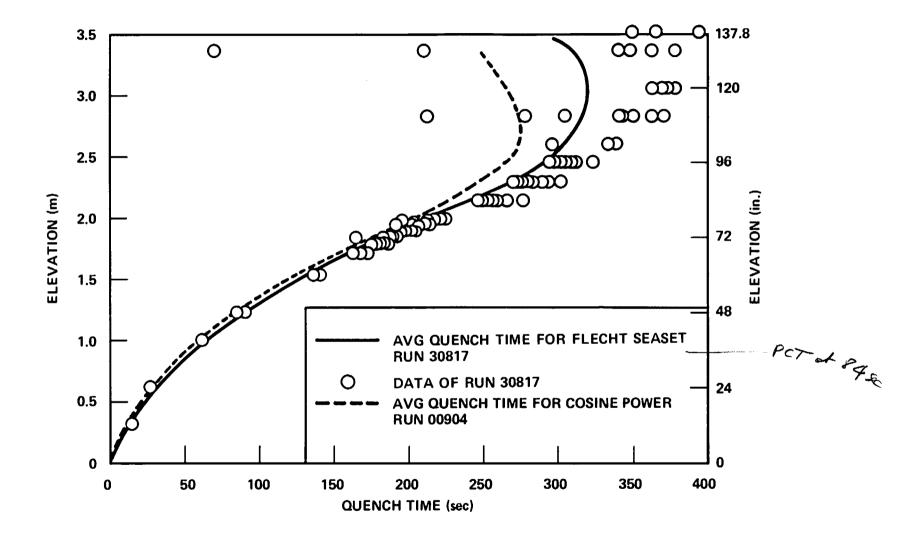
Figure 3-46. Overlap Test Quench Curve Comparison, FLECHT SEASET Run 30817 and Cosine Run 00904
