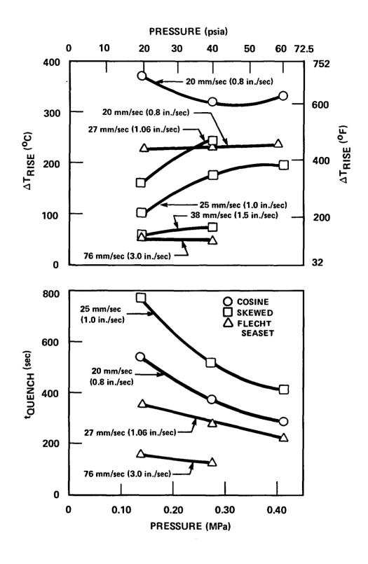
Figure 3-13. Pressure Effect on Temperature Rise and Quench Time
