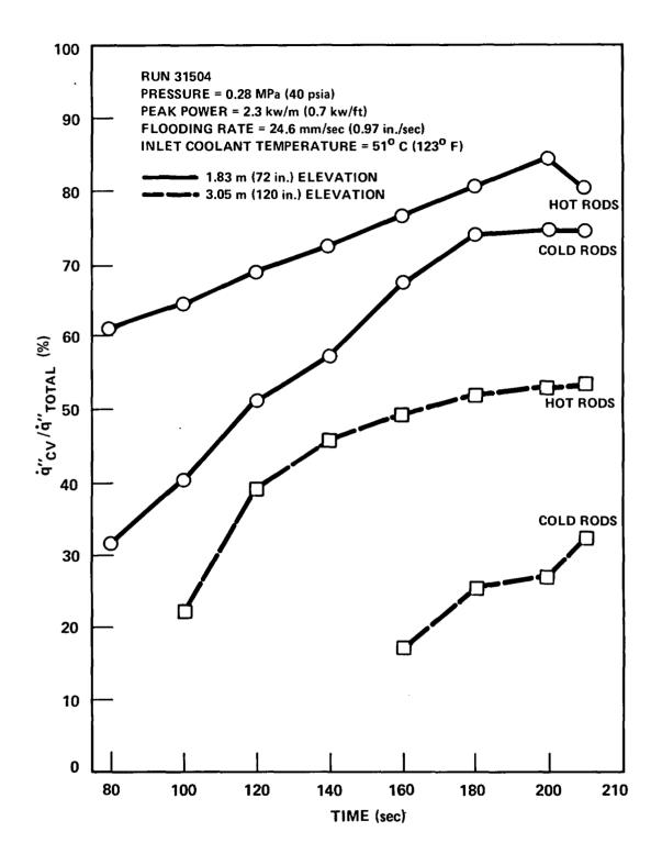
Figure 6-12. Relative Contribution of Convective Heat Flux During Reflood at 1.83 m (72 in.) and 3.05 m (120 in.) Elevations
