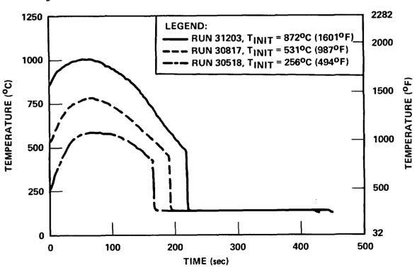
Figure 3-20. Initial Clad Temperature Effect on Temperature
