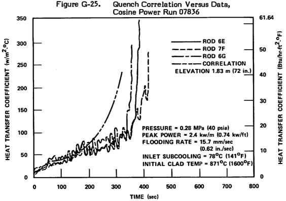
Figure G-26. Heat Transfer Coefficient Correlation Versus Data, Cosine Power Run 07836
