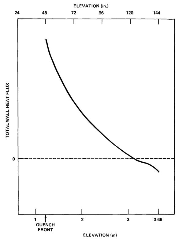
Figure 6-15. Typical Wall Heat Flux Axial Distribution for a Cosine-Shaped Power Profile Heater Rod During Reflood
