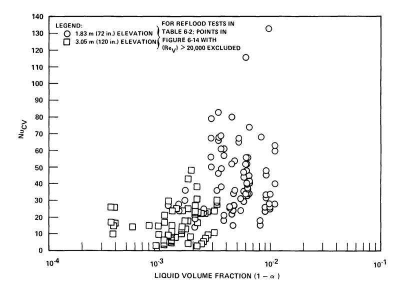
Figure 6-16. Calculated Nusselt Number (Based on Heater Rod Convective Heat Flux) Versus Liquid Volume Fraction
