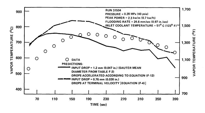
Figure 7-5. Comparisons of Predicted Vapor Temperature With Data, 3.05 m (120 in.) Elevation
