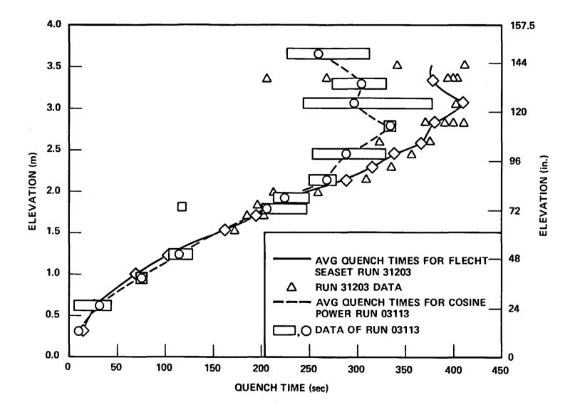
Figure 3-45. Overlap Test Quench Curve Comparison, FLECHT SEASET Run 31203 and Cosine Run 03113
