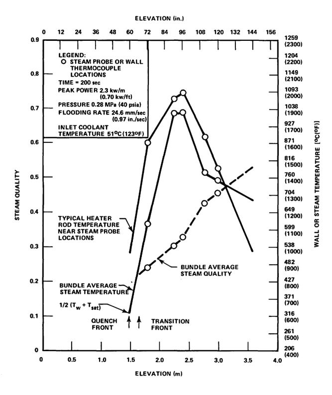
Figure 6-6. Data-Based Wall Temperature, Steam Temperature, and Steam Quality
