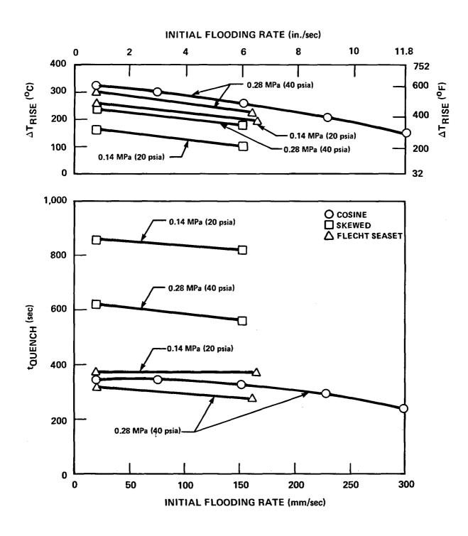
Figure 3-37. Initial Flooding Rate Effect on Temperature Rise and Quench Time
