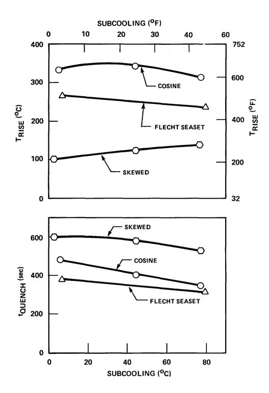
Figure 3-18. Subcooling Effect on Temperature Rise and Quench Time
