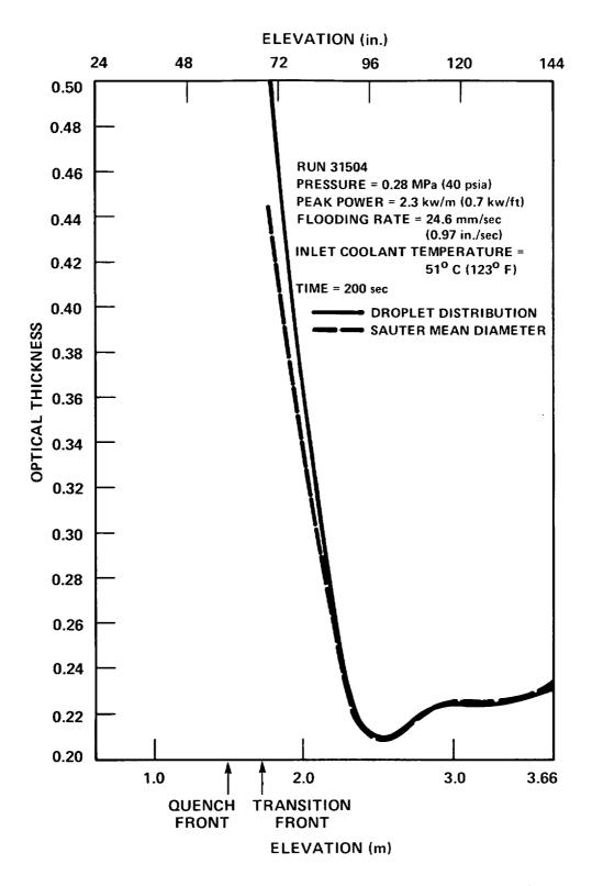
Figure 6-9. Calculated Optical Thickness in Dispersed Flow Regime
