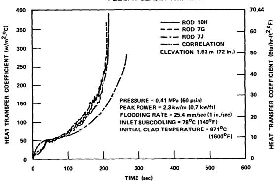
Figure H-10. Heat Transfer Coefficient Correlation Versus Data, FLECHT SEASET Run 32013
