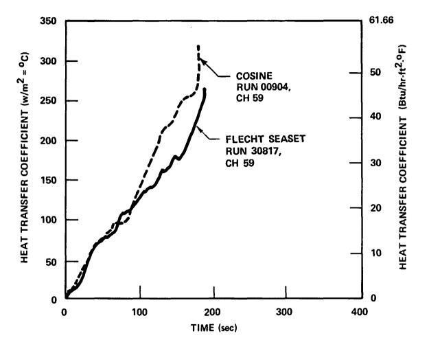
Figure 3-50. Overlap Test Heat Transfer Coefficient Comparison, FLECHT SEASET Run 30817 and Cosine Run 00904
