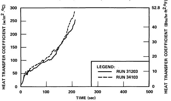
Figure 3-43. Average Heat Transfer Coefficient Comparison for Repeat Tests
