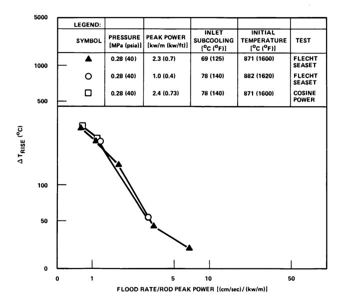
Figure 3-7. Temperature Rise Versus Flooding Rate and Rod Peak Power
