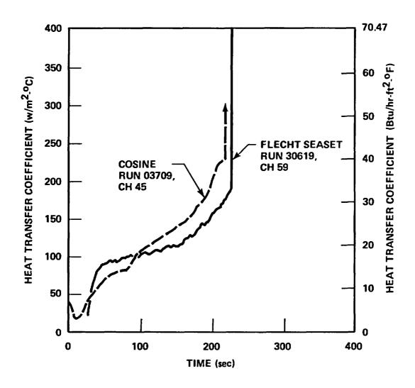
Figure 3-51. Overlap Test Heat Transfer Coefficient Comparison, FLECHT SEASET Run 30619 and Cosine Run 03709
