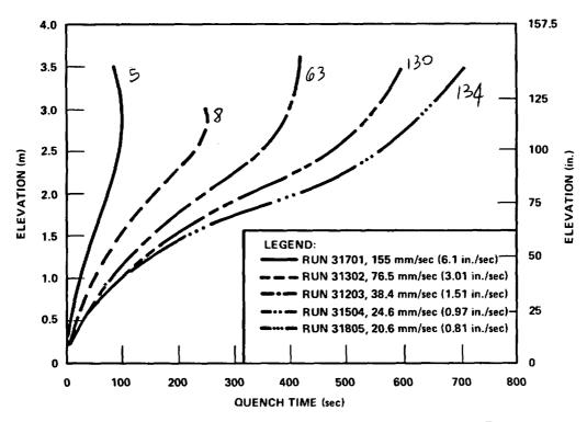
Figure 3-4. Quench Front Advances at Various Flooding Rates
