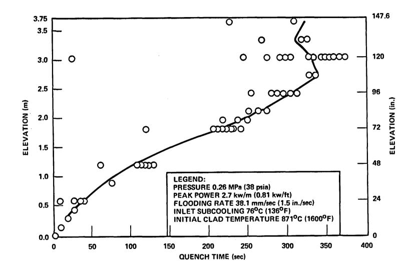
Figure 8-2. Quench Correlation Versus Data, FLECHT Cosine Run 03113
