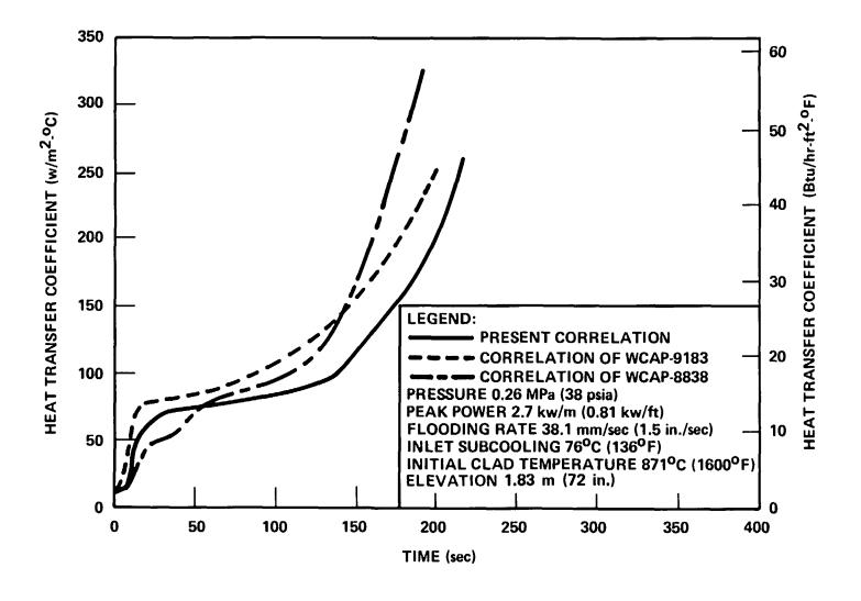
Figure 8-14. Comparison of Present Heat Transfer Coefficient Correlation With Previous Correlations, Cosine Power Run 03113
