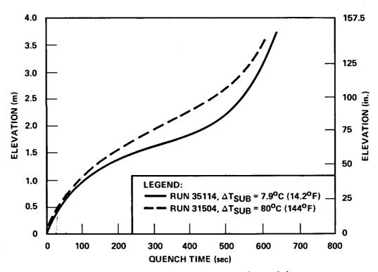
Figure 3-17. Subcooling Effect on Quench Front Advance
