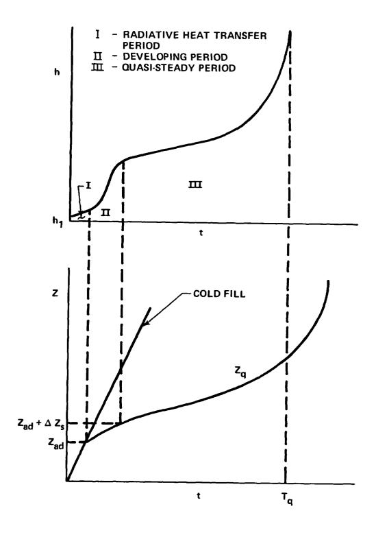
Figure 8-7. Adiabatic, Developing, and Quasi-Steady Periods in Heat Transfer Coefficient Correlation
