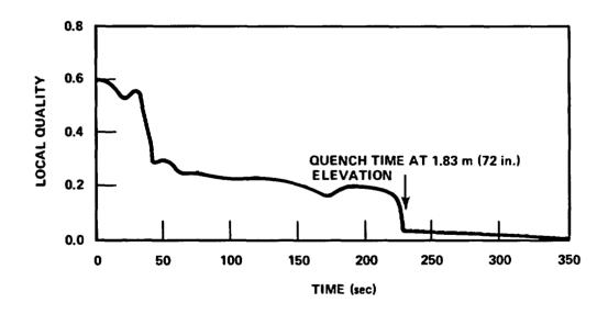
Figure B-20. Quality Transient, 1.83 m (72 in.) Elevation, Run 31922
