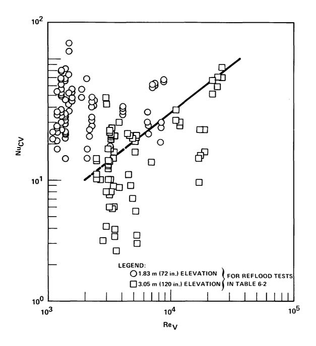
Figure 6-14. Calculated Nusselt Number (Based on Heater Rod Convective Heat Flux) Versus Vapor Reynolds Number
