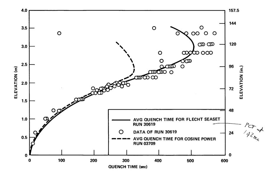
Figure 3-47. Overlap Test Quench Curve Comparison, FLECHT SEASET Run 30619 and Cosine Run 03709
