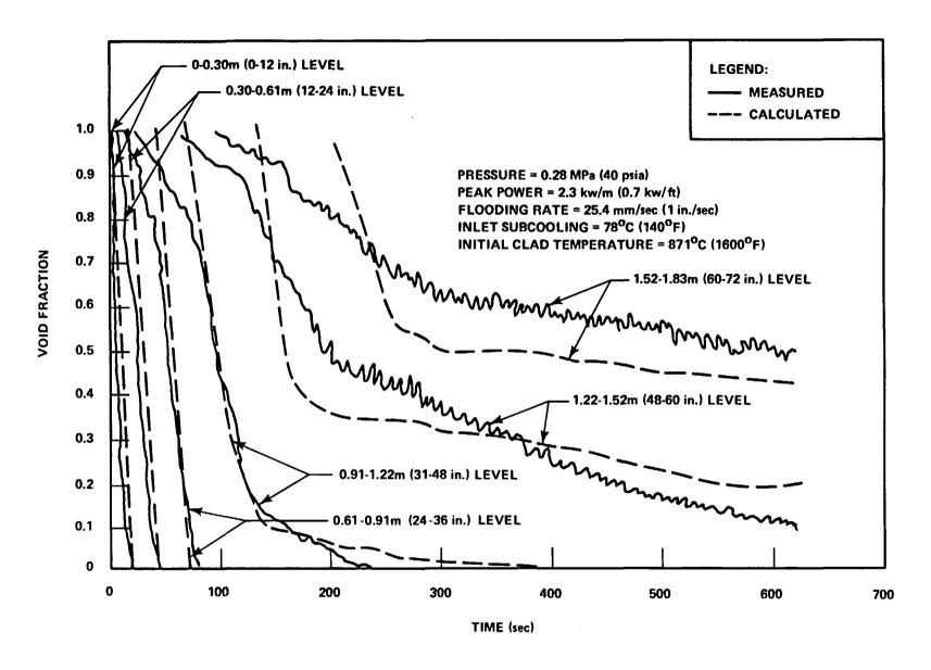
Figure 5-2. Comparison of Calculated and Measured Void Fraction, Run 31504 (sheet 1 of 2)
