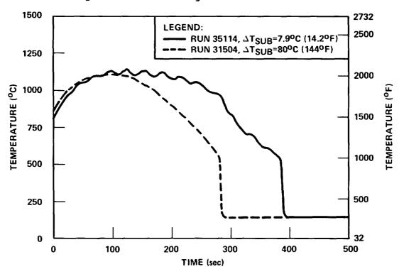
Figure 3-15. Subcooling Effect on Temperature
