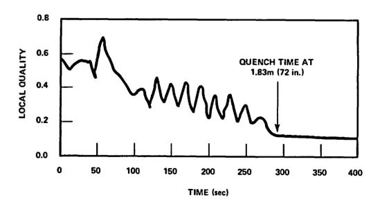
Figure B-28. Quality Transient, 1.83 m (72 in.) Elevation, Run 34006
