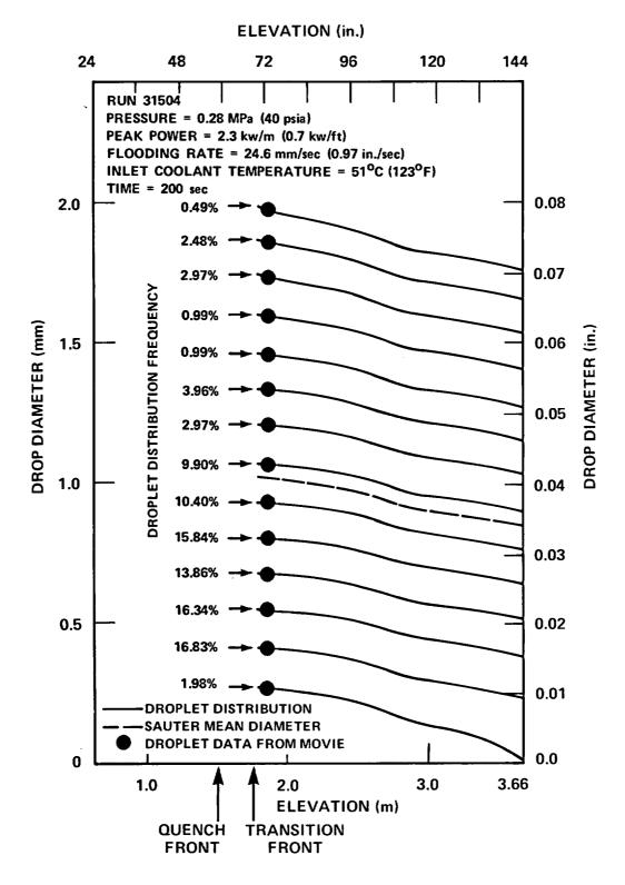
Figure 6-10. Calculated Drop Sizes in Dispersed Flow Regime
