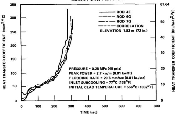
Figure H-18. Heat Transfer Coefficient Correlation Versus Data, Cosine Power Run 02603
