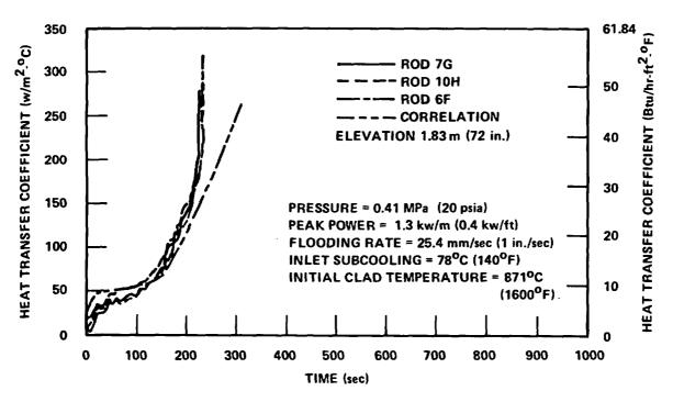
Figure H-14. Heat Transfer Coefficient Correlation Versus Data, FLECHT SEASET Run 39122
