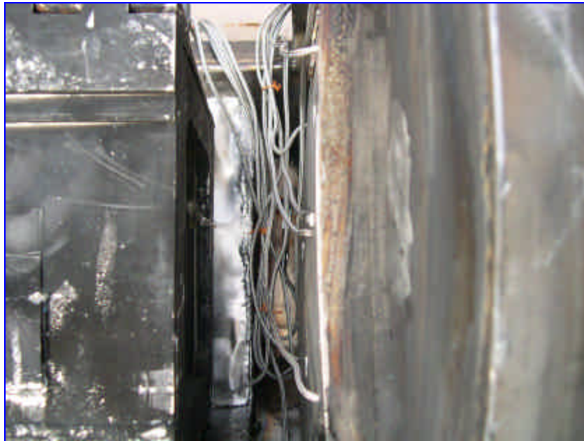
Figure 3-23 Outerpack Internals after December 15 Burn Test
