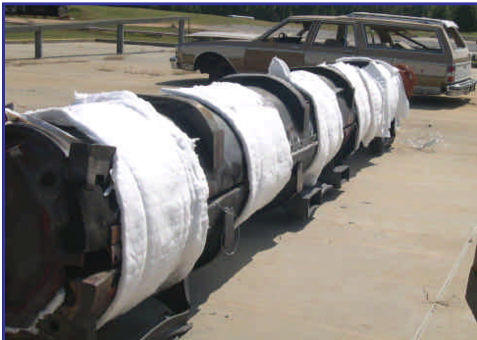
Figure 3-11 Package Exterior Wrapped with Ceramic Fiber Insulation
