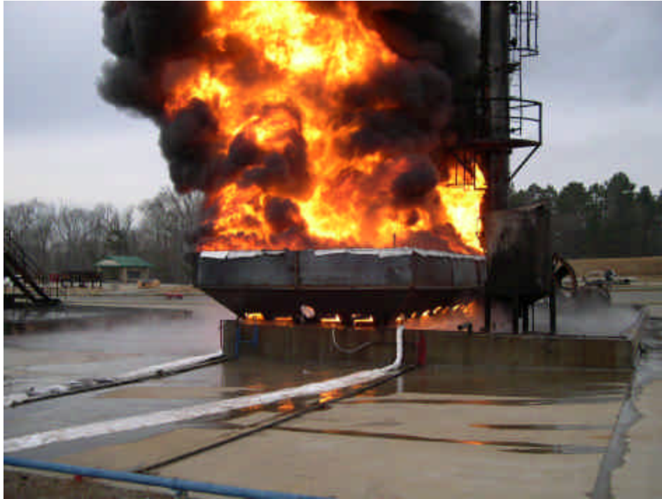
Figure 3-6 Traveller CTU During Pool Fire Test
