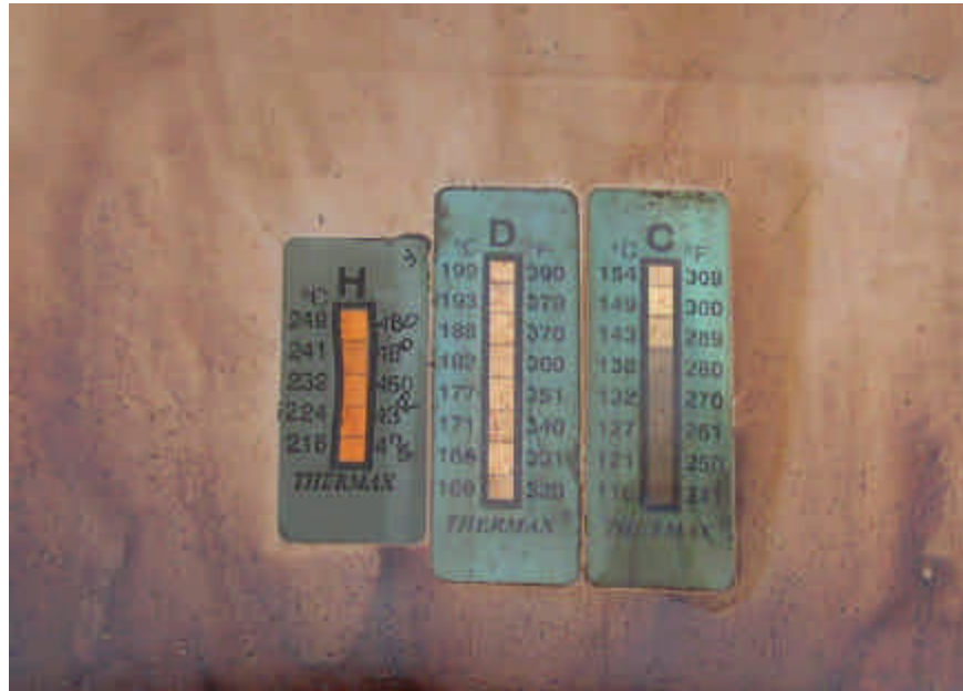
Figure 3-8 Temperature Strip Condition After CTU Burn Test
