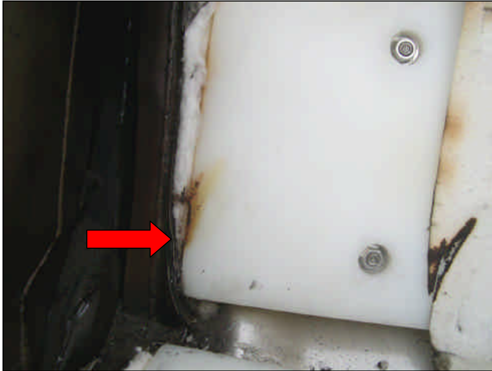
Figure 3-43 Location of Possible Combustion of Moderator
