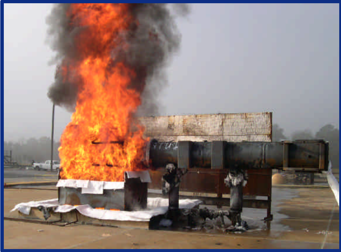
Figure 3-19 December 15, Impact Limiter Burn Test
