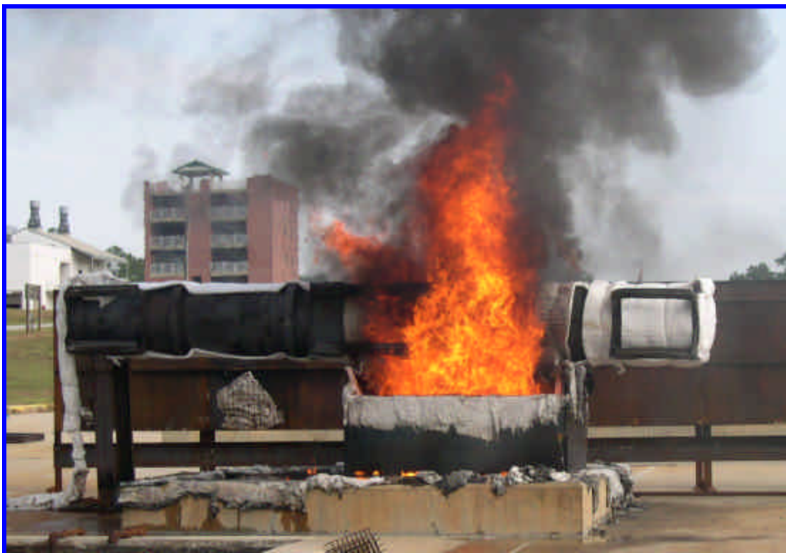
Figure 3-3 Seam Burn Test
