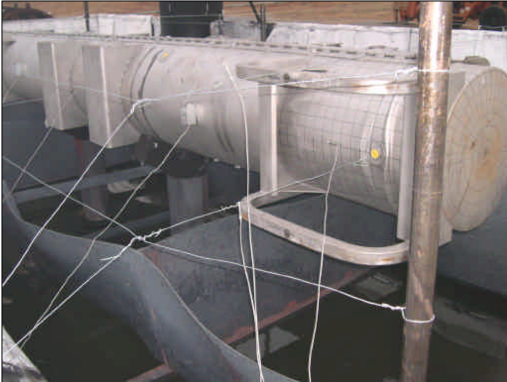
Figure 3-32 Test Stand for Fire Test
