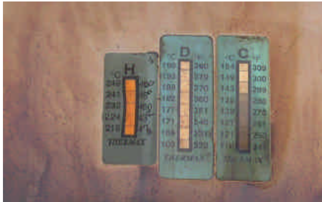
Figure 3-46 Temperature Strip Set After Fire Test
