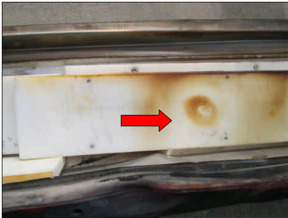
Figure 3-44 Localized Melt Spot in Lid Moderator Block
