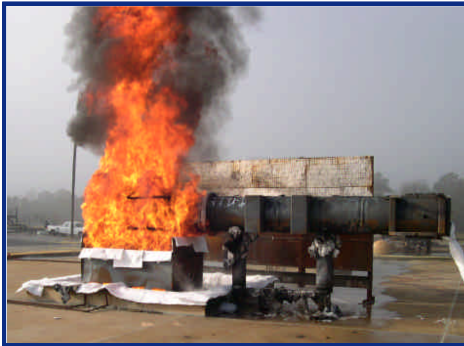
Figure 3-4 December 15, Impact Limiter Burn Test
