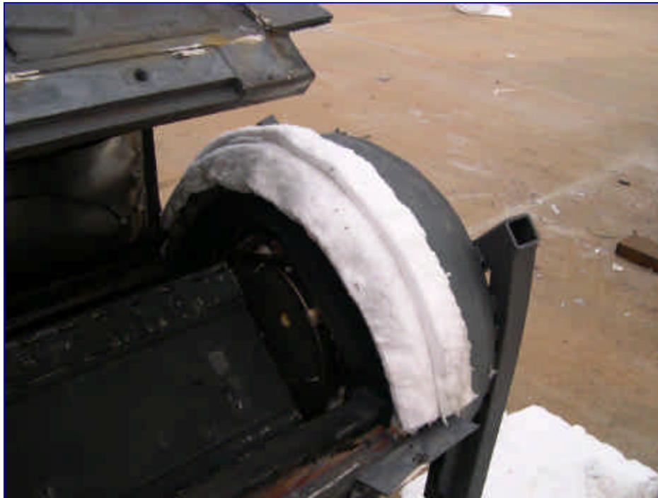
Figure 3-24 Kaowool Layers on Outerpack Bottom Impact Limiter
