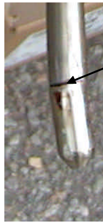
Figure 2-154 Cracked Rod From CTU Fuel Assembly
