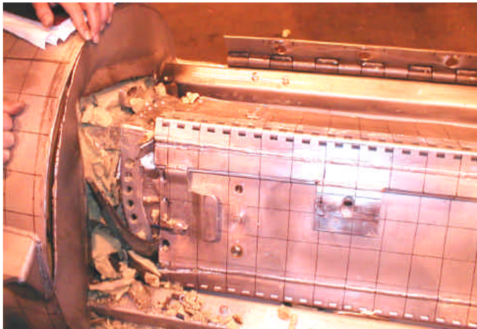
Figure 2-128 Traveller Prototype Clamshell and Bottom Impact Limiter After Test Series 3
