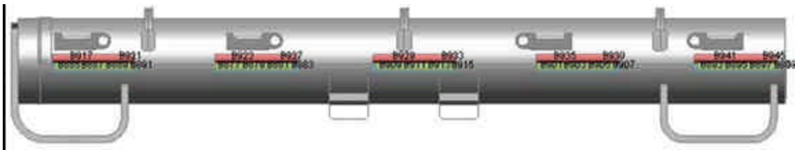
Figure 2-32 Bolt Labels for Right Outerpack
