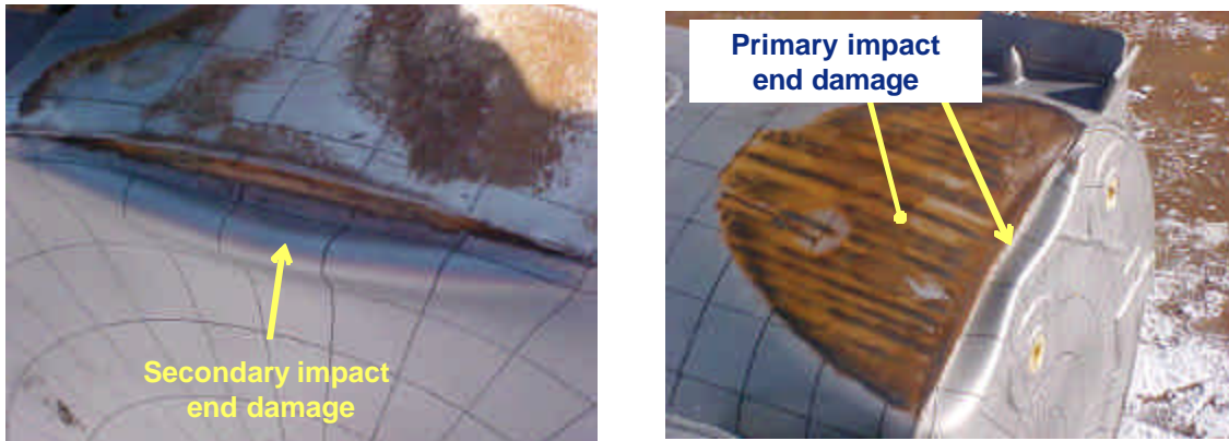
Figure 2-25 Damage from Prototype Low Angle Drop (Test 1.1)
