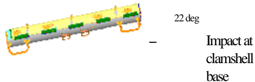
Figure 2-135 QTU Test Series 2 Drop Orientations
