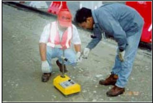
A typical moisture-density gauge in use.
