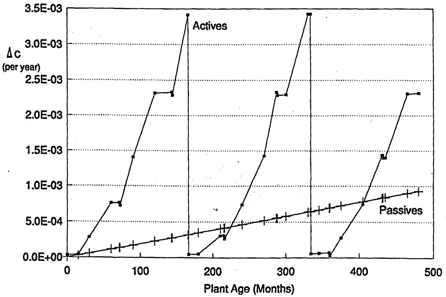
**FIGURE 5. SENSITIVITY ANALYSIS EVALUATING THE AGING CONTROL OF A GIVEN TEST AND MAINTENANCE PROGRAM**
