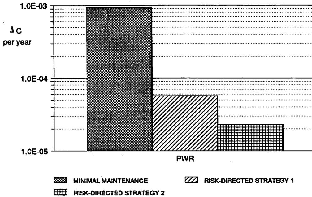
**FIGURE 8. RELATIVE CORE DAMAGE FREQUENCY INCREASE DUE TO AGING:
