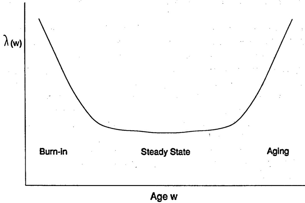
**FIGURE 2. THE BATHTUB CURVE OF FAILURE RATE VERSUS AGE**
