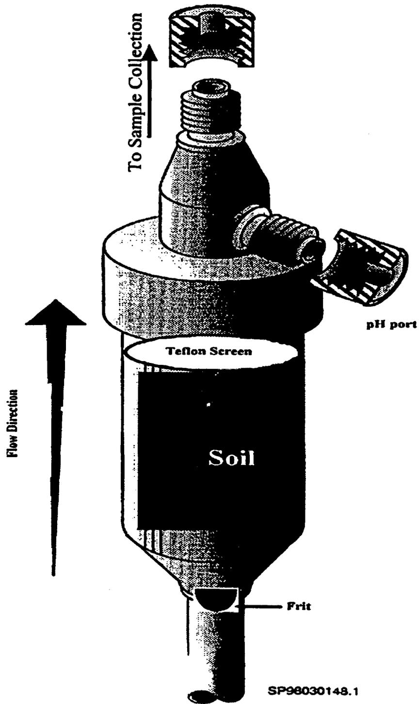
Figure 3- 1. Schematic of Column Apparatus.
