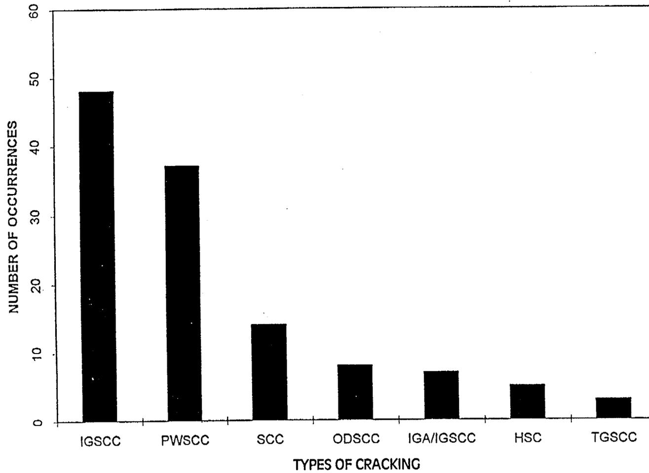
Figure 2-8 Passive Structures and Components - Degradation Occurrences Distribution By Type of Cracking Induced By Corrosion
