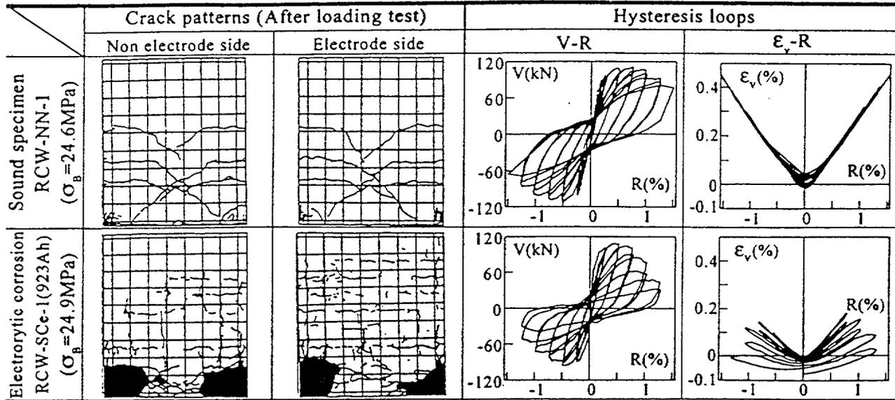
a: Shear Walls (Top - Non-Degraded; Bottom - Degraded)
