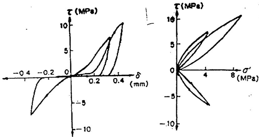
(a) Shear stress ( $\tau$ ) vs. Shear Deformation ( $\delta$ ) Relationship
