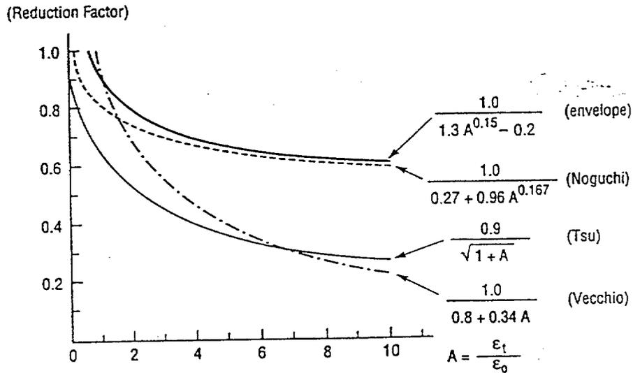
Fig. 10: Compressive Strength Reduction Factors for Cracked Concrete
