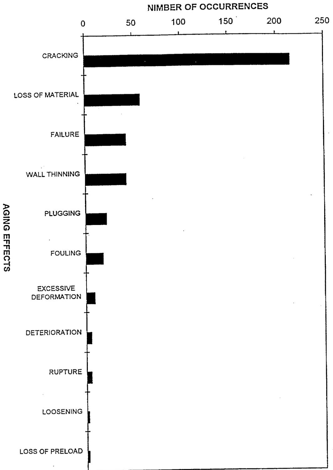
Figure 2-5 Passive Structures and Components - Degradation Occurrences
