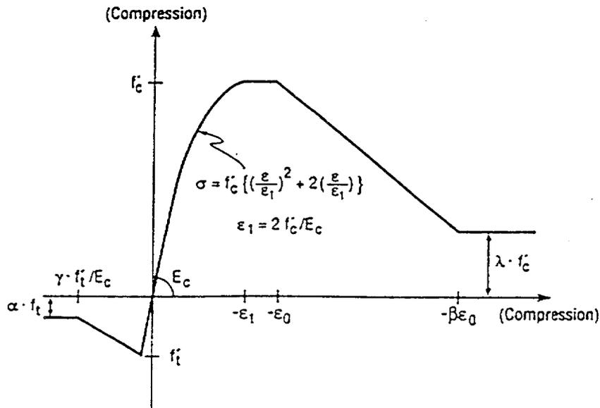
Fig. 8: Envelope Curve for Concrete
