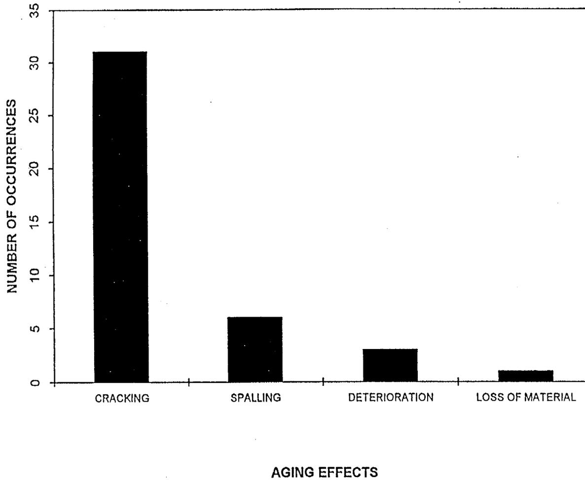
Figure 2-6 Passive Structures and Components - Degradation Occurrences
