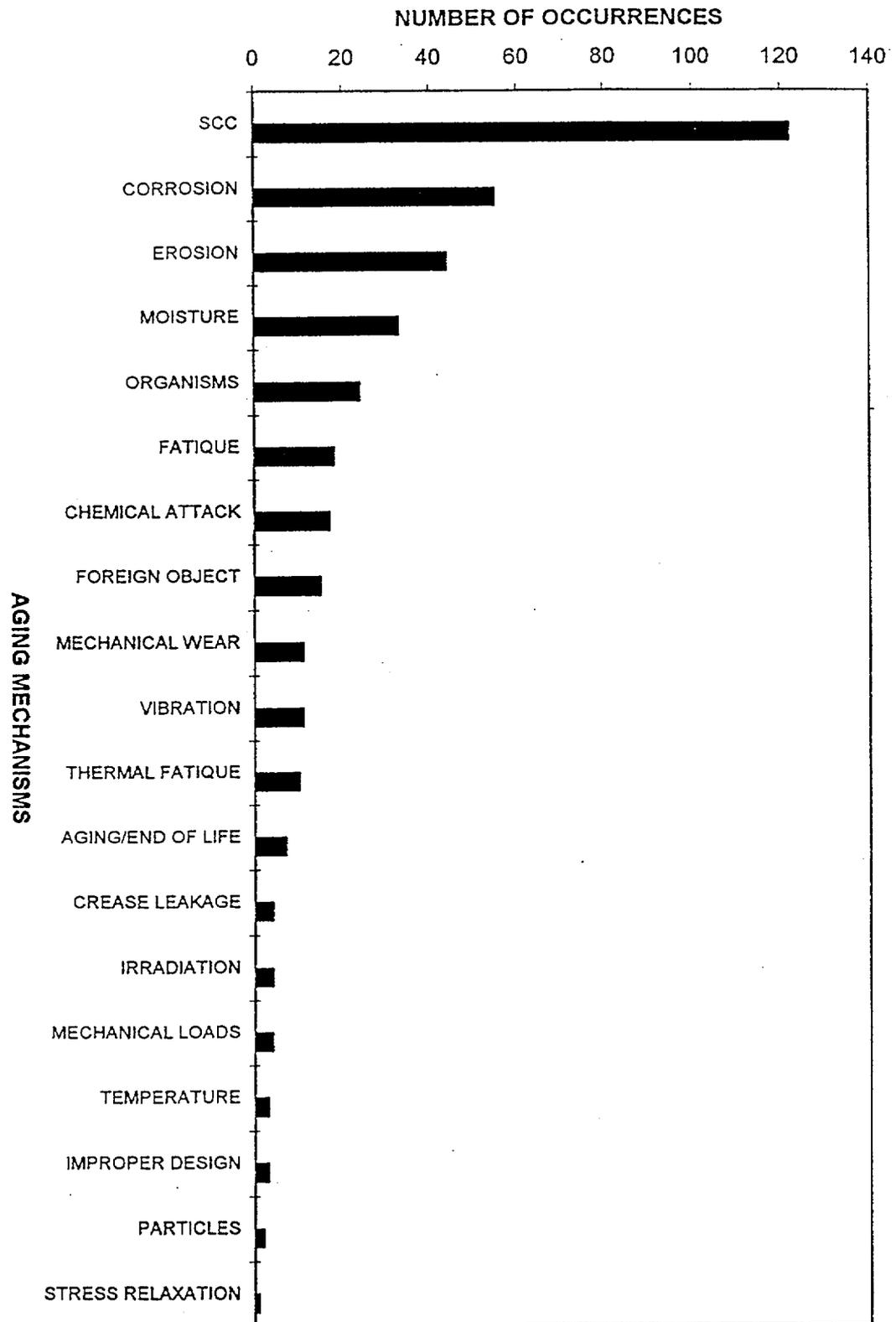
Figure 2-7 Passive Structures and Components - Degradation Occurrences
