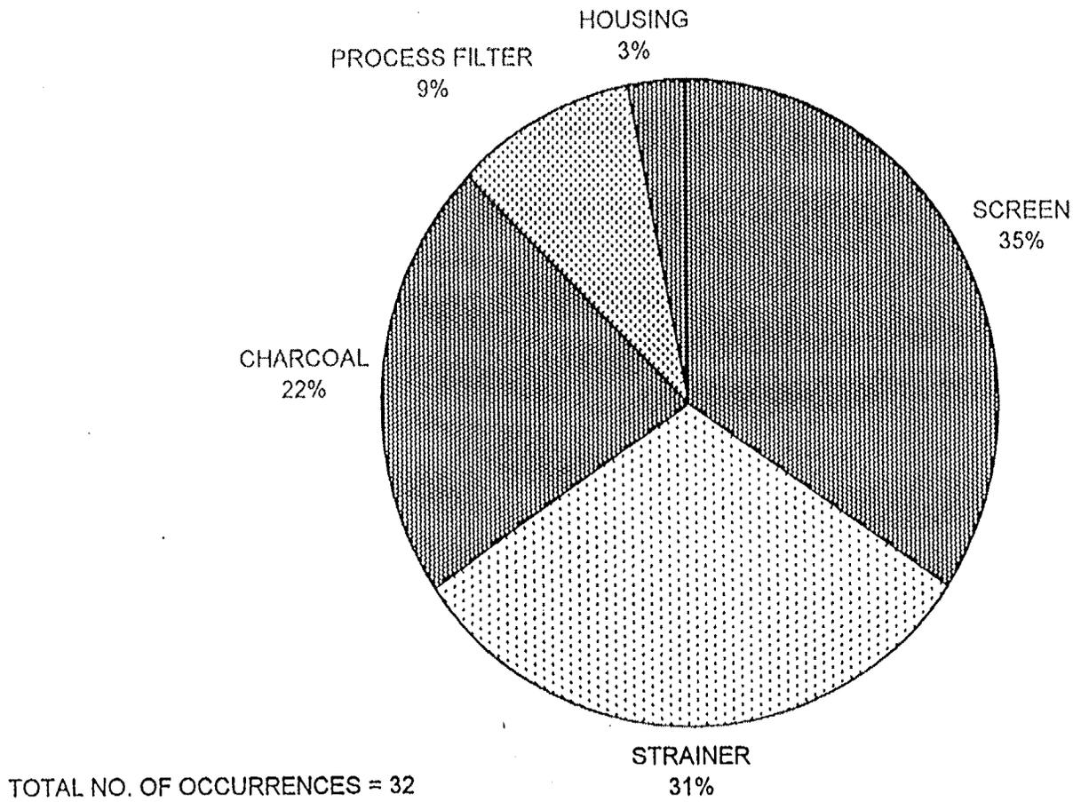
Figure 2-12 Passive Structures and Components - Degradation Occurrences
