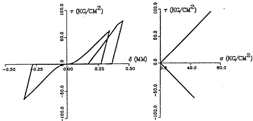
(a) Shear Stress vs. Shear Deformation Relationship
