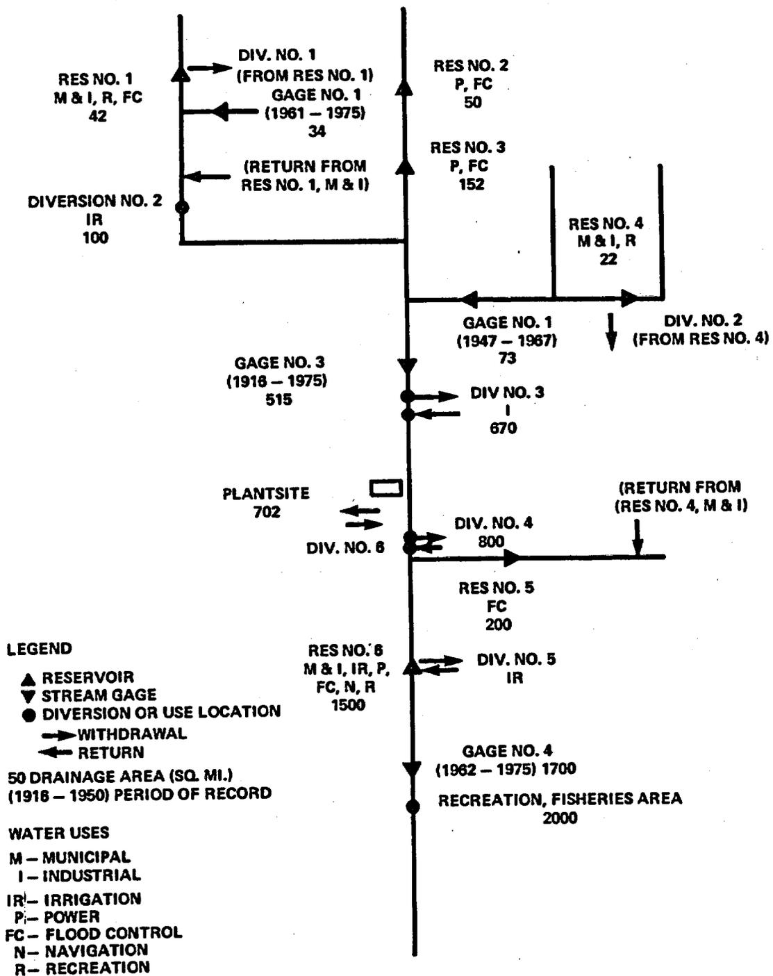
FIGURE 16. TYPICAL SCHEMATIC DIAGRAM OF A RIVER BASIN
