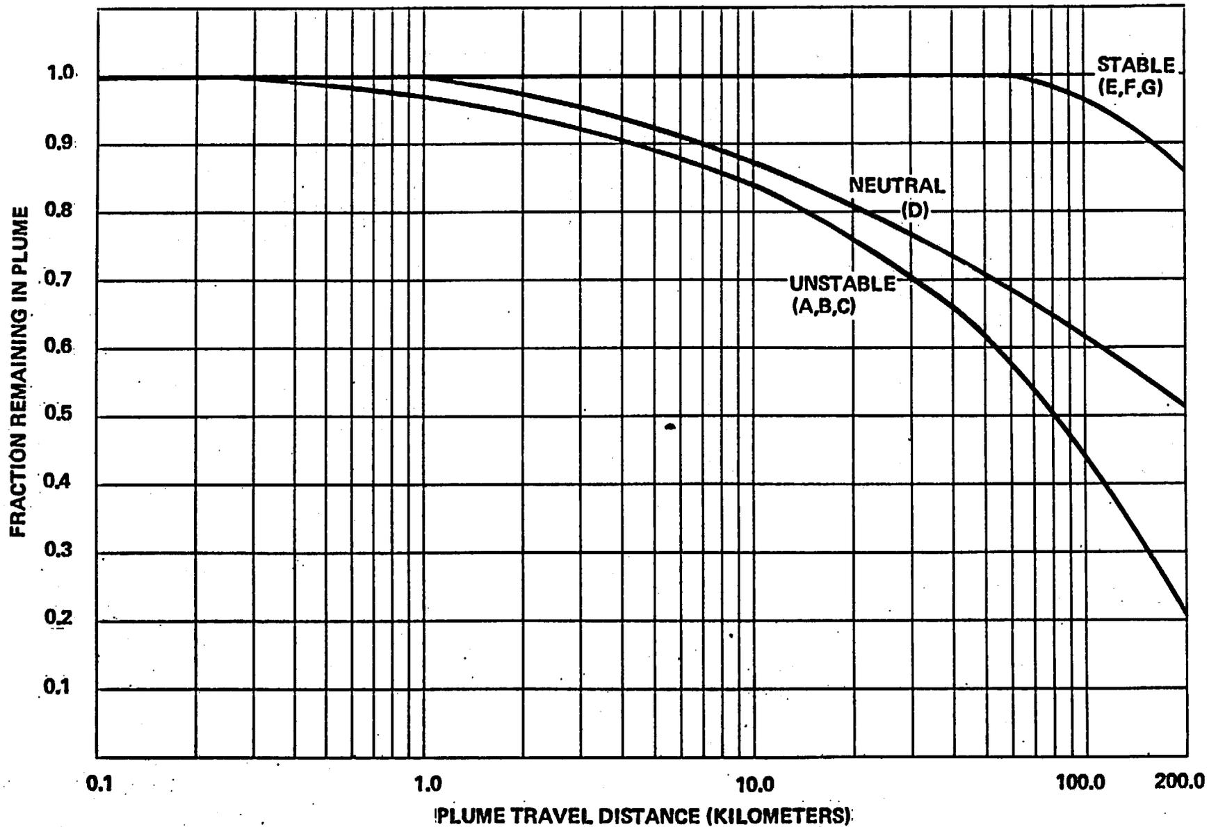
Figure 4. Plume Depletion Effect for 60-m Releases (Letters denote Pasquill Stability Class)
