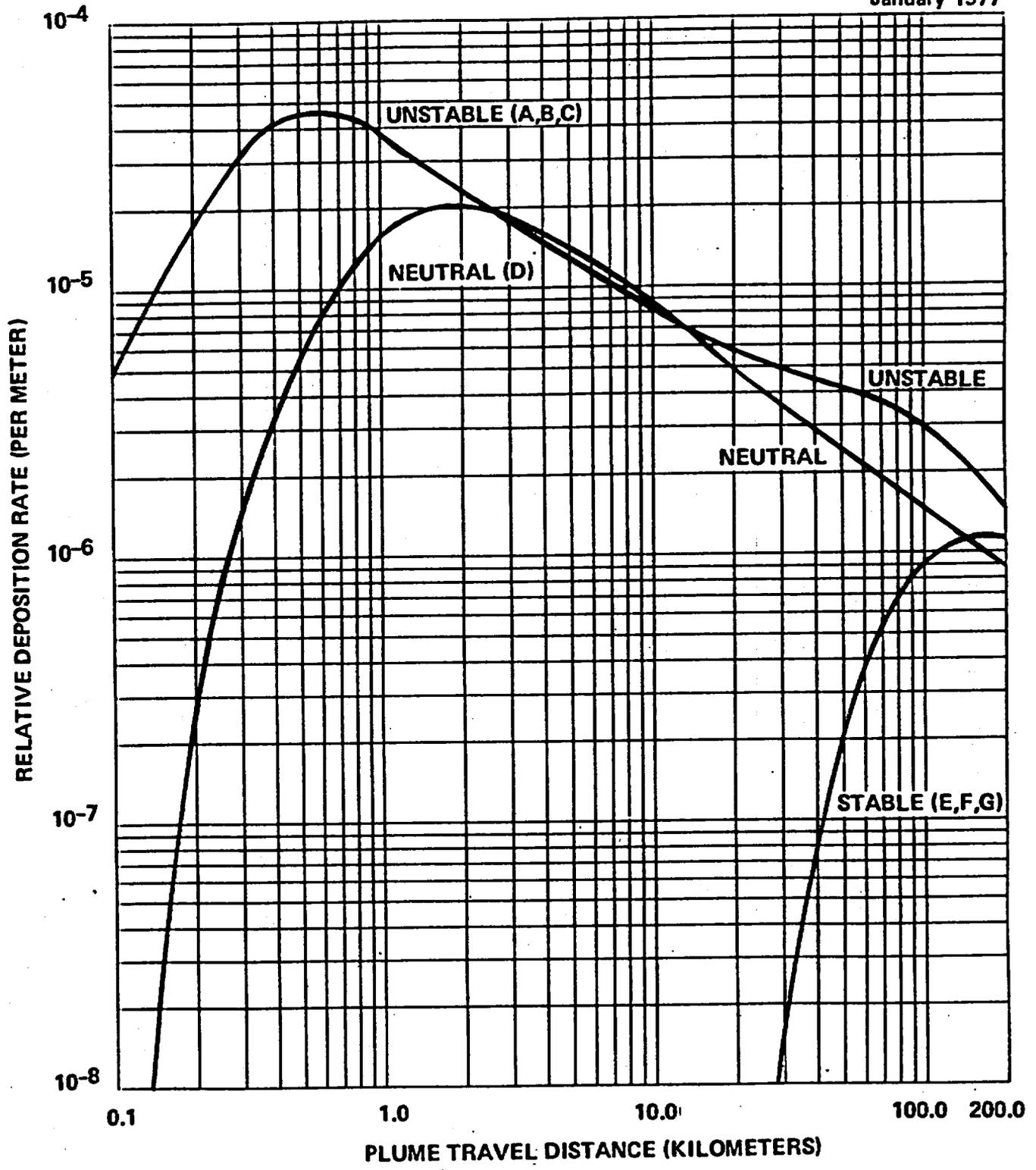
Figure 9. Relative Deposition for 60m Releases (Letters denote Pasquill Stability Class)
