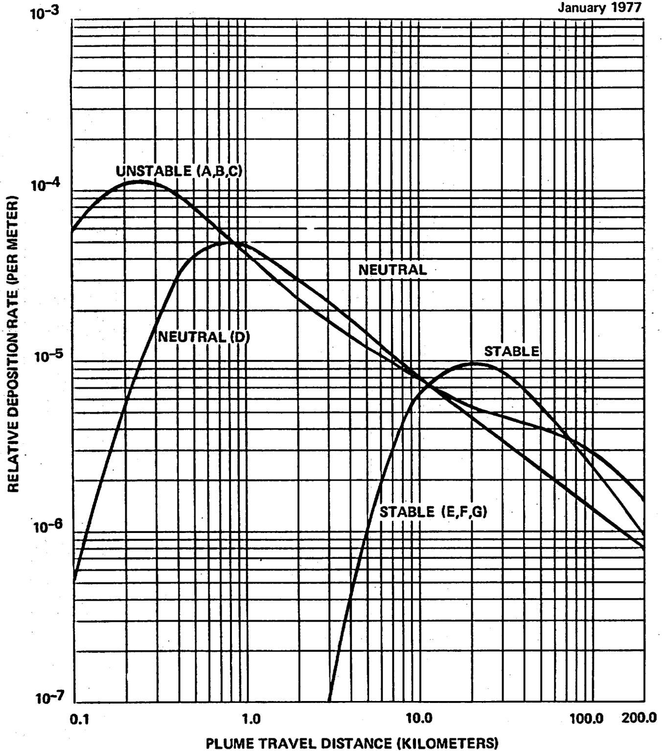
Figure 8. Relative Deposition for 30m Releases (Letters denote Pasquill Stability Class)
