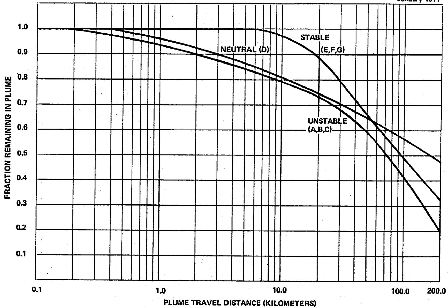
Figure 4. Plume Depletion Effect for 30m Releases (Letters denote Pasquill Stability Class)
