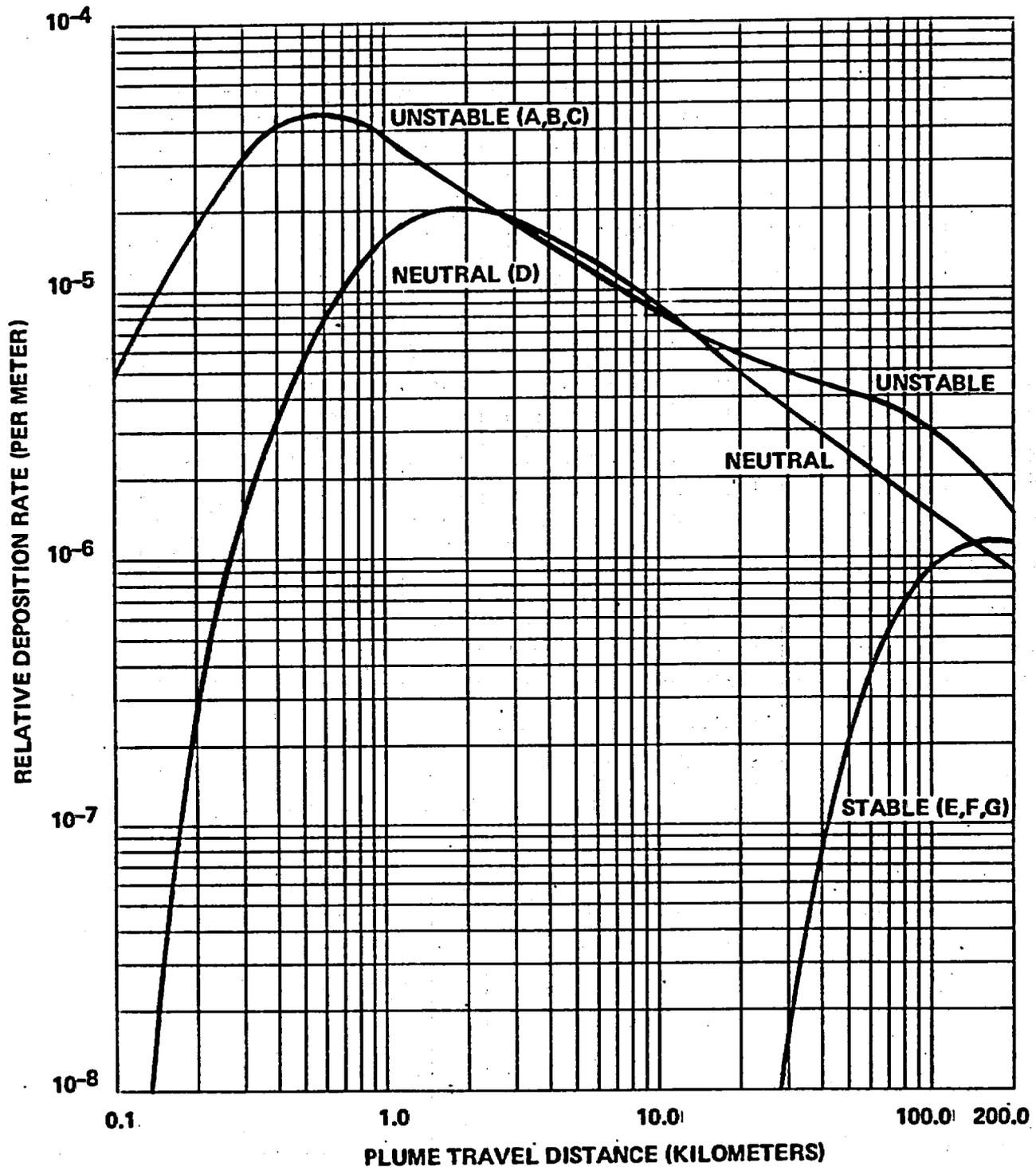
Figure 8. Relative Deposition for 60-m Releases (Letters denote Pasquill Stability Class)
