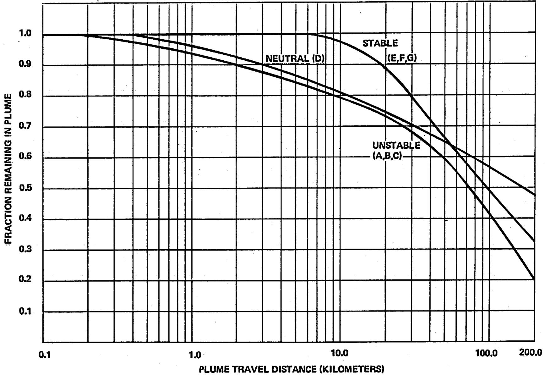
Figure 3. Plume Depletion Effect for 30-m Releases (Letters denote Pasquill Stability Class)
