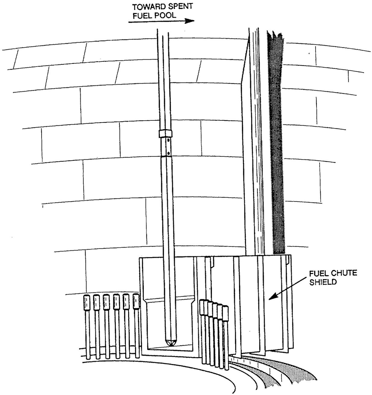
Figure B-3 Portable Radiation Shield
