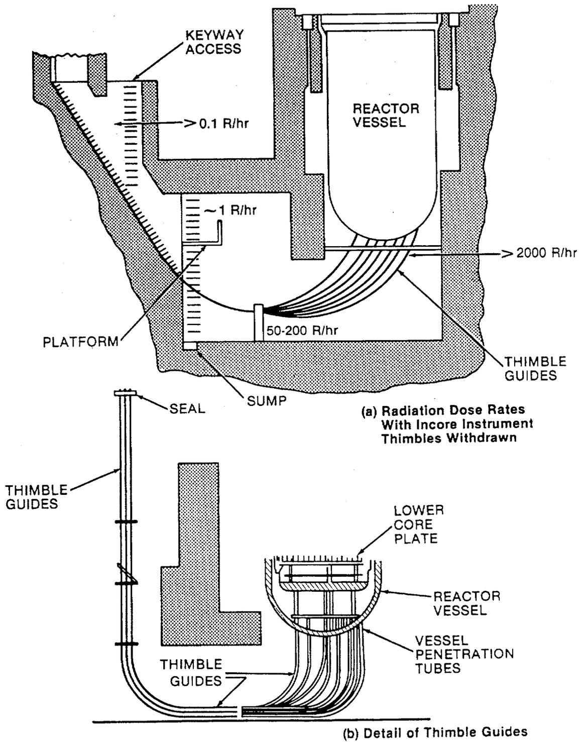
Figure B-1 Pressurized Water Reactor Cavity
