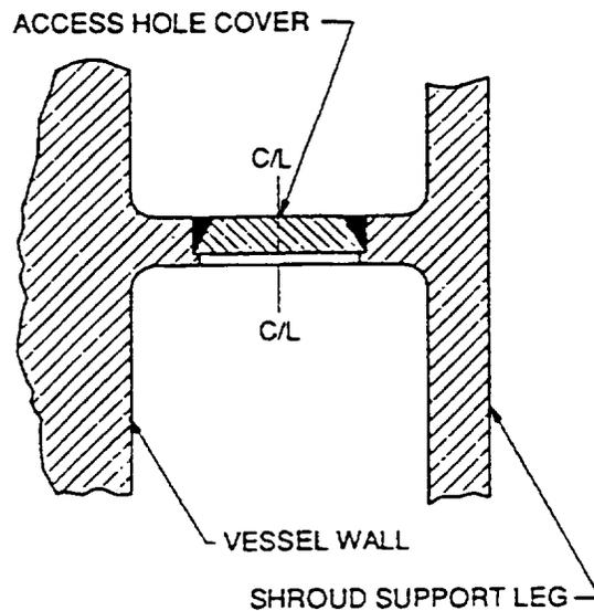
Figure 2-12. Access hole cover plate.
