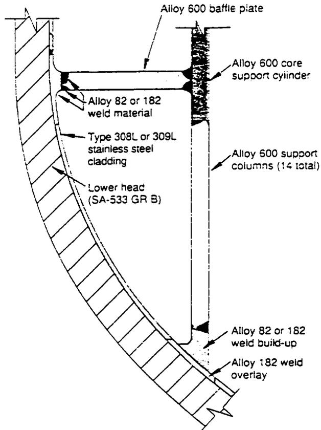
Figure 2-11. Typical core shroud support materials and weldments.
