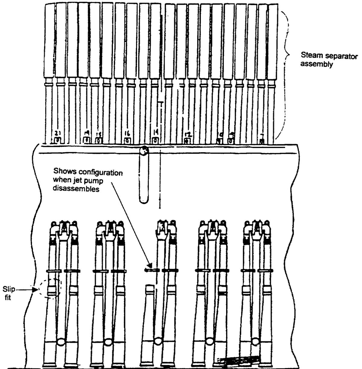
Figure 4-3. Probable jet pump disassembly from hold-down beam failure.
