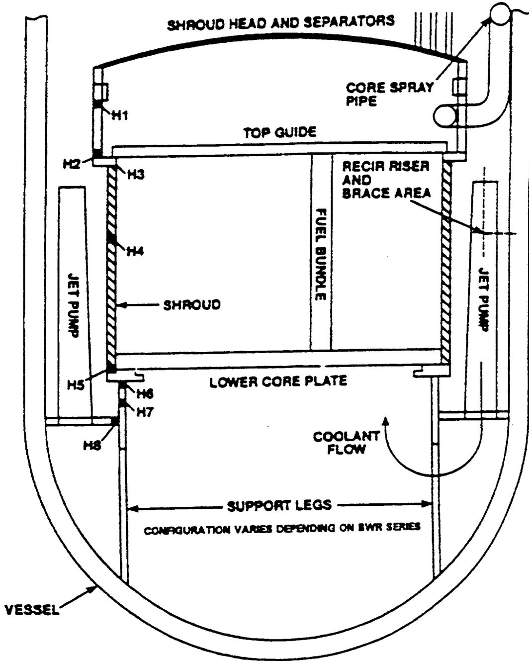
Figure 3-1. Typical core shroud weld locations.
