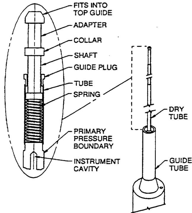
**Figure 2-5.** In-core instrumentation dry tube.
