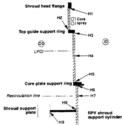
Typical Weld Locations in Core Shroud
