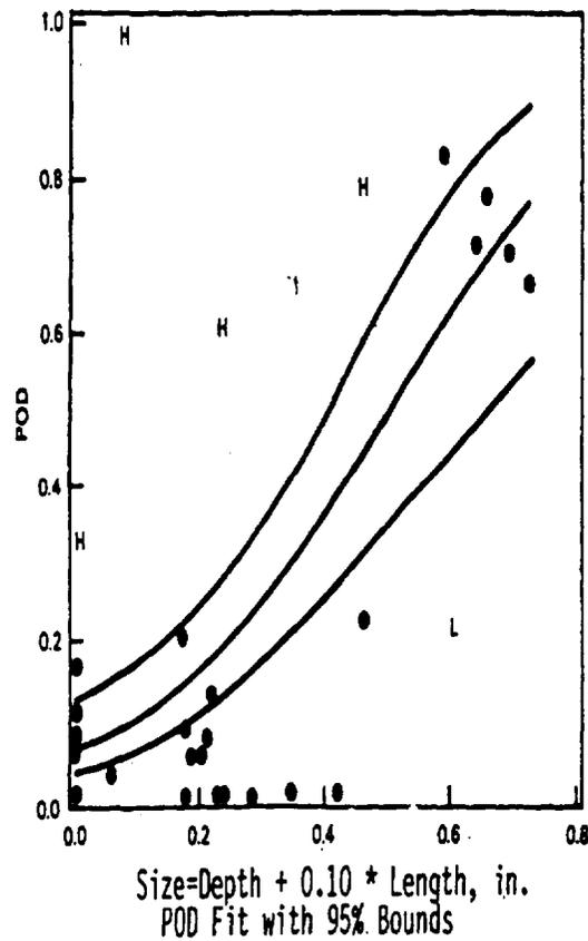
**Figure 10-5.** Logistic curve fit to POD data versus crack size for near-side thermal fatigue cracks in wrought stainless steel material (Doctor et al., 1988).
