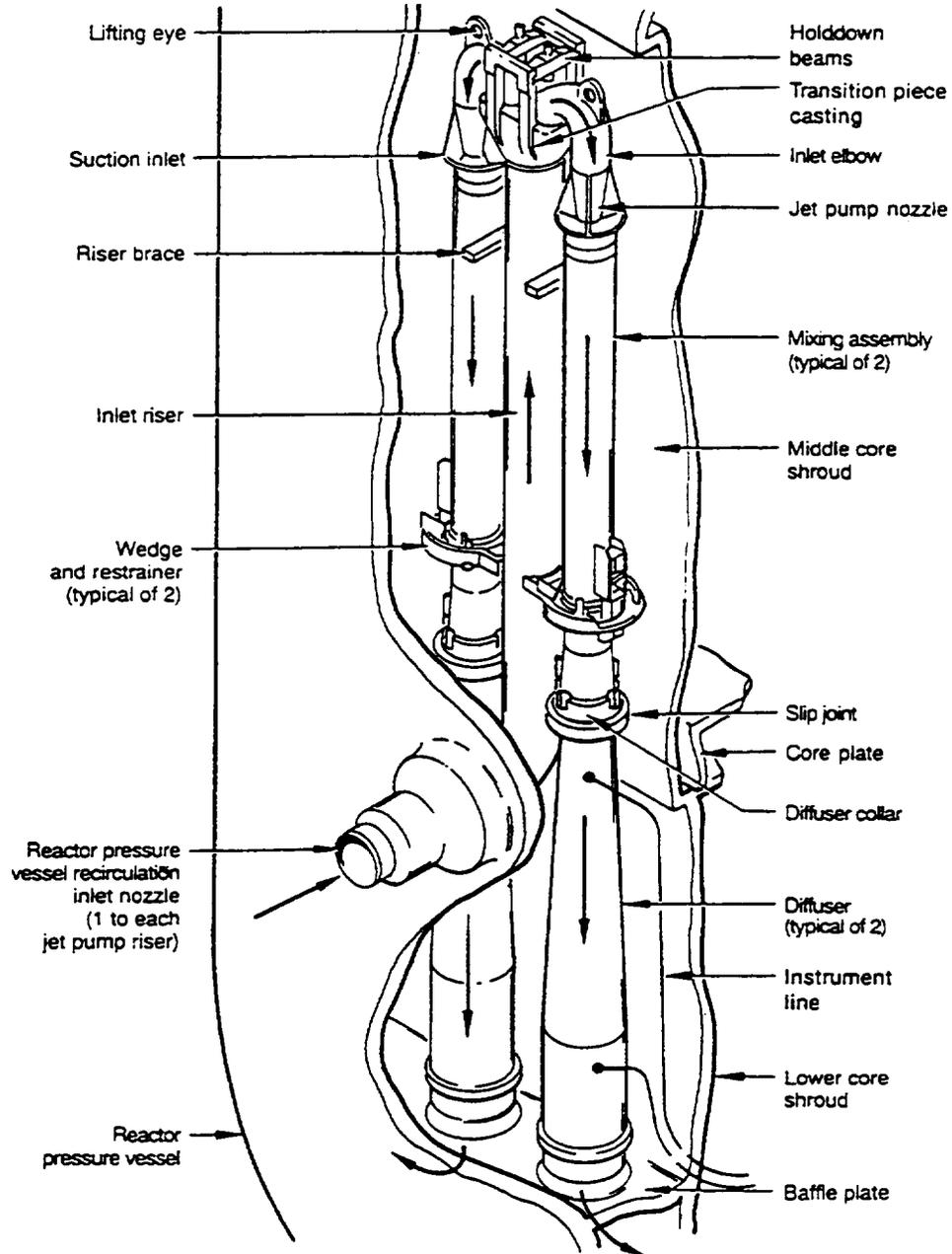
Figure 2-21. Jet pump assembly.
