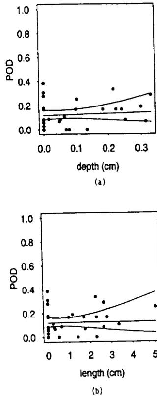
**Figure 10-3.** Logistic curve fit to POD data with 95% bounds (wrought SS with IGSCC, far-side inspection, all teams). a) POD vs. depth, b) POD vs. length (Heasler and Doctor 1996).
