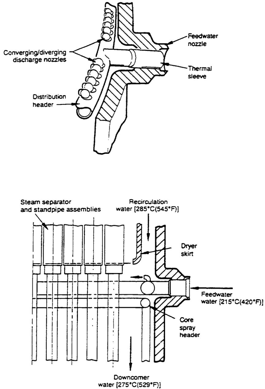
Figure 2-20. Feedwater sparger with nozzles.
