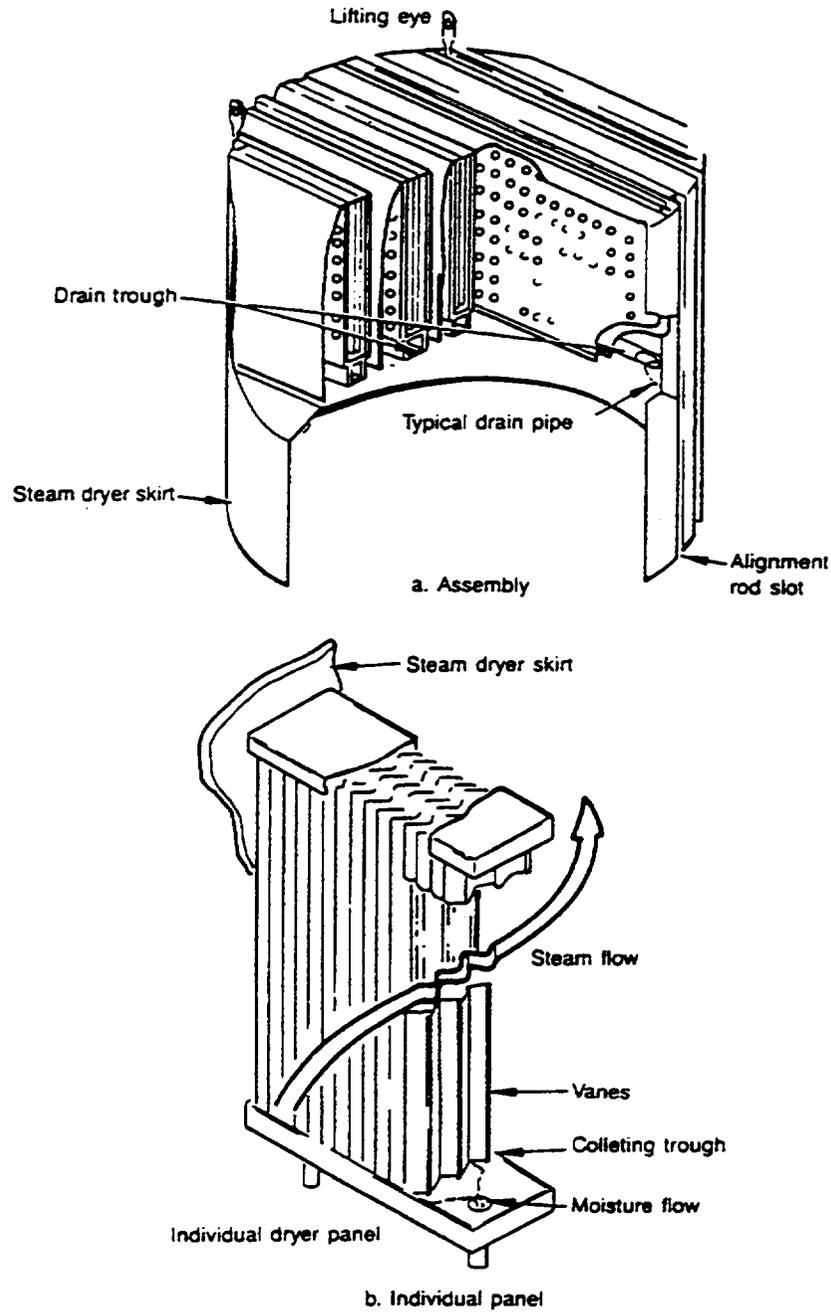
Figure 2-24. Steam dryer assembly.
