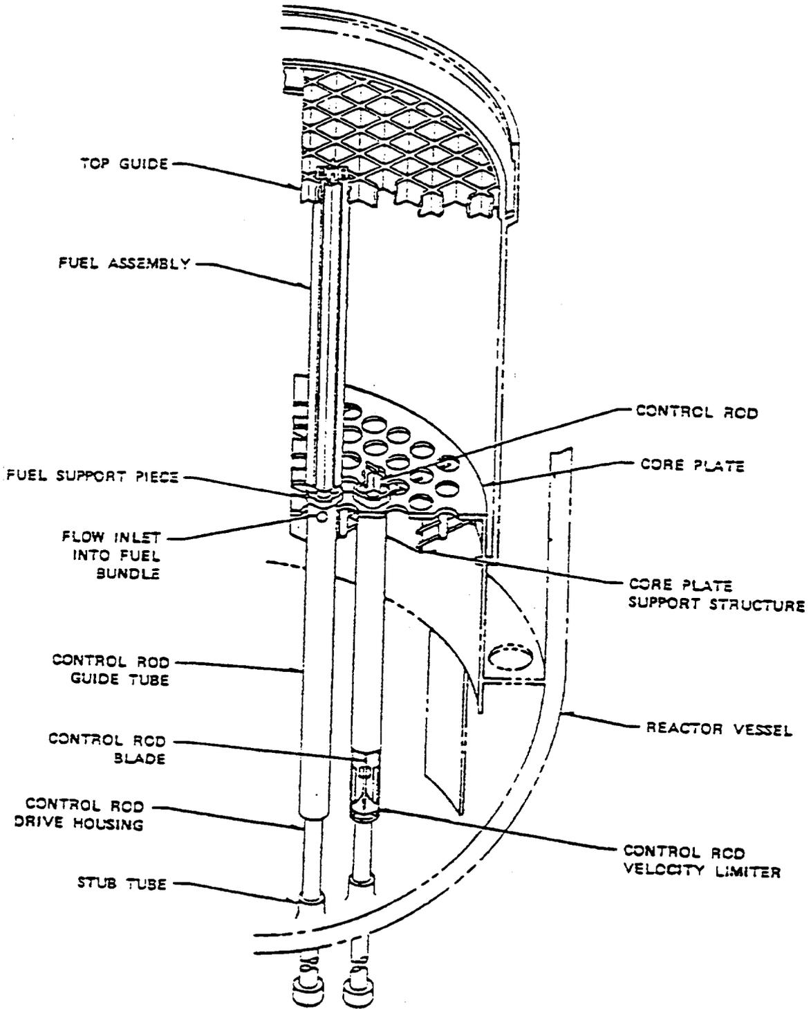
Figure 2-6. Typical control rod and drive assembly inside the reactor vessel.
