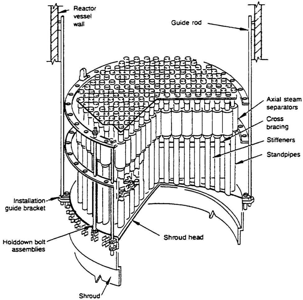
**Figure 2-15.** Arrangement of core shroud head, head bolts, standpipes, steam separators, and guide rods.
