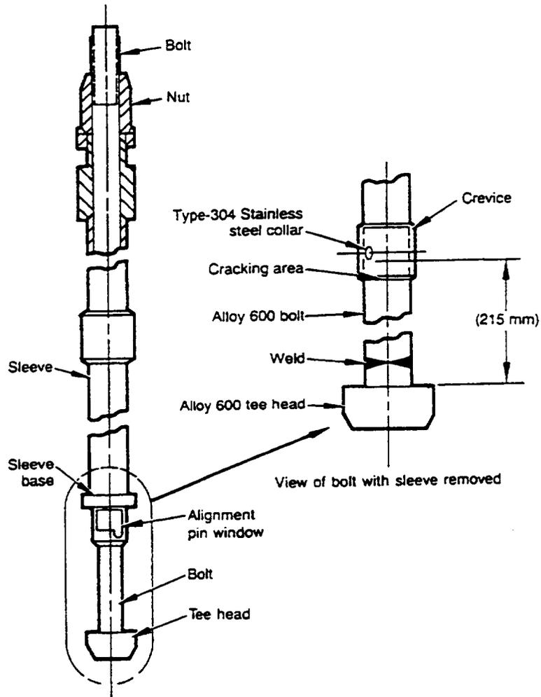
Figure 2-16. Core shroud head bolts.
