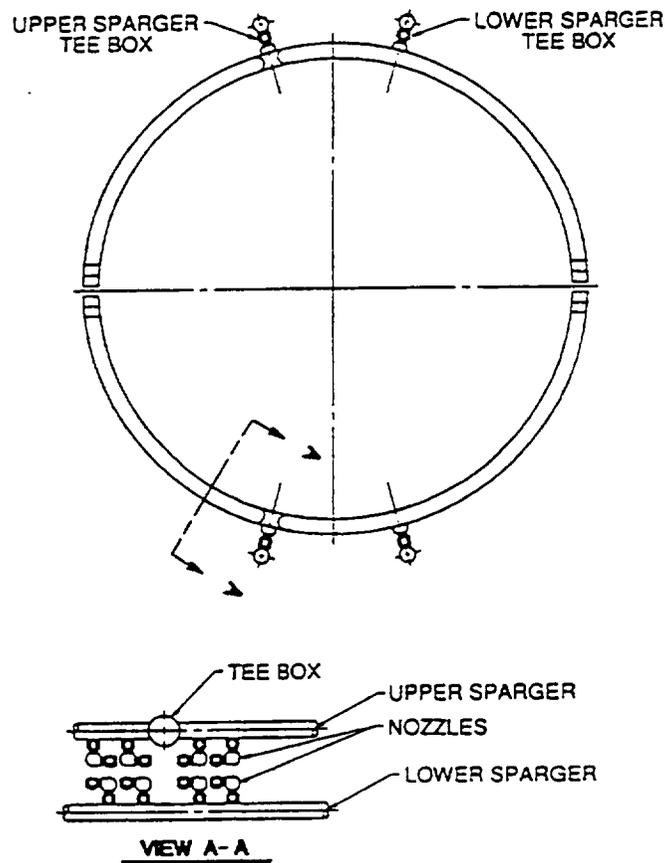
Figure 2-18. Core spray sparger.
