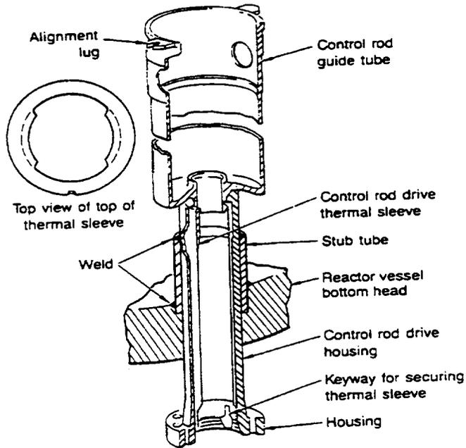
Figure 2-8. Typical control rod drive housing, stub tube, and guide tube arrangement.
