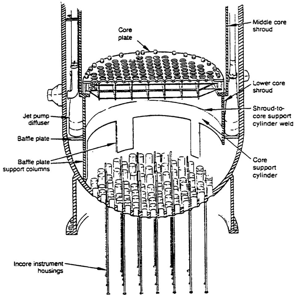
Figure 2-13. Lower plenum region internals including core plate.
