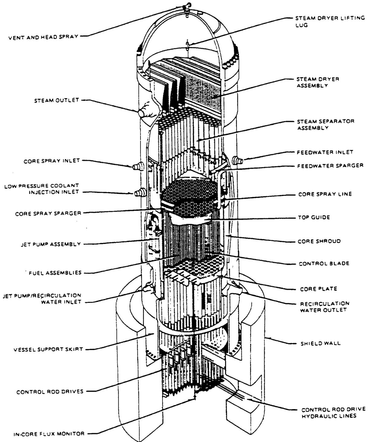
Figure 2-3. BWR/5 or BWR/6 reactor vessel internals.
