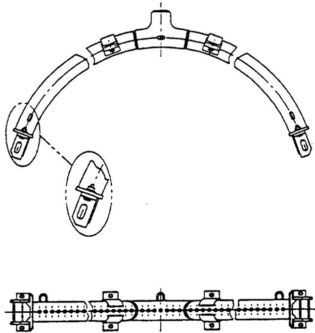
**Figure 2-19.** Feedwater sparger with holes.
