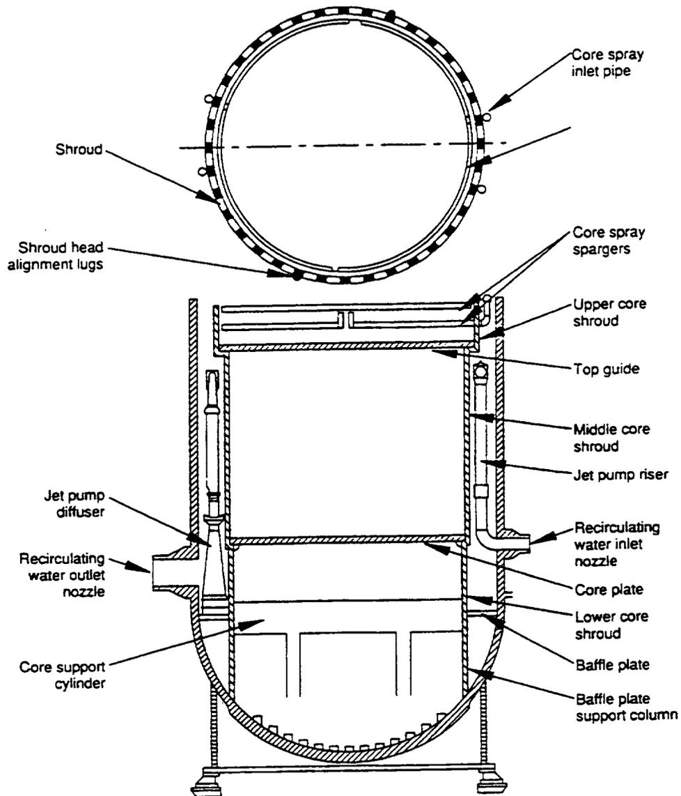
Figure 2-14. Arrangement of core shroud, core spray spargers, core shroud support, and jet pumps.
