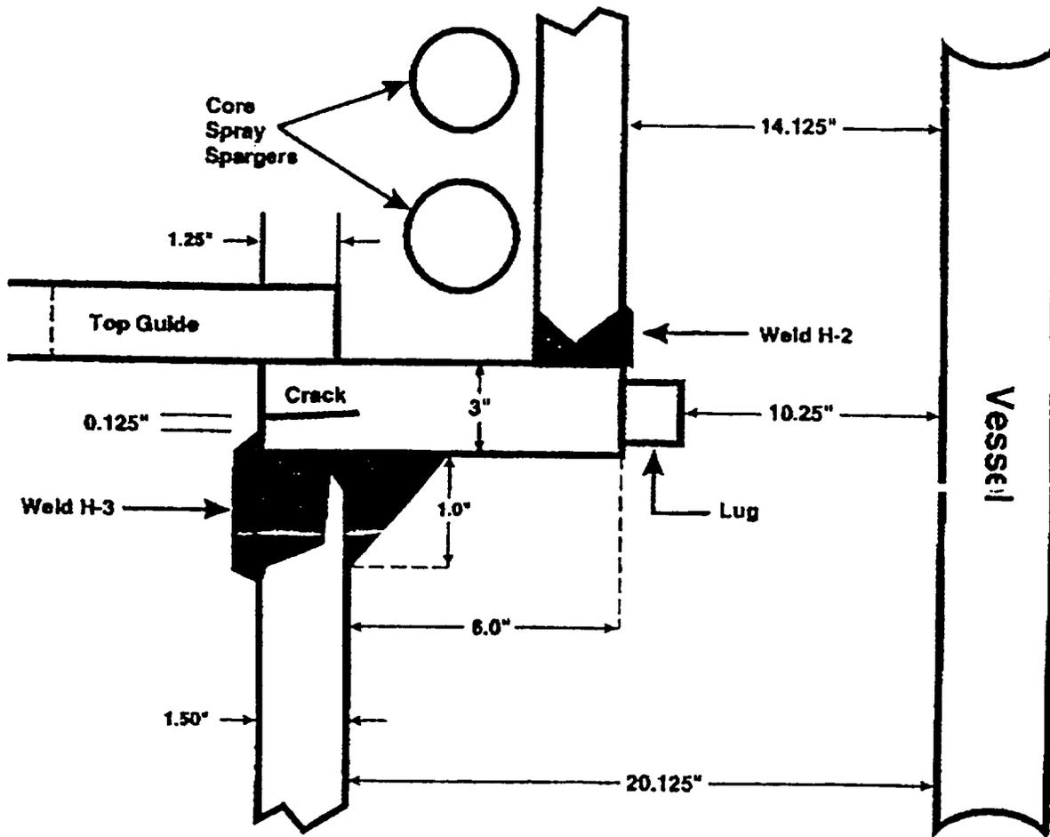
Figure 3-2. Details of Brunswick Unit 1 significant core shroud cracking.
