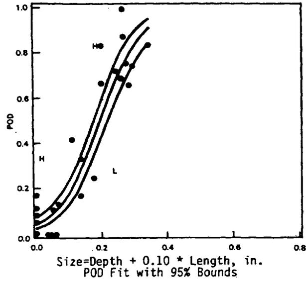
**Figure 10-4.** Logistic curve fit to POD data versus crack size for near-side IGSCC cracks in wrought stainless steel material (Doctor et al., 1988).
