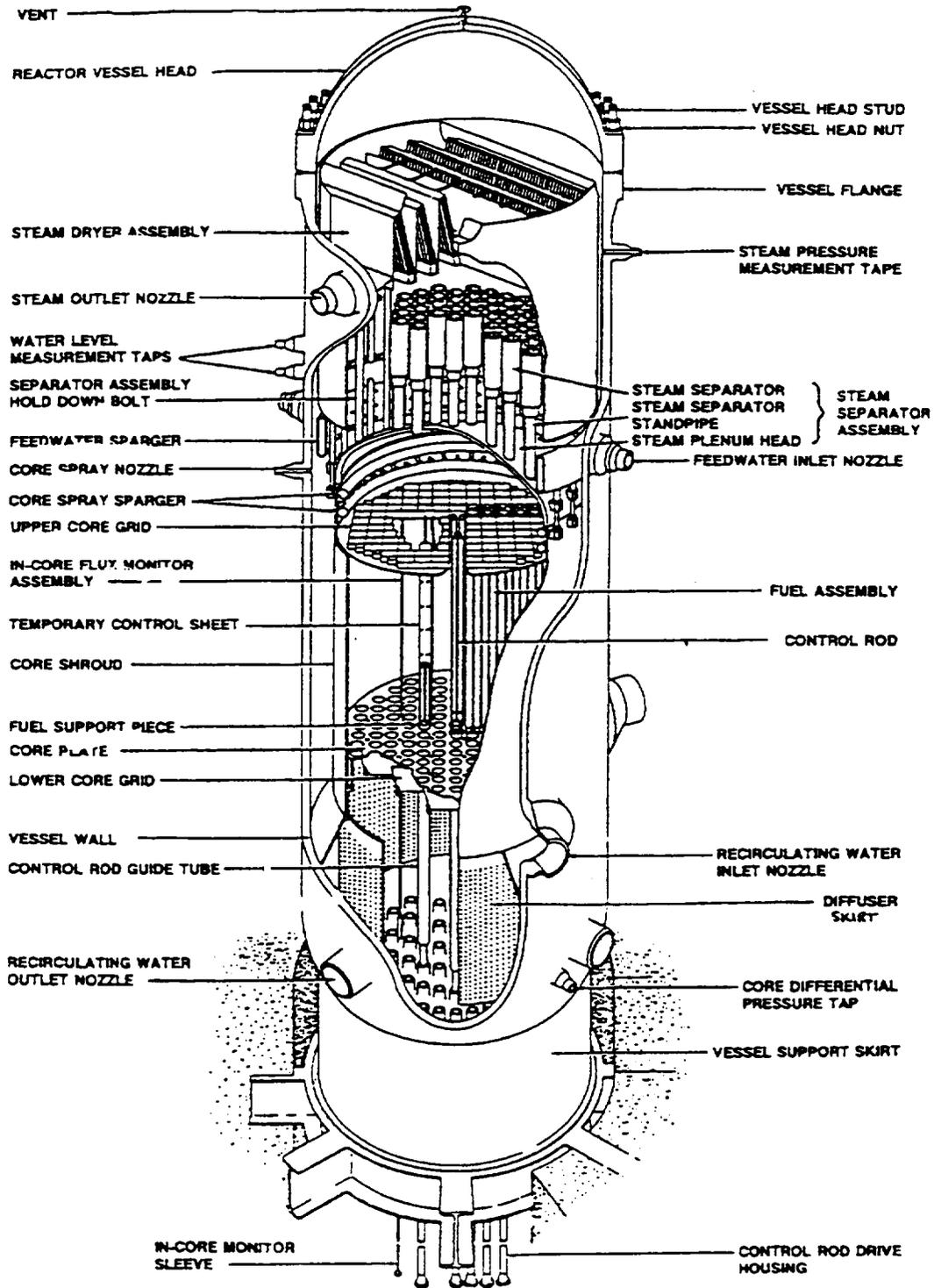
Figure 2-1. BWR/2 reactor vessel internals.
