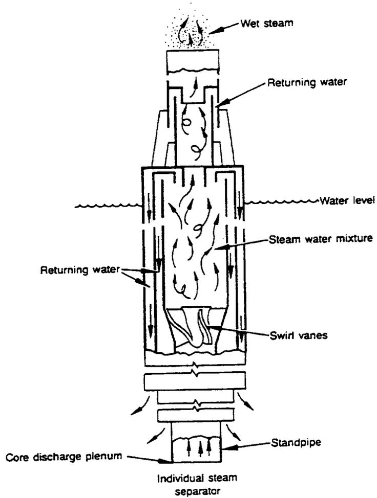
Figure 2-23. Steam separator assembly.
