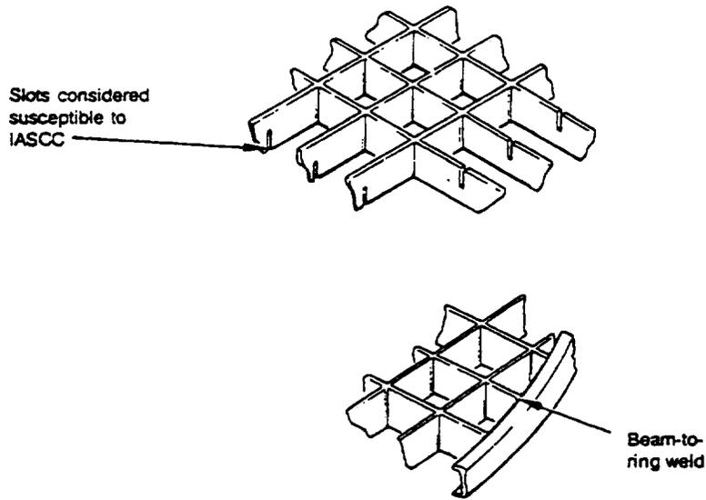
Figure 2-17. Fabrication details of typical BWR/2 through BWR/5 top guide.
