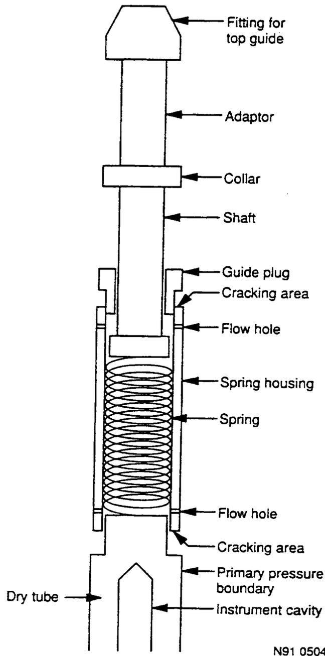
**Figure 4-5.** Location of dry tube cracking.
