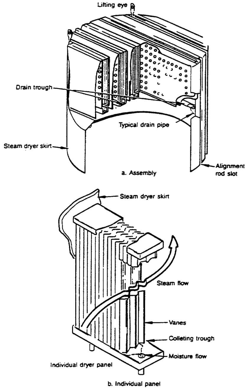
Figure 2-24. Steam dryer assembly.
