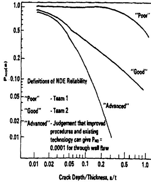
**Figure 10-1.** Probability of non-detection ( $P_{ND}$ ) of IGSCC in 254 mm (10 in.) stainless steel pipe (Simonen, 1990).
