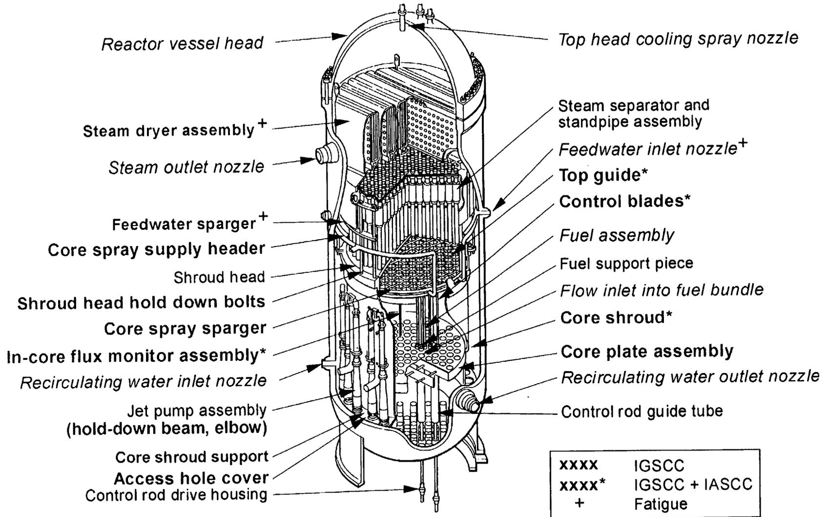
**Figure 1-1.** BWR reactor internal components that have experienced IGSCC damage.
