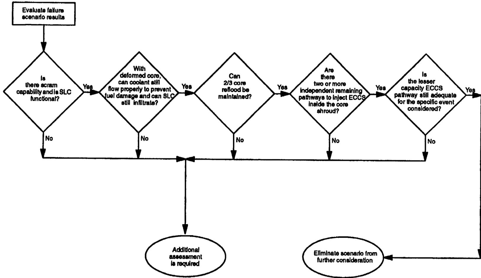
Figure 6-1. Screening logic for the elimination of low-safety-impact scenarios during initiating events.
