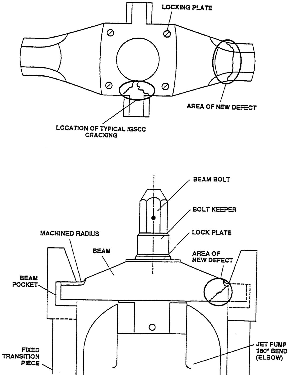
Figure 4-2. Location of cracking in jet pump hold-down beams.
