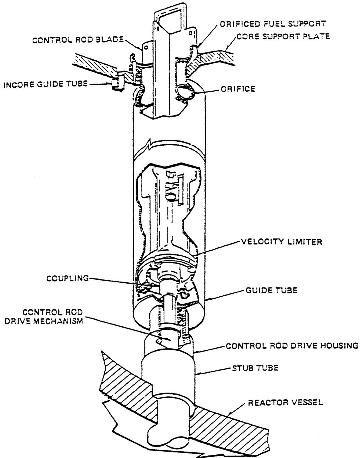
Figure 2-9. Control rod arrangement in lower plenum.
