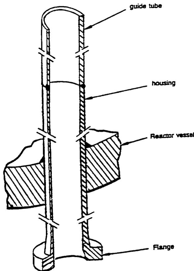
**Figure 2-4.** In-core instrumentation housing and guide tube.
