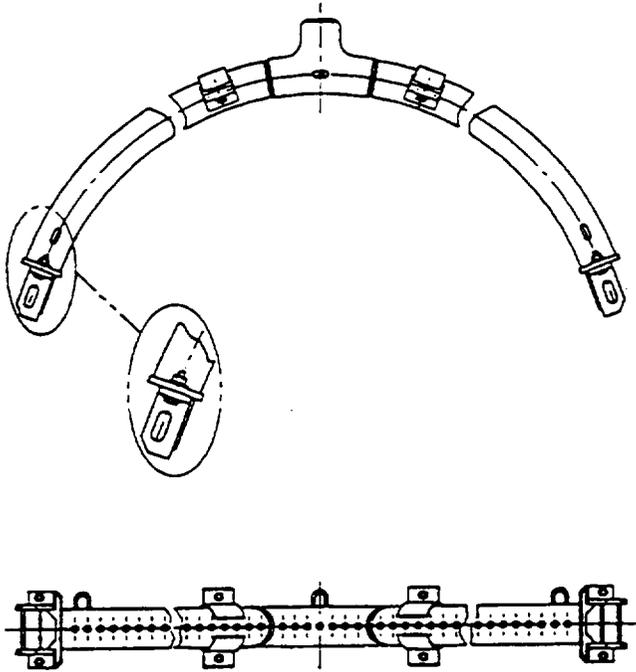
Figure 2-19. Feedwater sparger with holes.
