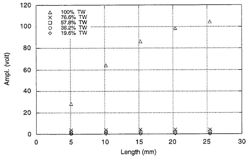
Fig. 3.12. Measured differential peak-to-peak signal amplitude (in volts) as a function of length by 18.3-mm (0.72-in.)-diameter magnetically biased bobbin coil on 25-notch EDM standard at (a)  $f = 100$  kHz, and (b)  $f = 400$  kHz.
