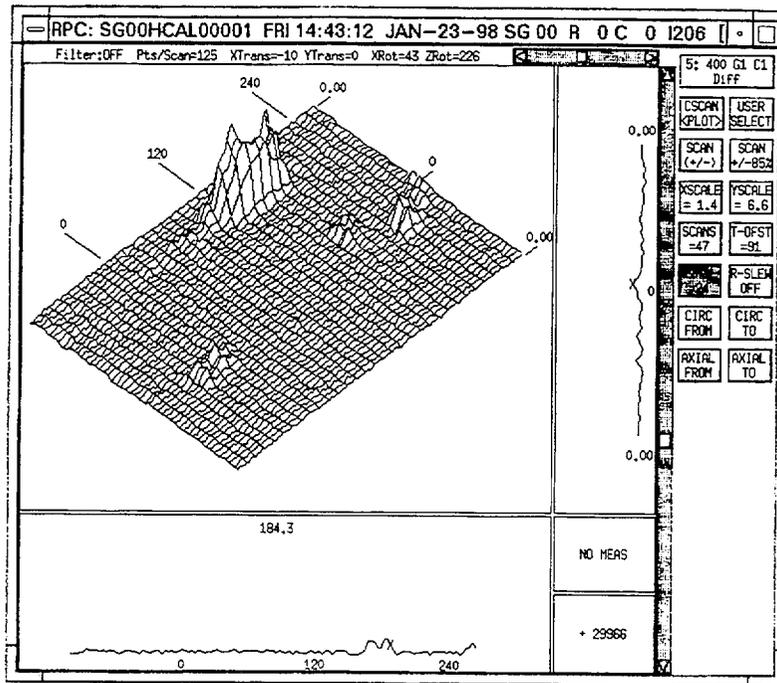
Fig. 4.4. Eddy current test of laboratory-degraded circumferential ODSCC in 22.2-mm (7/8-in.)-diameter Alloy 600 (heat no. NX8527) tube specimen SGL-063.
