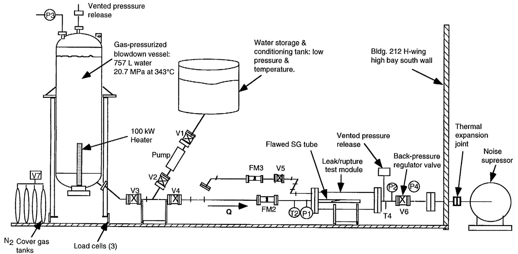
Fig. 4.12. Schematic diagram of Pressure and Leak-Rate Test Facility.
