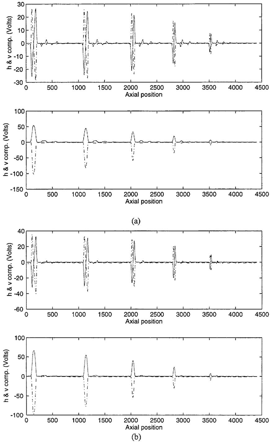
Fig. 3.8. Differential (top) and absolute channel (bottom) readings at (a)  $f = 100$  kHz, and (b)  $f = 400$  kHz with 18.3-mm (0.72-in.)-diameter magnetically biased bobbin coil on EDM standard with five sets of axial EDM notches ranging in depth from  $\approx 20\%$  to 100% TW. Nominal notch lengths in each set were 5.08 mm (0.2 in.), 10.16 mm (0.4 in.), 15.24 mm (0.6 in.), 20.32 mm (0.8 in.), and 25.4 mm (1.0 in.).
