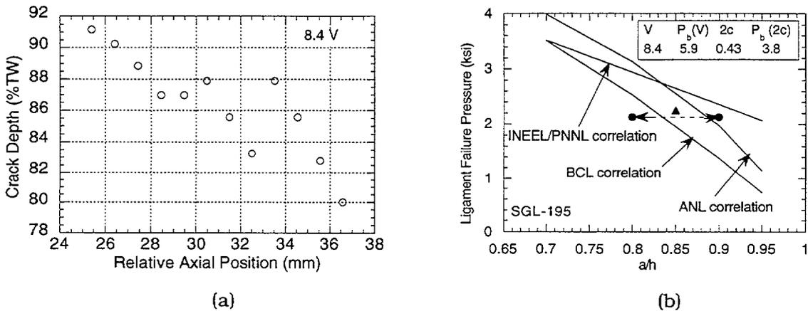
Fig. 4.39. (a) Measured crack depth profile in specimen SGL-195 by EC +Point and (b) predicted ligament failure pressure at room temperature for 10.9-mm (0.43-in.)-long rectangular crack as a function of crack depth. Circles represent range of crack depth measured by EC +Point method at pressure corresponding to first measurable leakage rate, and triangle represents average crack depth.
