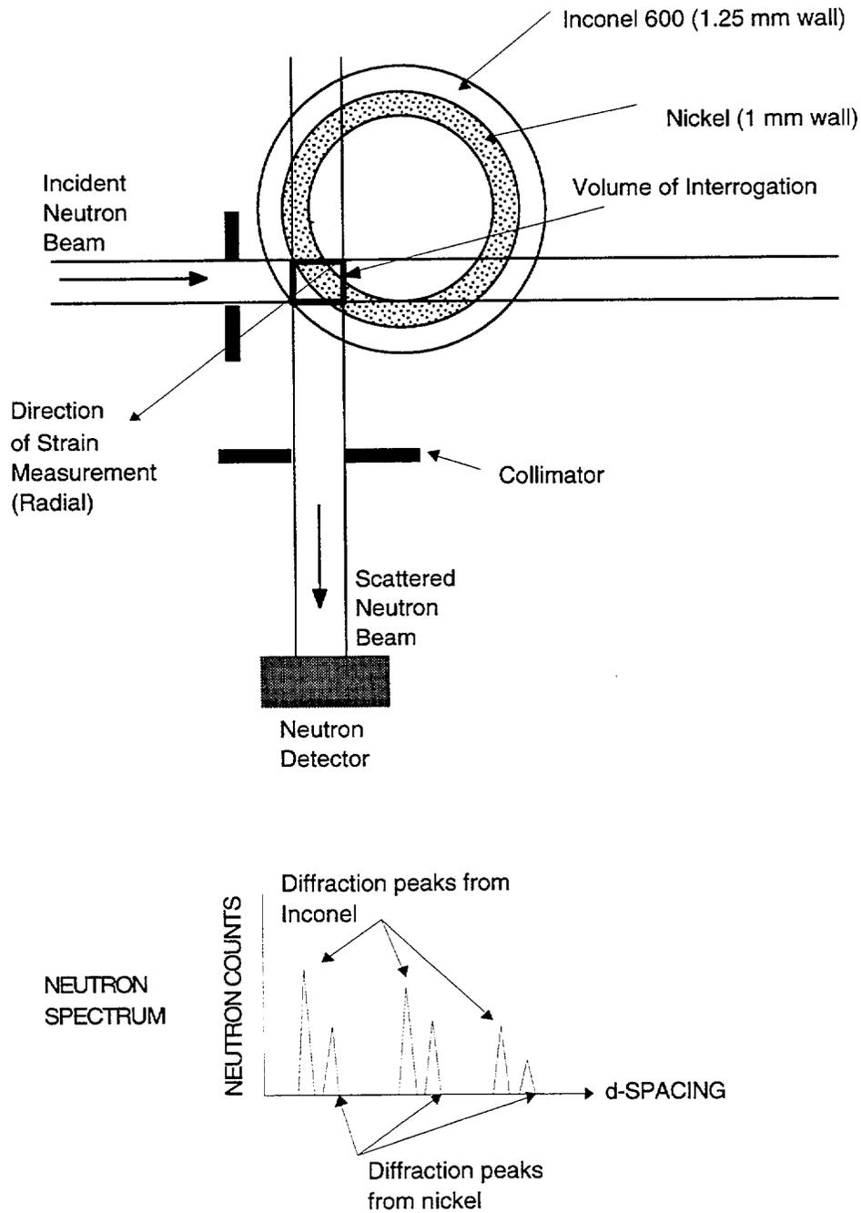
Fig. 5.5. Configuration of incident and scattered neutron beam from ANL IPNS used to simultaneously measure bulk radial strain in Alloy 600 parent tube and nickel sleeve. The diffraction peaks of nickel and Alloy 600 are easily separated, allowing strain relative to a reference to be determined.
