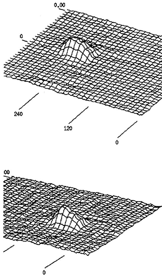
*Fig. 2.4. Comparison of 3-D presentations of eddy current signal from +Point Coil at 300 kHz for OD circumferential crack in Alloy 600 test section without (top) and with (bottom) a small amount of oxide coating. Change in eddy current signal from presence of coating, if any, are slight.*
