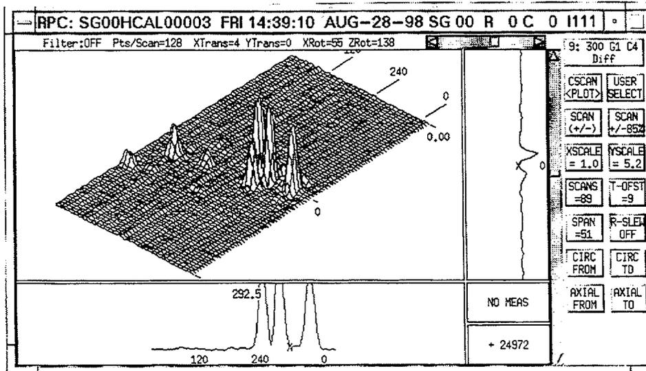
Fig. 4.7. Eddy current NDE of multiple axial ODSCC in Alloy 600 (heat no. NX8527) tube specimen SGL-289. Circumferential components of SCCs are also seen around tube.
