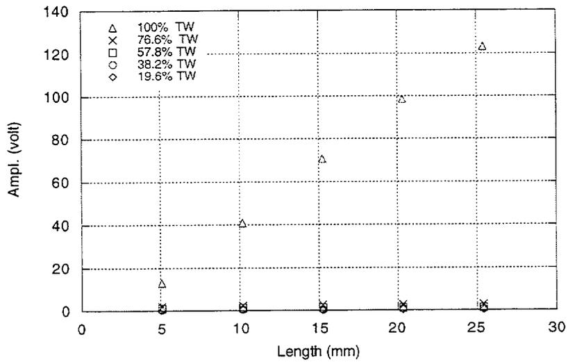
Fig. 3.11. Measured absolute peak signal amplitude (in volts) as a function of length by 18.3-mm (0.72-in.)-diameter magnetically biased bobbin coil on 25-notch EDM standard at (a)  $f = 100$  kHz, and (b)  $f = 400$  kHz.
