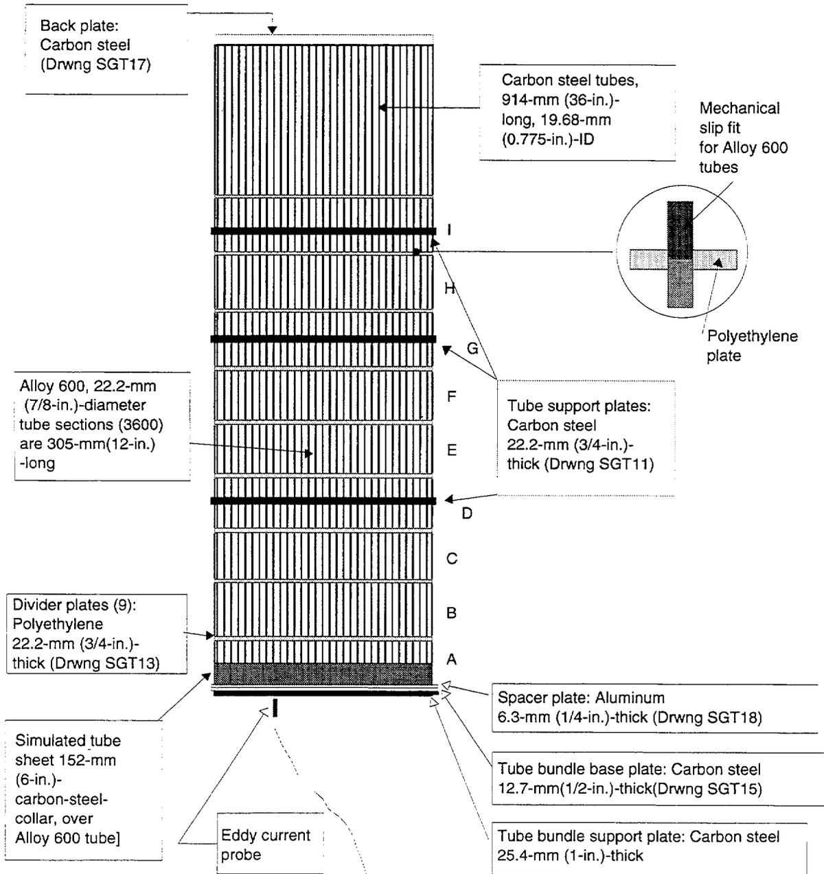
Fig. 2.2. Schematic diagram of mock-up tube bundle (total height 3.7 m [12 ft]).
