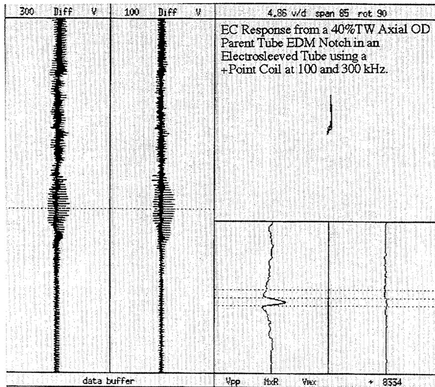
Fig. 5.4. Ultrasonic (top) and EC (bottom) signals from 0.5-mm (0.020-in.)-deep (40% TW) OD axial notch in parent metal of electrosleeved tube. Ultrasonic (70° shear) and EC flaw signals are detectable but UT signal is better.
