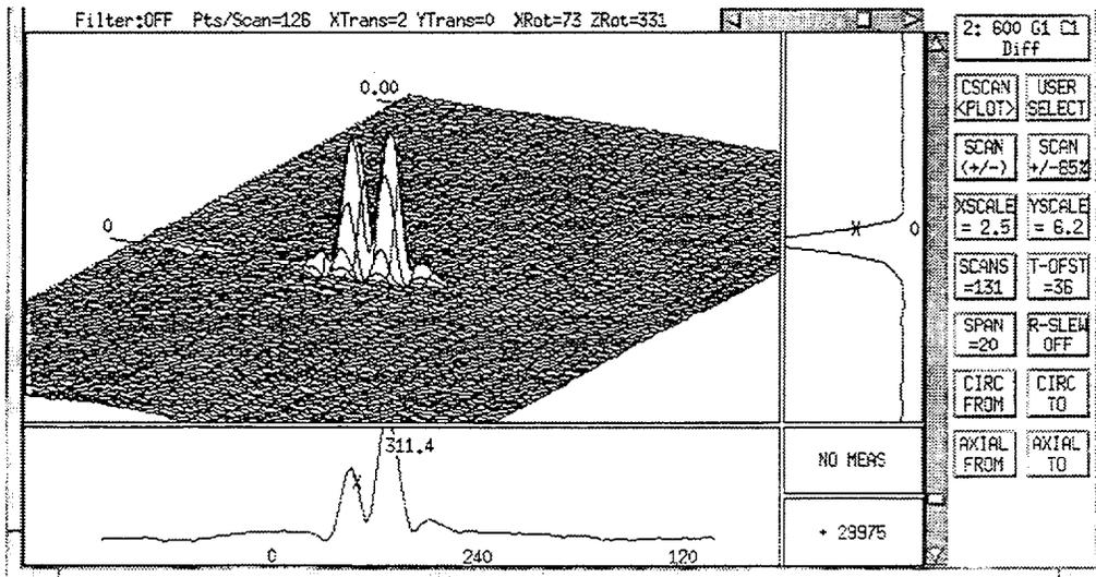
Fig. 4.2. Eddy current test of degraded throughwall circumferential ODSCC in 22.2-mm (7/8-in.)-diameter Alloy 600 (heat no. NX8527) tube specimen SGL-033.
