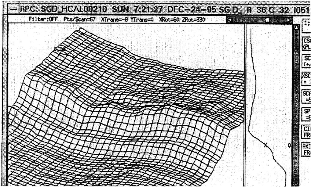
Fig. 2.16. 1995 c-scan plot of TTS of tube R36 C32 made with a 2.92-mm (0.115-in.)-diameter MRPC. No indication around roll transition was called at that time, and tube was not plugged. Tube axis is from lower left to upper right, with 360° of tube shown.
