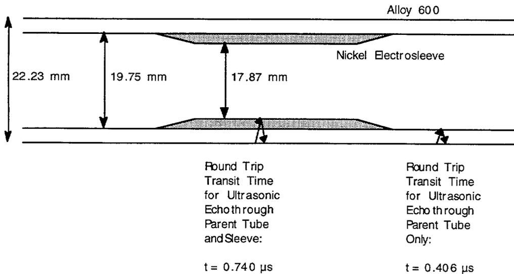
Longitudinal Velocity of Sound (Alloy 600) =  $(22.23 - 19.75) / (0.406) = 6110 \text{ m/s}$
