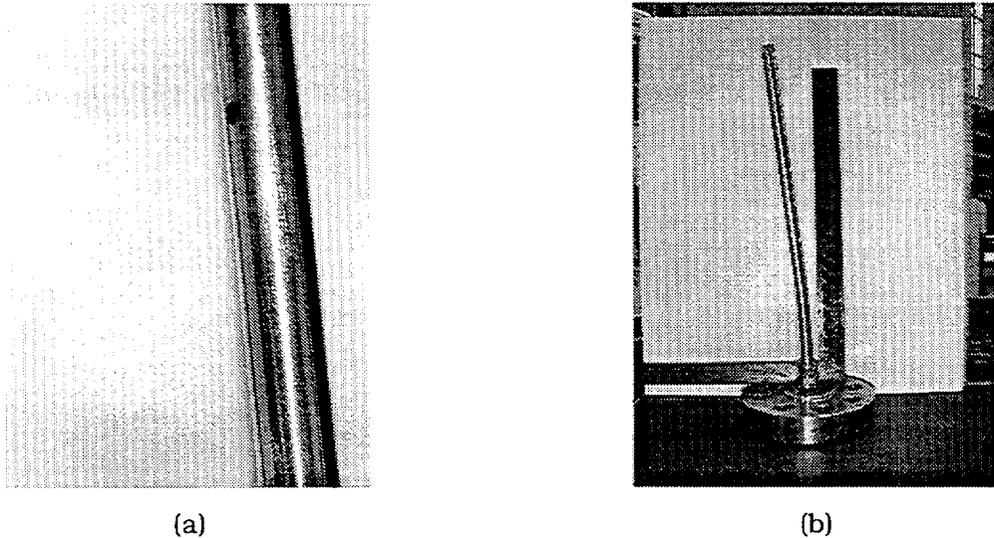
Fig. 4.16. Two views of tube T5EOTWX.250D containing 6.35-mm (1/4-in.)-diameter circular hole after testing, showing bending produced by thrust from water jet.
