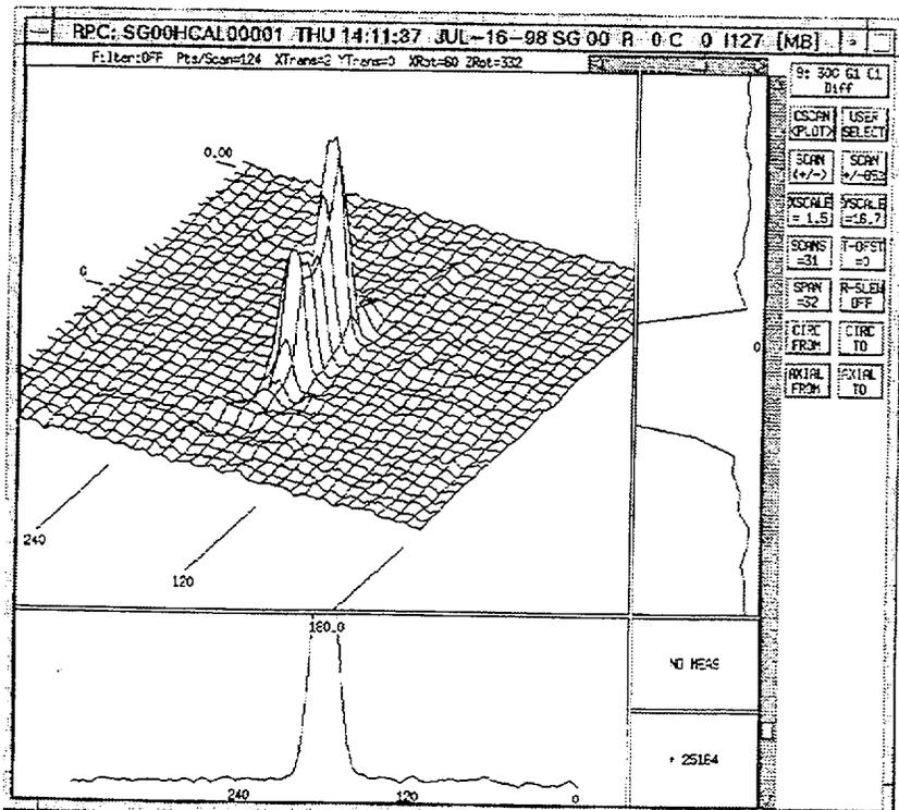
Fig. 4.6. Eddy current NDE of axial ODSCC in Alloy 600 (heat no. NX8527) tube specimen SGL-273. Two short throughwall cracks may be connected by a ligament.
