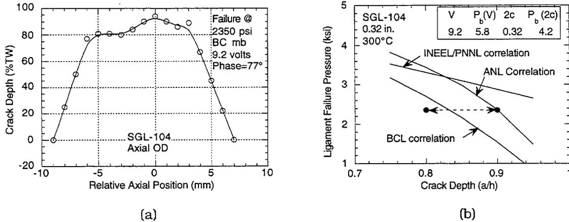
Fig. 4.40. (a) Measured crack depth profile in specimen SGL-104 by EC +Point and (b) predicted ligament failure pressure at 300°C for 8.1-mm (0.32-in.)-long rectangular crack as a function of crack depth. Circles represent range of crack depth measured by EC +Point method at pressure corresponding to first measurable leakage rate.
