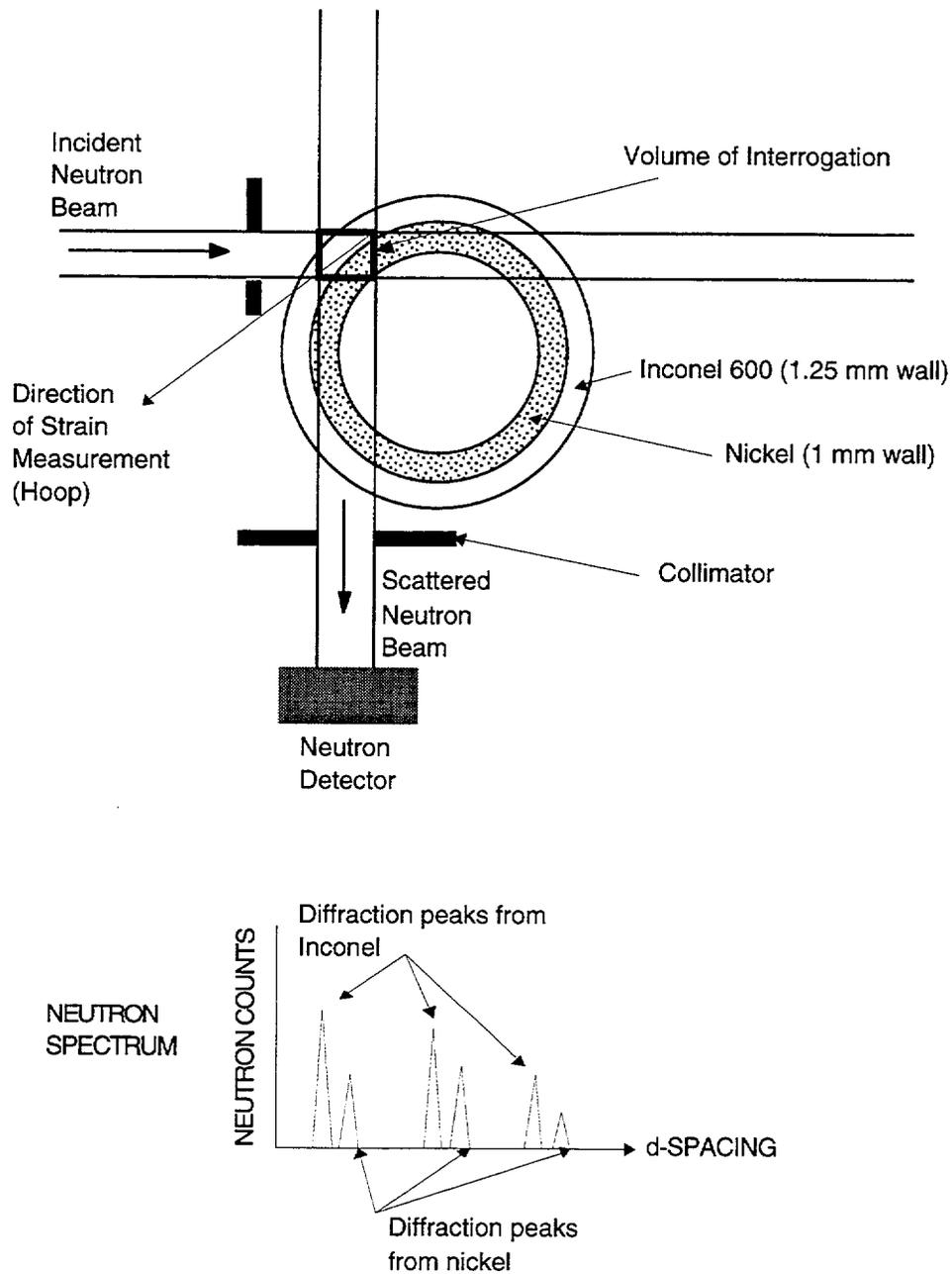
Fig. 5.6. Configuration of incident and scattered neutron beam from ANL IPNS used to simultaneously measure bulk hoop strain in parent tube and nickel sleeve. The diffraction peaks of nickel and Alloy 600 are easily separated, allowing strain relative to reference material to be determined.
