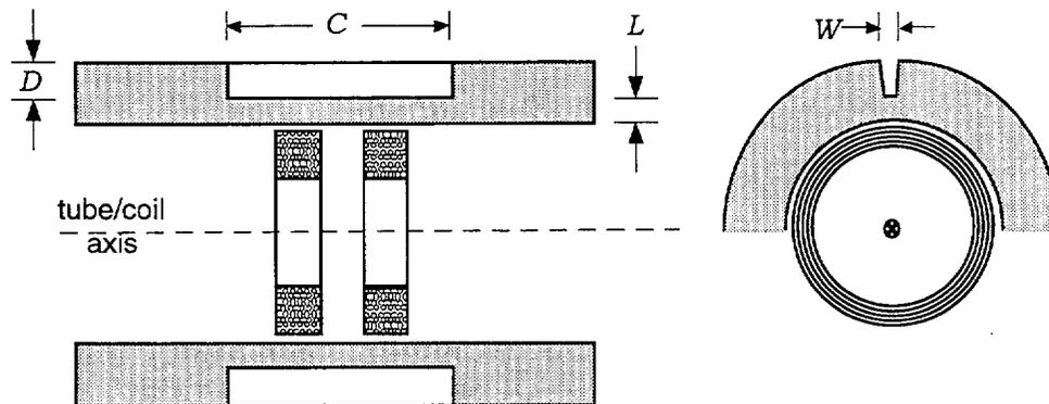
Fig. 3.1. Cross-sectional geometry of differential bobbin coil inside a tube with four symmetric OD discontinuities of length  $C$  and width  $W$ .
