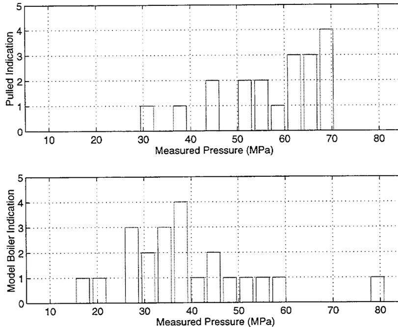
Fig. 3.13. Distribution of pulled tube (top) and model boiler (bottom) indications as a function of failure pressure used for multivariate analysis.
