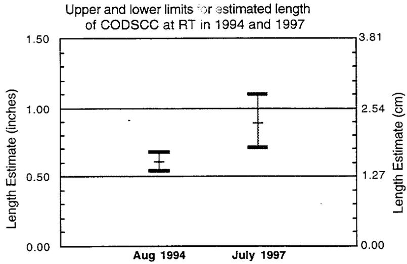
Fig. 2.19. Estimated length with range of uncertainty for circumferential outer diameter stress corrosion crack (CODSCC) at top of tube sheet in tube 39-46 of McGuire retired steam generator before (August 1994) and after (July 1997) plugging.
