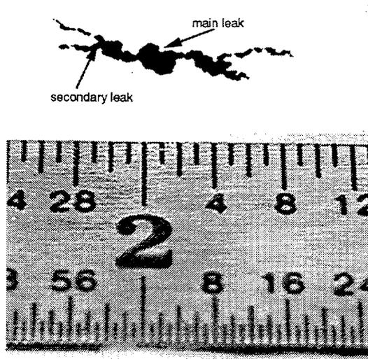
Fig. 4.20. Pretest image of tube SGL-177 with flaw highlighted by dye penetrant and digital image processing; two regions of throughwall penetration are indicated by bubble testing.
