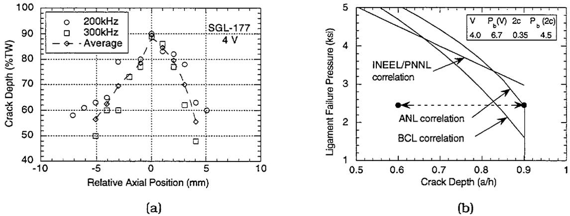
Fig. 4.38. (a) Measured crack depth profile in specimen SGL-177 by EC +Point and (b) predicted ligament failure pressure at room temperature for 8.9-mm (0.35-in.)-long rectangular crack as a function of crack depth. Circles represent range of crack depth measured by EC +Point method at pressure corresponding to first measurable leakage rate.
