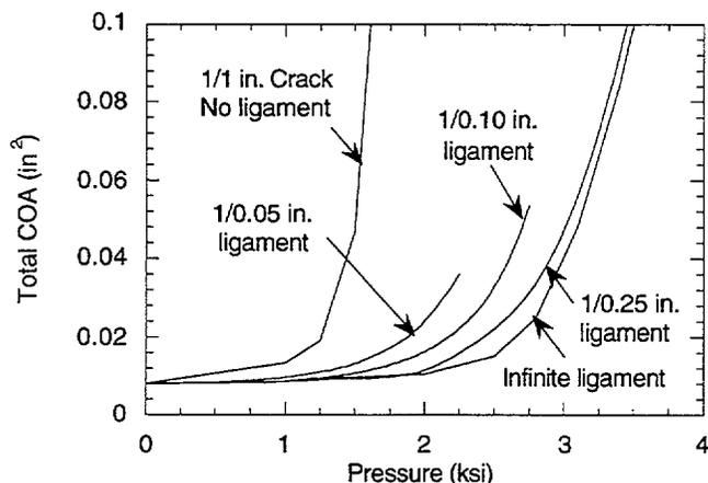
Fig. 4.34. Calculated variation of flaw opening area with pressure for single flaw 25.4-mm (1-in.) long and two flaws each 12.7-mm (0.5-in.) long separated by ligaments of various widths. Each flaw had an initial width of 0.20 mm (0.008 in.).
