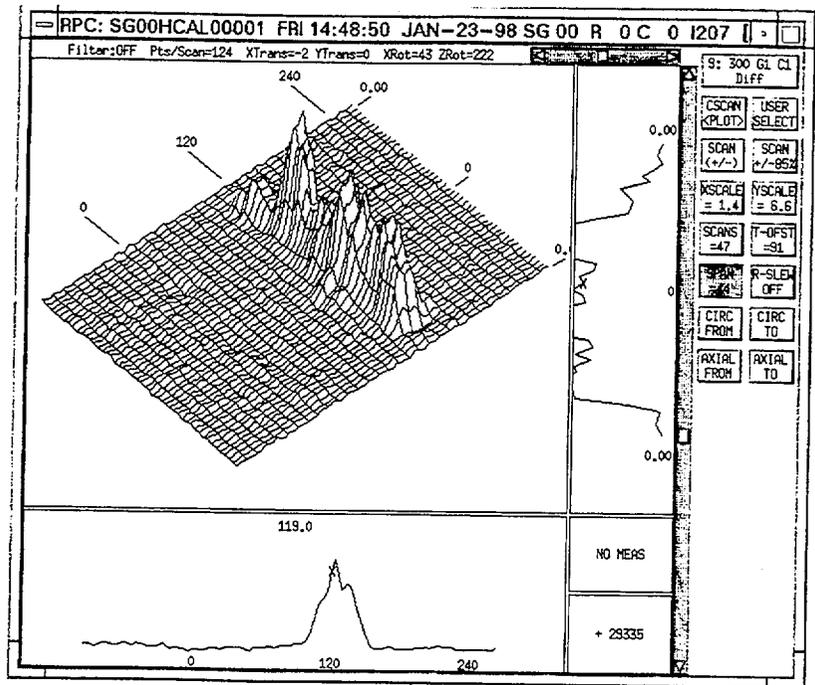
Fig. 4.5. Eddy current test of laboratory-degraded throughwall axial ODSCC in 22.2-mm (7/8-in.)-diameter Alloy 600 (heat no. NX8527) tube specimen SGL-065.
