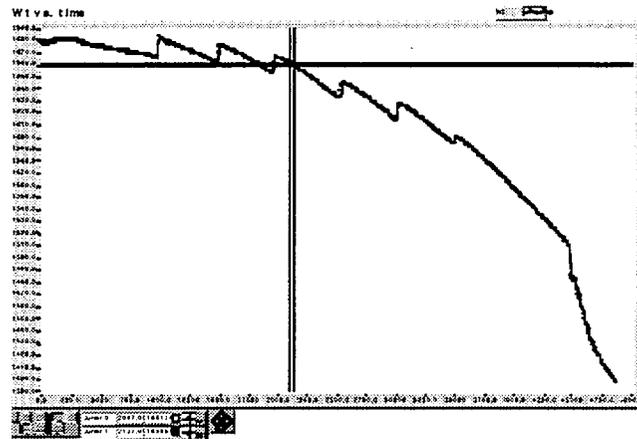
Fig. 4.15. Blowdown vessel weight vs. time during test of tube with 0.794-mm (1/32-in.)-diameter hole (T6EOTWX.031D).
