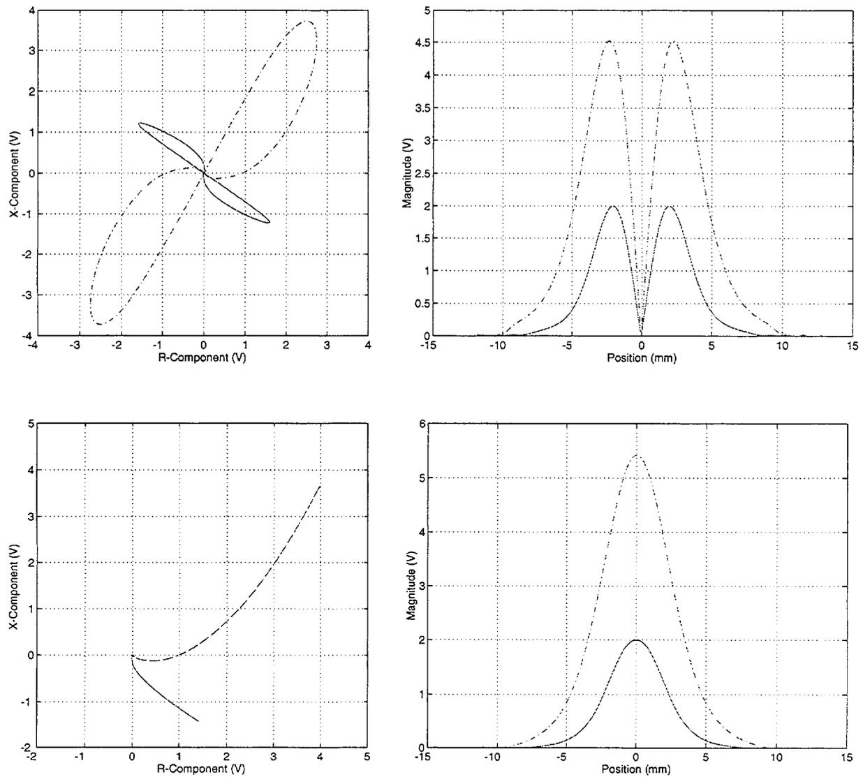
Fig. 3.3. Differential (top) and absolute (bottom) bobbin probe impedance trajectory (left) and signal amplitude (right), in volts, at  $f = 400$  kHz (solid line), and  $f = 100$  kHz (dashed line) for four 20% ASME standard OD FBHs placed  $90^\circ$  apart around tube circumference.
