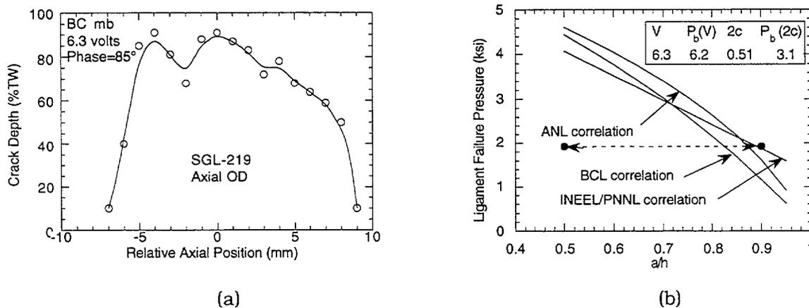
Fig. 4.41. (a) Measured crack depth profile in specimen SGL-219 by EC +Point and (b) predicted ligament failure pressure at 300°C for 13.0-mm (0.51-in.)-long rectangular crack as a function of crack depth. Circles represent range of crack depth measured by EC +Point method at pressure corresponding to first measurable leakage rate.
