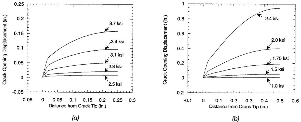
Fig. 4.31. Calculated total crack opening displacement as a function of internal pressure for single (a) 12.7-mm (0.5-in.)-long and (b) 25.4-mm (1.0-in.)-long TW cracks.
