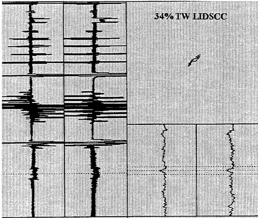
Fig. 2.7a. Lissajous figure for +Point™ coil at 200 kHz for crack estimated from destructive analysis to be 34% TW.
