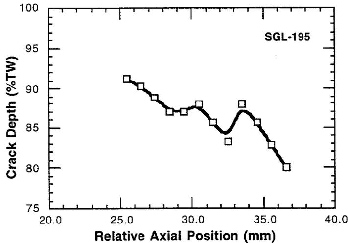
Fig. 2.9. Axial OD crack depth as a function of position for test section SGL-195 using phase analysis at 300 kHz with a +Point coil and EDM notches for calibration. Only eddy current signals with good S/N ratios were analyzed. Signals from ends of crack had much lower amplitude than signals near the middle. Solid line represents smooth curve fit to measurements.
