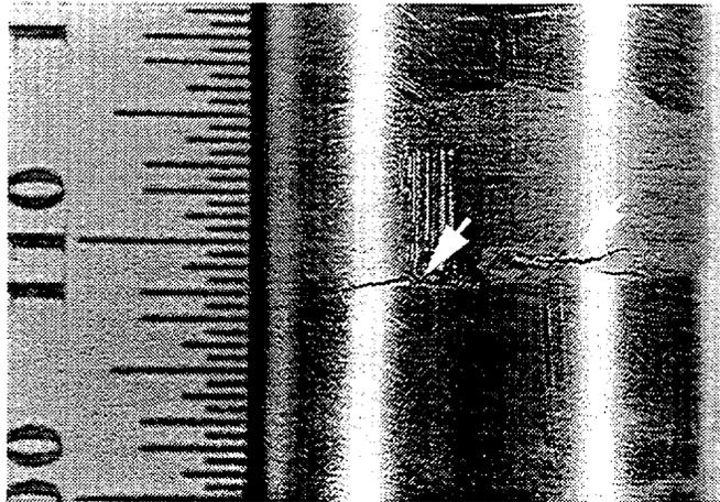
Fig. 4.1. Laboratory-degraded throughwall circumferential ODSCC in 22.2-mm (7/8-in.)-diameter Alloy 600 (heat no. NX8527) tube specimen SGL-033.
