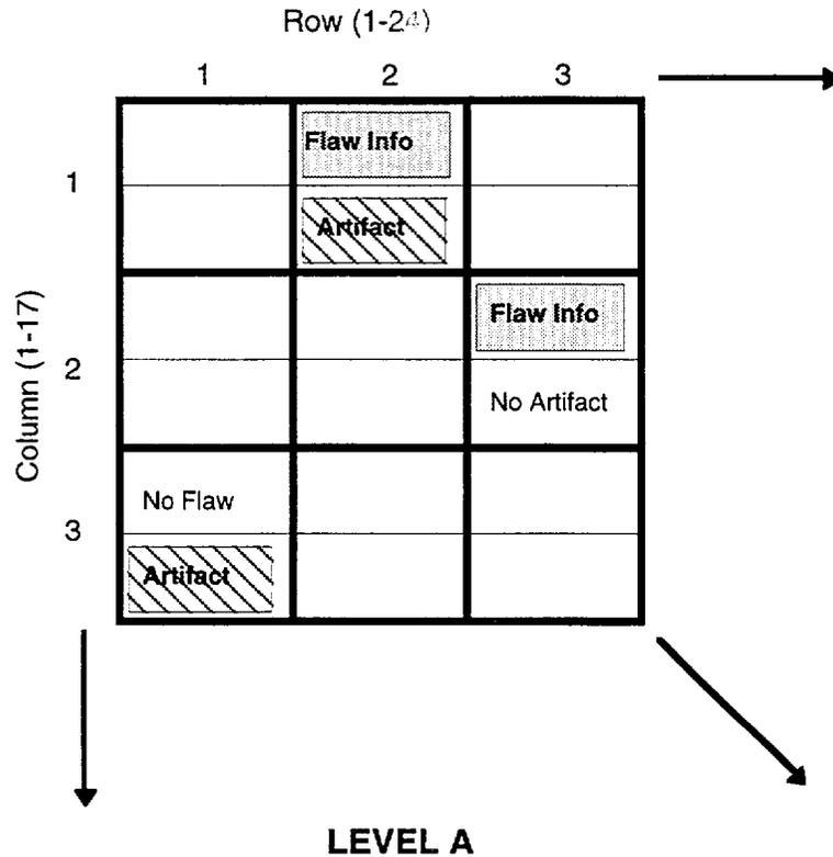
Fig. 2.5. Schematic representation of section of flaw map at specified level "A" (one of nine levels, A through I).
