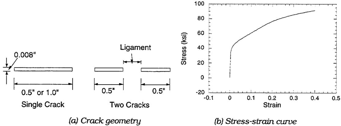
Fig. 4.30. (a) Crack geometry and (b) stress-strain curve assumed for analysis.
