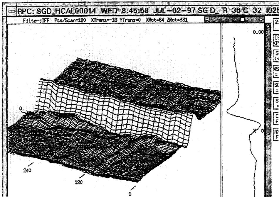
Fig. 2.18. 1997 c-scan image of same region shown in Figs. 2.16 and 2.17 made with +Point™ coil; call again is MAI. Value of additional data from +Point™ coil can be seen here, where multiple axial indications in and around roll transition can be seen more clearly than in Fig. 2.17.
