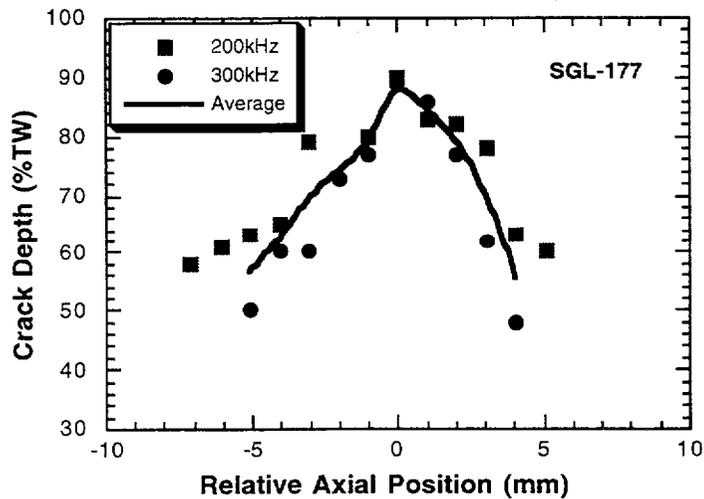
Fig. 2.10. Axial OD crack depth as a function of position for test section SGL-177 using phase analysis at 200 and 300 kHz with a +Point coil and EDM notches for calibration. Only eddy current signals with good S/N ratios were analyzed. Signals from ends of crack had much lower amplitude than signals near the middle, and thus depth estimates were not made beyond the region shown in figure.
